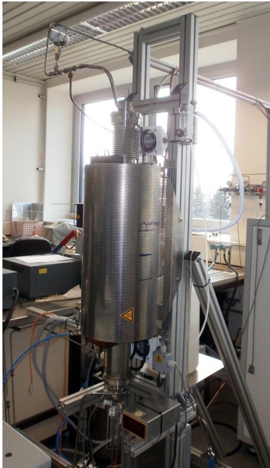
Hydrogenation facility LORA furnace
