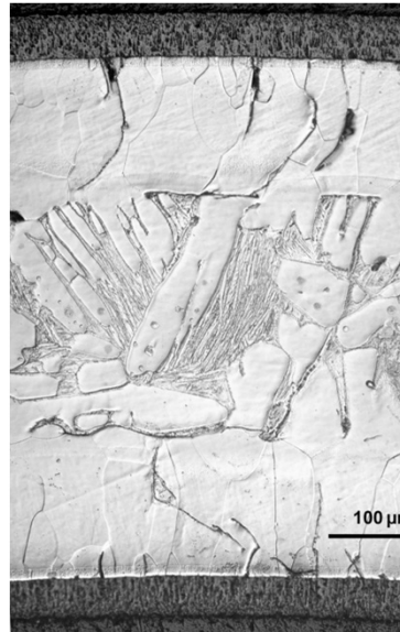
Annealing 900 s: ZrO 2 52 µm, dissolved 12 µm, alpha-Zr(O) 165 µm
