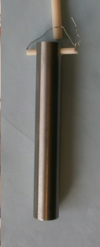
Cooled specimen after pre-oxidation and annealing
