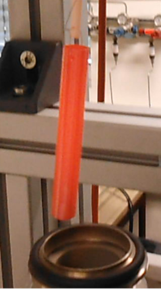
Specimen withdrawal in air after test Estimated cooling rate was 5 K/s
