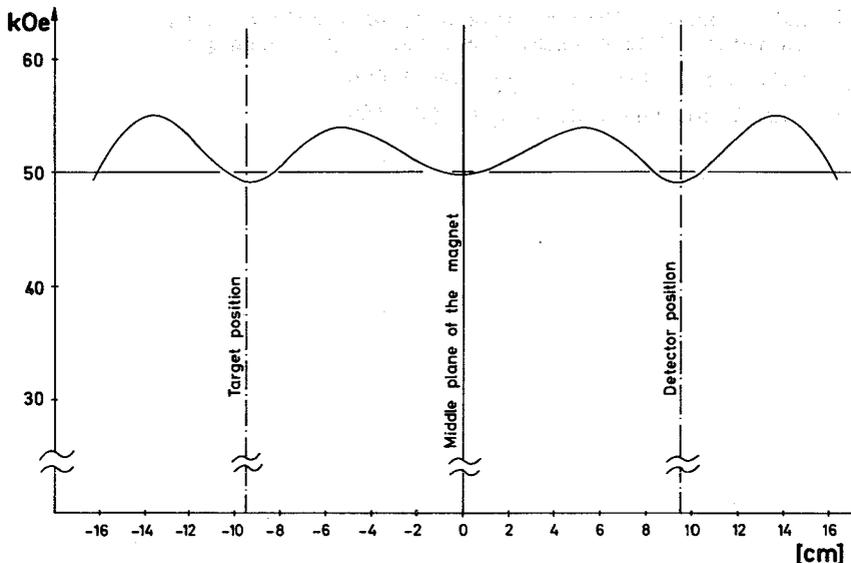
FIG. 5. Magnetic field strength on the spectrometer axis.
