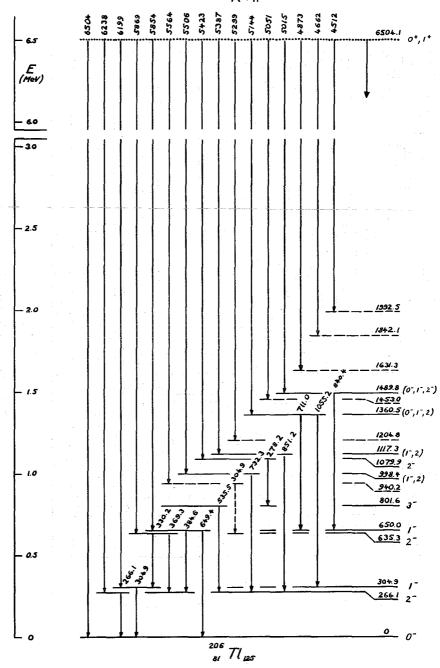
FIG.4. Transition diagram of <sup>206</sup>T1.
