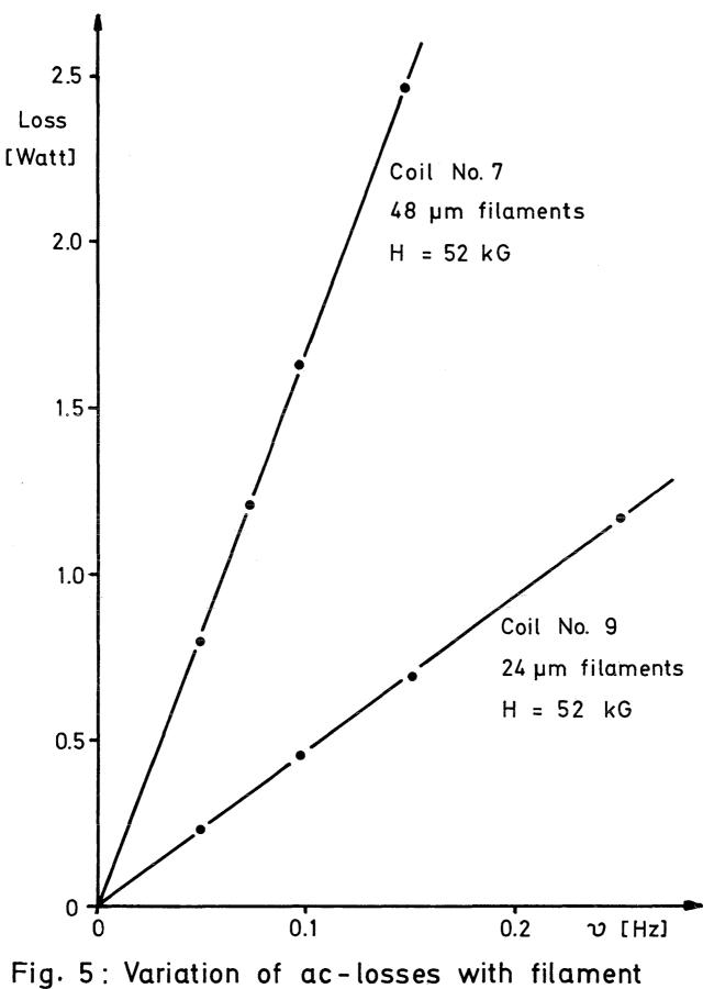
diameter for twisted Cu/CuNi composites
