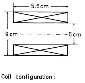
2990 turns of 0.05 cm diam. composite (61x42µm filaments) Twist: 1 turn/inch I<sub>quench</sub> ≈ 101 A ≜ H<sub>quench</sub> ≈ 40 kG
