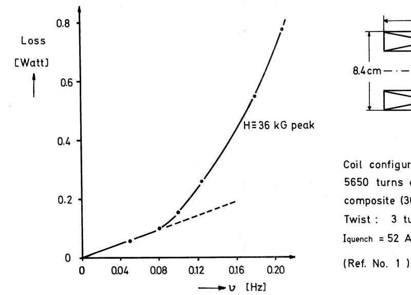
Coil configuration: 5650 turns of 0.05 cm diam. composite (361 x 13 µm filaments) Twist : 3 turns/inch Iquench = 52 A = Hquench = 50 kG
