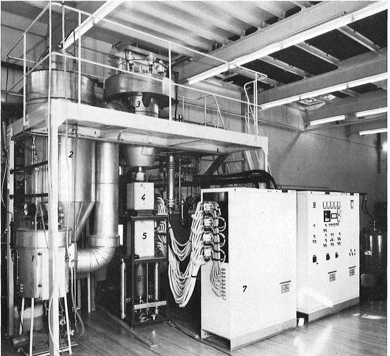
Fig. 2 General view of the inactive pilot-scale facility for vitrification of fission product solutions
