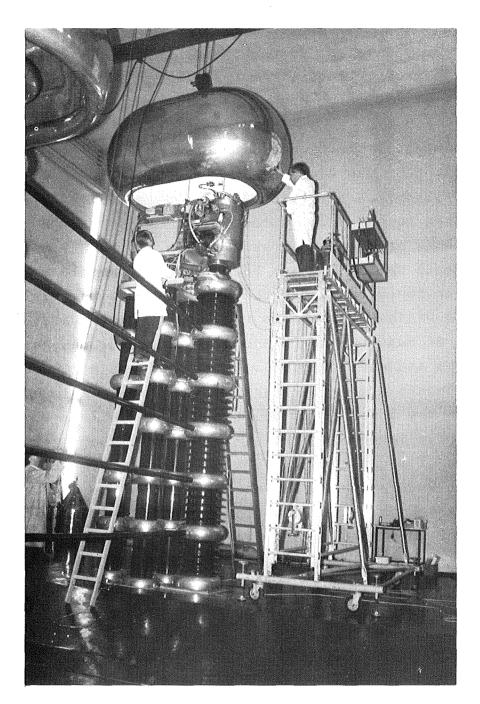
Fig. 5: Experimental set-up for the neutralization experiments at Grafschaft. Underneath the raised high voltage dome of the accelerator the cylindrical cryostat of the cluster ion beam source can be recognized.
