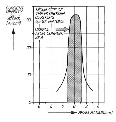
Fig. 3: Intensity profile of a hydrogen cluster beam with an average cluster size of approximately  $5.5 \times 10^4$  H-atoms probably required for ionization.
