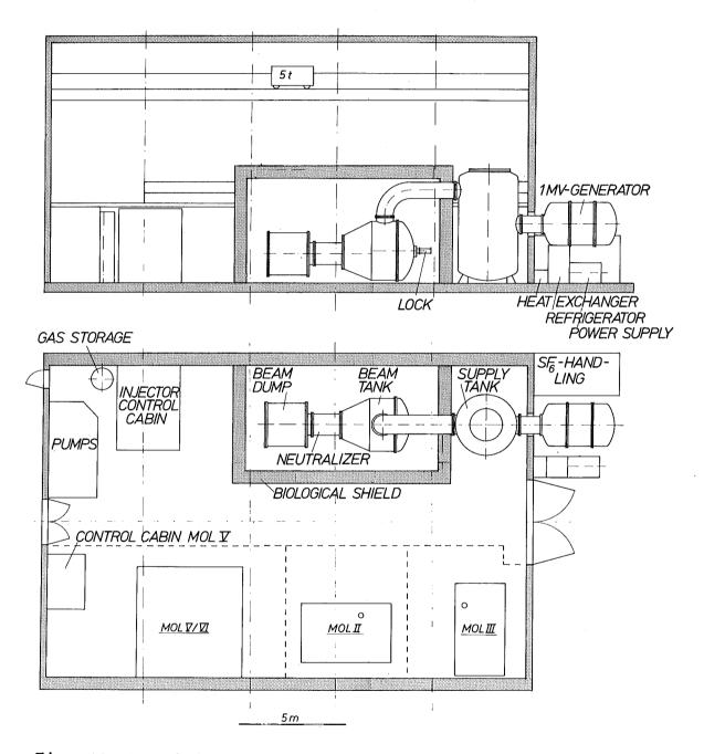
Fig. 10: Preliminary arrangement of the injector in the experimental hall of IKVT.
