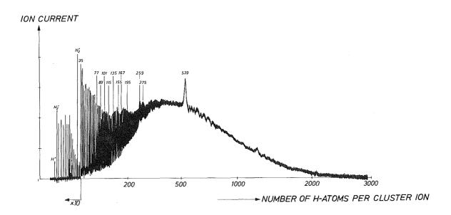
Fig. 1: Cluster ion spectrum generated by electron impact ionization of clusters of approximately 10<sup>4</sup> Hatoms. The cluster ions contain on the average 300 H-atoms per charge.
