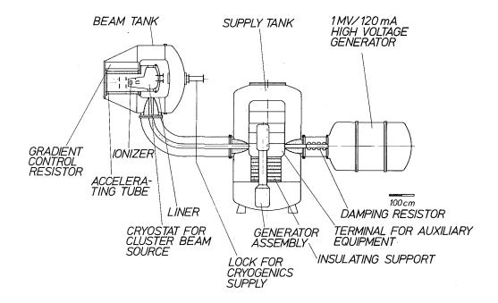
Fig. 6: Schematic representation of the injector structure with the three units of beam tank, supply tank, and high voltage generator.
