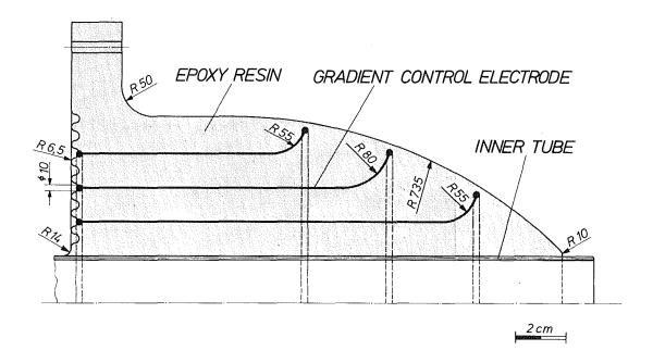
Fig. 9: Potential controlled bushing for a voltage of 1 MV. The tubular inner conductor is surrounded by an insulating body made of epoxy resin whose cast control electrodes determine the potential conditions.
