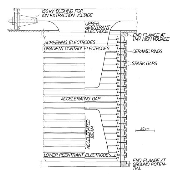
Fig. 7: 1 MV-accelerator tube for the injector.
