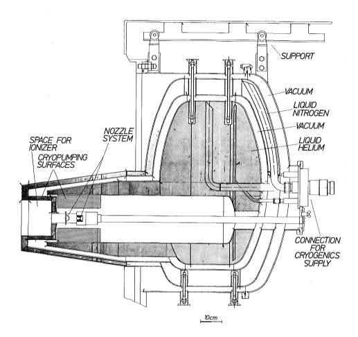
Fig. 8: Draft design of the cryostat of the cluster beam source of the injector.
