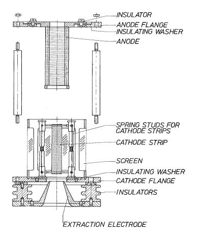
Fig. 2: The electron impact ionizer shown on this diagram was used to produce the cluster ions with the mass spectrum shown in Fig. 1.
