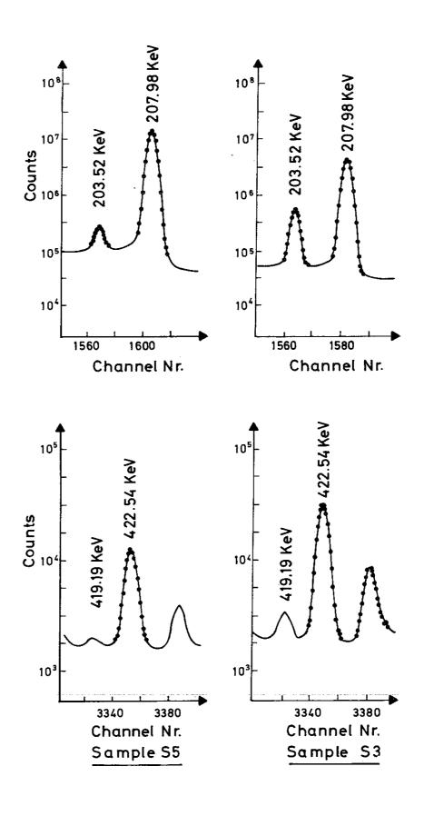
Fig. Al Gamma Spectra of Plutonium Samples Taken Using a 18 cc Ge(Li)-Detector - 200 keV and 420 keV Regions.
