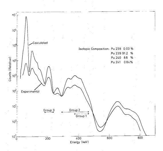
Fig. 1 Typical Gamma Spectrum of a Plutonium Sample
