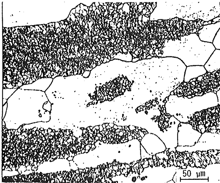
FIG. 2-Light micrograph illustrating mixed recrystallized (light) and unrecrystallized (dark) structure of commercially processed 7050-T6X1 plate. Etched in 25% HNO 3 for 3 min. at 70°C.
