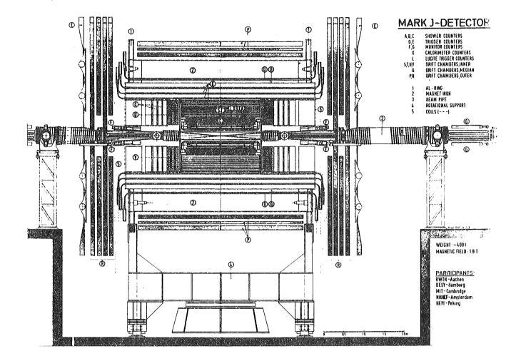
Fig. 4 The MARK J detector (Aachen-DESY-LAPP-MIT-NIKHEF-Peking collaboration).
