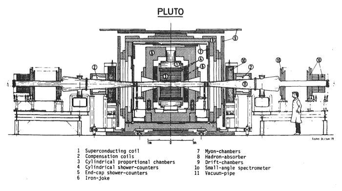
Fig. 3 The PLUTO detector in its PETRA configuration (Aachen-Bergen-DESY-Hamburg-Maryland-Siegen-Wuppertal Collaboration)
