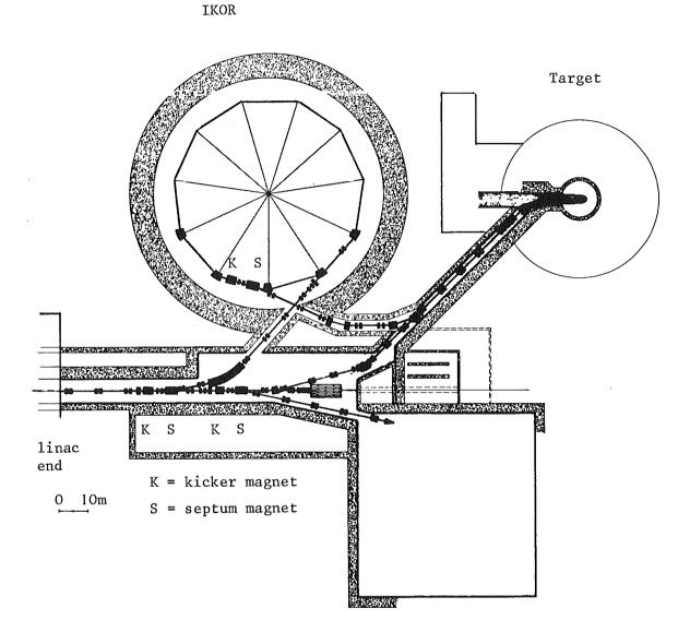
Fig. 1 SNQ linac and IKOR beam transport, general layout
