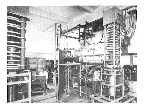
Fig. 5: The study klystron assembled in the test facility
