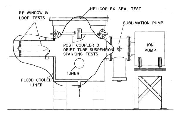
has 11 ports around the circumference to accommodate: drive line, vacuum port, drift tube, post coupler, tuner, field probe, viewing ports, port to test helicoflex and other seals and spares. The resonant frequency is calculated to be 276.5 MHz empty and 273 MHz with a drift tube installed. The load is designed to operate at 400 kW to test rf lines at high power.
