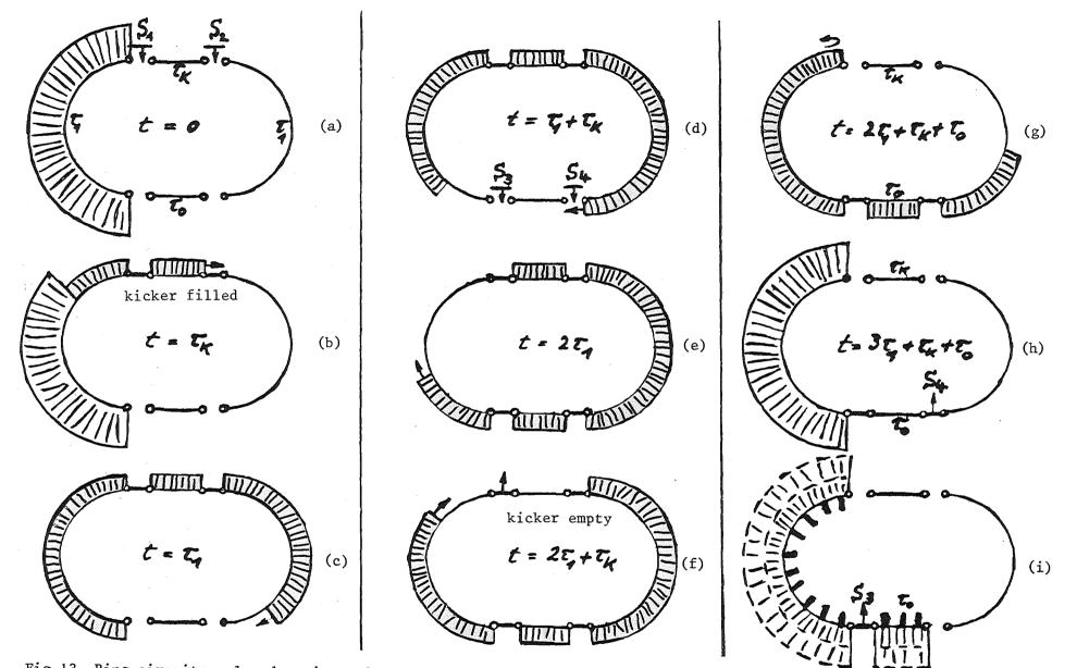
Fig.13 Ring circuit: pulse duration =  $2\tau_1 - \tau_k$  for full excitation of the kicker field. After refilling, smoothening, separation (S3) and discharge of the auxiliary line section ( $\tau_0$ ), the initial condition (t=0) is re-established.
