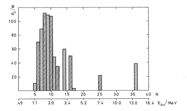
Fig. 3 Beam power load  $P_D$  per drift tube at 5 % duty cycle resulting from particle losses due to incomplete bunching as a function of the drift tube number N and the proton energy  $E_{kin}$  (multiparticle simulation with 2000 macro particles; large statistical errors above 2.5 MeV)
