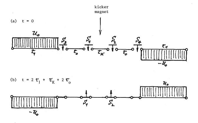
Fig.12 Modified twin wave system: the addition of empty line sections ( $\tau_0$ ) permits an opening of the gas discharge switches S1 and S2 at zero voltage and zero current after the charge exchange between the 2 PFN's has been completed (or shortly before that).
