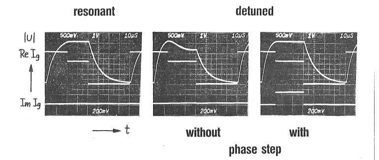
Fig. 2 Dead beat filling of a detuned resonator
