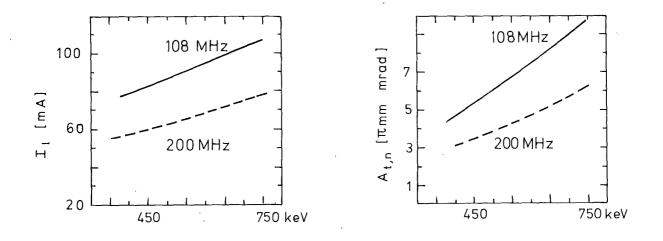
Fig. 2 Longitudinally accepted beam current  $I_1$  and normalized transverse acceptance  $A_{tn}$  as a function of the injection energy into the Alvarez accelerator  $E_{kin}$  (analytical estimate for 3  $\pi$  mm mrad normalized emittance; parameter is the Alvarez accelerator frequency; higher beam currents can be accelerated in practice)
