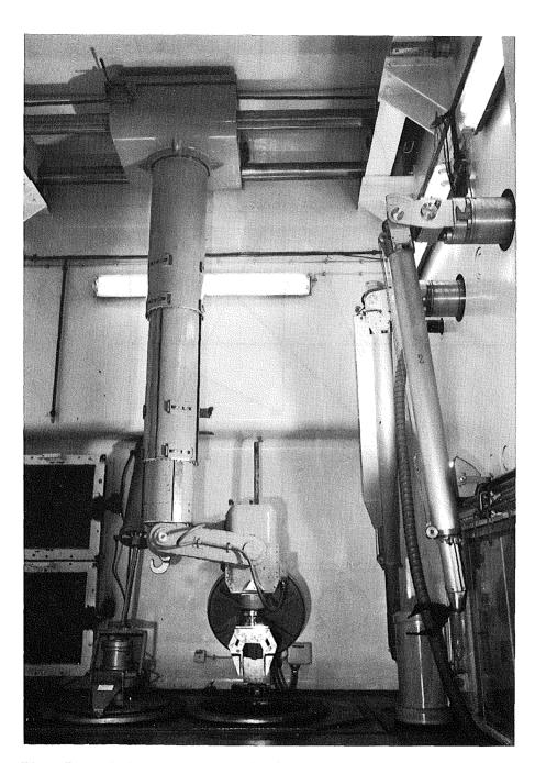
Fig. 5 SM5-C Power Manipulator, Handling Capacity 300 kg, Lifting Capacity on the Hook 2000 kg, 8 Motions
