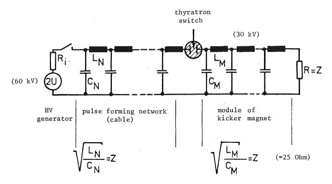
Fig.7 Generation of kicker pulses for beam ejection, schematically. The indicated values are typical for one of the 8 IKOR kicker modules.
