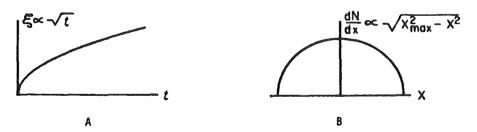
Fig. 5. Beam-bumping program (A) produces beam distribution (B).
