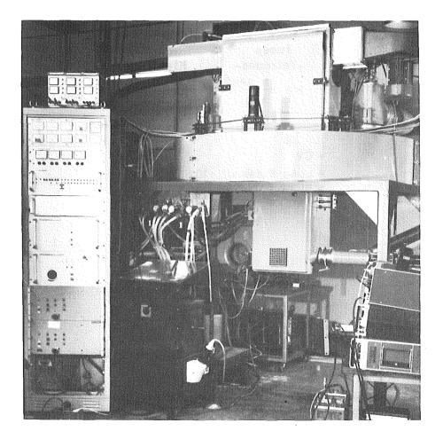
Fig. 3: Tetrode amplifier prototype
