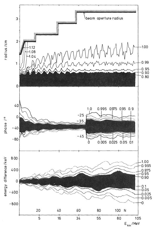
Fig. 4 Transverse (top) and longitudinal (below) density distribution inside the bunch along the Alvarez accelerator. Parameter is that particle fraction having smaller radius, phase or energy than given by a considered curve. In the top diagram the bunching losses are included. N = drift tube number,  $E_{kin}$  = proton energy (multiparticle simulation, hence the curves labelled with 1.0 or 0.0 are subject to large statistical errors).
