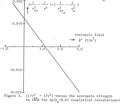
From this figure we see that a sextupole strength B"=1.16 T/m<sup>2</sup> is required in order to keep  $(1/\gamma_{tr}^2 - 1/\gamma^2)$ =constant. This value is in good agreement with the value obtained from the AGS program by Reich(see ref.2):  $B'' = 1.2 T/m^2$ .
