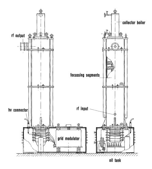
Fig. 7: 3.5 MW klystron amplifier unit
