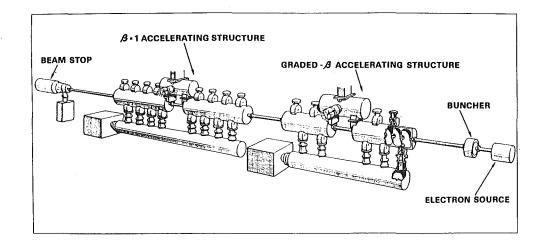
Diagram showing the principal components of the Electron Test Accelerator.
