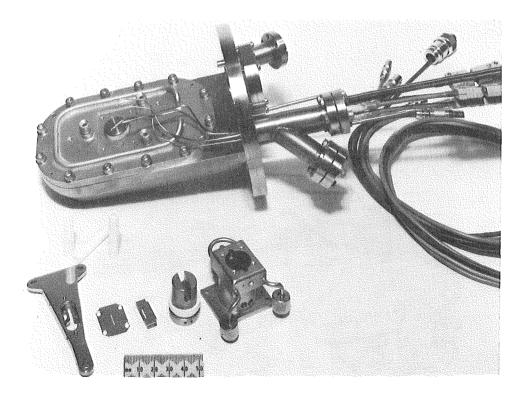
Figure 2. Discharge Chamber and Extractor Assembly
