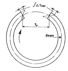
Fig. 1 In the absence of longitudinal RF or space-charge fields, the azimuthal beam void of duration  $T_v$  (= 100 ns in IKOR) shrinks by 2 x  $\int \Delta T_{rev}$  due to the drift-ing caused by the beam momentum spread. (Not to scale)
