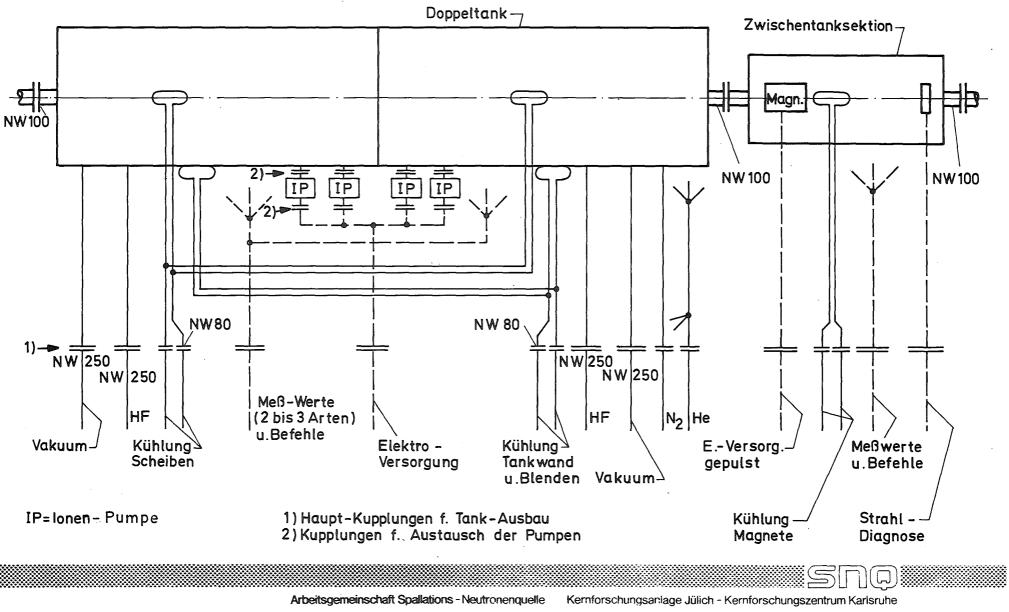
Fig. 17. Disk-and-washer accelerator, coupling diagram
