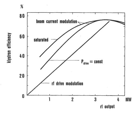
Fig. 6: Klystron efficiency depending on the modulation method
