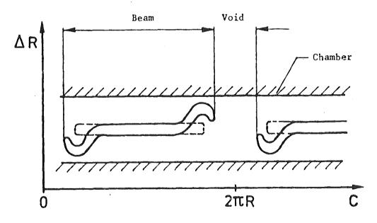
Fig. 3 Radial and longitudinal distortions at the beam edges near the void (full lines) at  $n \gtrsim 0$  due to longitudinal space-charge fields resulting from longitudinal density gradients /1/. (Not to scale)
