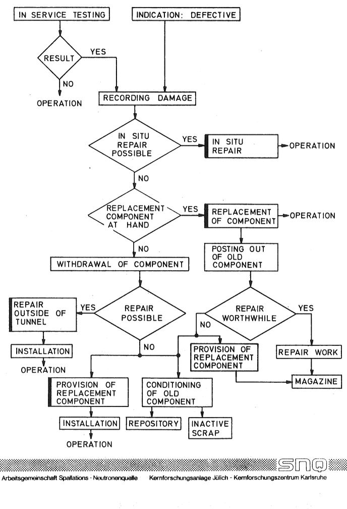
Fig. 15. Flow diagram and alternatives of repair.
