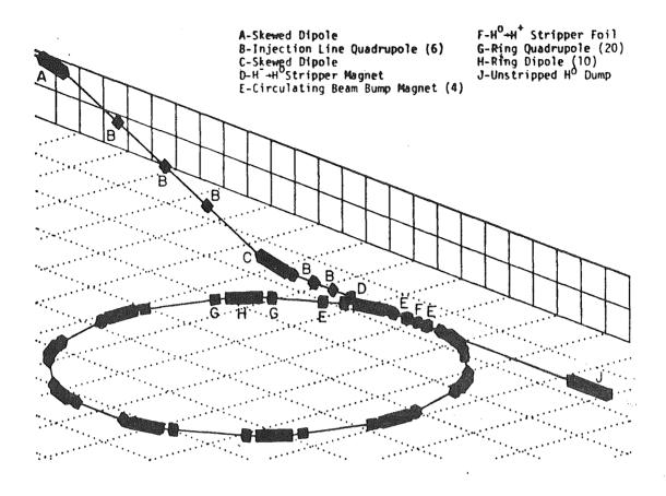
Fig. 1. PSR injection system schematic.
