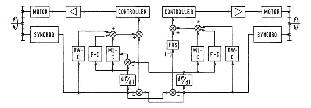
Fig. 3. BILATERAL SERVO SYSTEM WITH TWO-CIRCUIT POSITION CONTROL WITH COMPENSATIONS, FOR ELECTRIC MASTER-SLAVE MANIPULATOR
