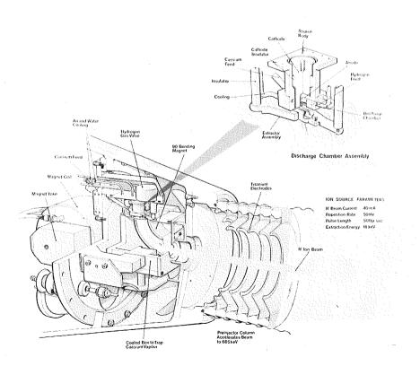
Figure 4. Ion Source and Accelerator Column
