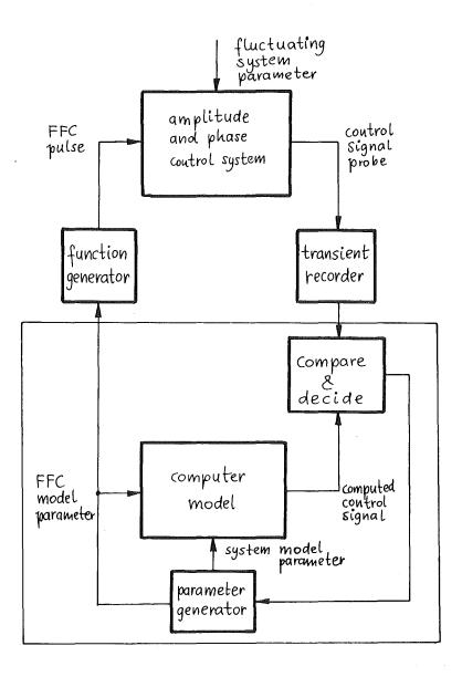
Fig. 6 Basic block diagram of adaptive feedforward parameter adjustment
