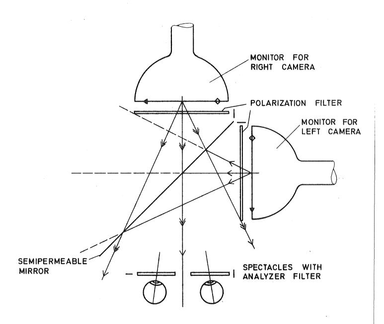
Fig. 6. Viewing equipment for stereo television
