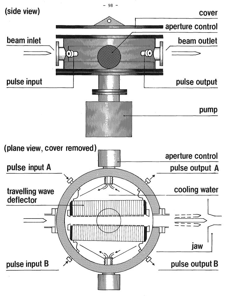
Fig.15 Rf kicker assembly in the low-energy beam transport of the SNQ linac. (450 keV,  $\beta \approx 3$  %, effective length = 0.4 m, minimum required UL = 360 Vm for  $\epsilon$  = 3  $\pi$  /uradm).
