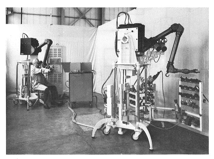
Fig. 4 EMSM 1 Electric Master-Slave Manipulator, Handling Capacity 25 kg, 9 Motions
