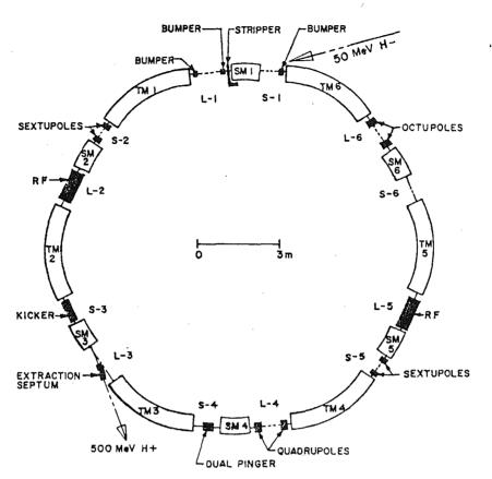
Fig. 4. RCS Component Arrangement
