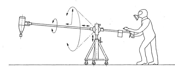
Fig. 11. Supported remotely handled tool (e.g. an impact wrench)
