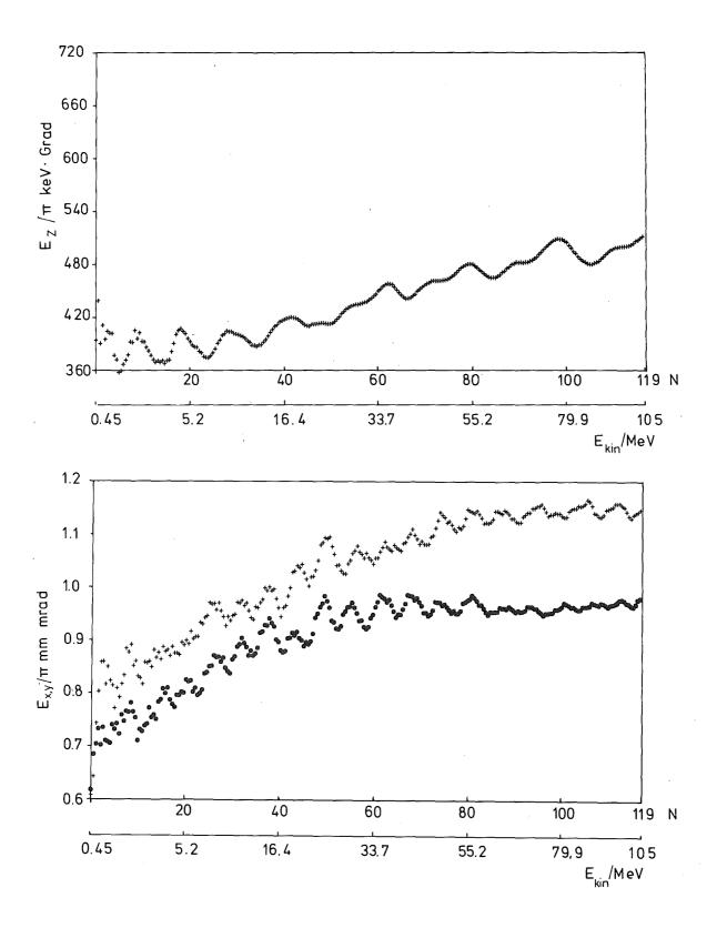
Fig. 5 Normalized rms-emittance along the Alvarez accelerator (at the top the longitudinal  $E_z$ , at the bottom the transverse ones  $E_x$ ,  $E_y$ ; N = drift tube number,  $E_{kin}$  = proton energy)
