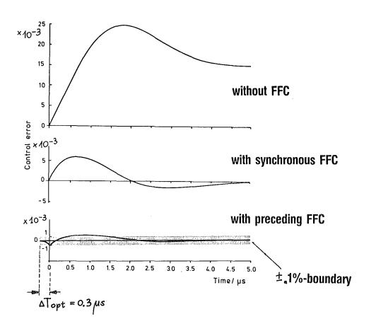
Fig. 5 Control error due to transient beam loading without, with synchronous and with preceeding feedforward control (FFC)
