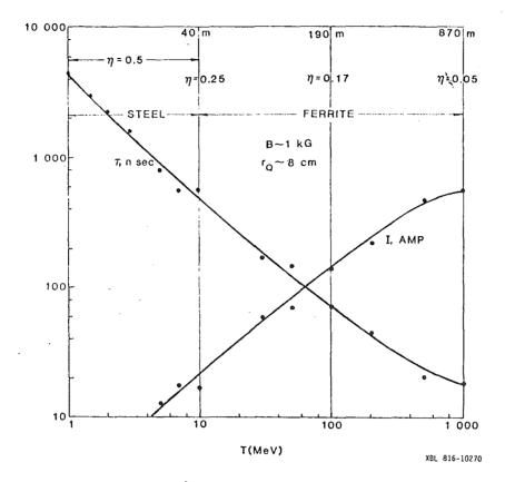
Figure 2: An example of how the current and pulse duration should vary to minimize the overall cost (on the conservative (C) basis). The fraction of space occupied by magnets, n, is indicated and can be seen to be small over most of the length. With the F cost-basis the length is halved.
