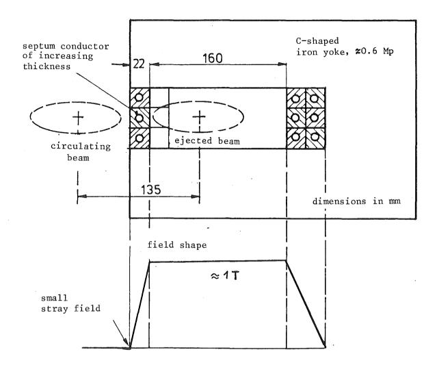
Fig.3 IKOR septum magnet, schematically. length 0.8 m current 67 kA power  $\approx 160$  kW
