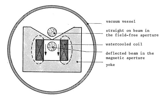
Fig. 4 Lambertson-Septum (iron septum, schematically, kick vertical, main deflection horizontal)
