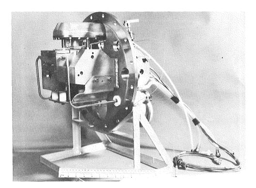
Figure 1. Ion Source Assembly
