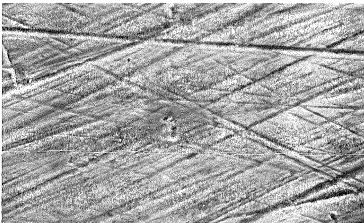
Fig. A 9 Typical surface appearance of as-received Stellite 6 H
