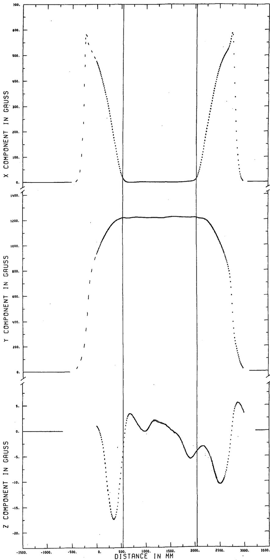
Fig. 16 Magnetic field components measured along the cooling axis (ion trajectory). The vertical lines indicate the limits of the cooling solenoid.
