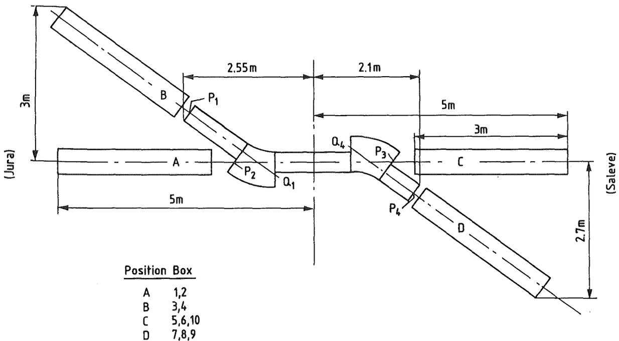
Fig. 6 Ground plan of the measuring site showing magnet reference points  $P_i$ ,  $Q_i$  (see text) and the positions of the scanning device (A-D) for the measurement of the field map boxes.
