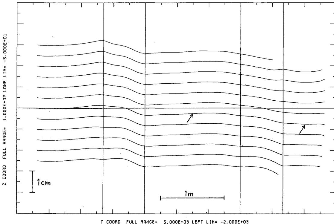
Fig. 22 Field lines started in a plane corresponding to the cathode of the electron gun. a) Lines started with horizontal displacements from the cathode centre, and shown in horizontal projection and in special coordinates (Appendix 3). b) Lines started with vertical displacements and shown in vertical projection. The field line from the cathode centre is marked by arrows. The bending plane of the toroids is in the horizontal plane (measuring position).
