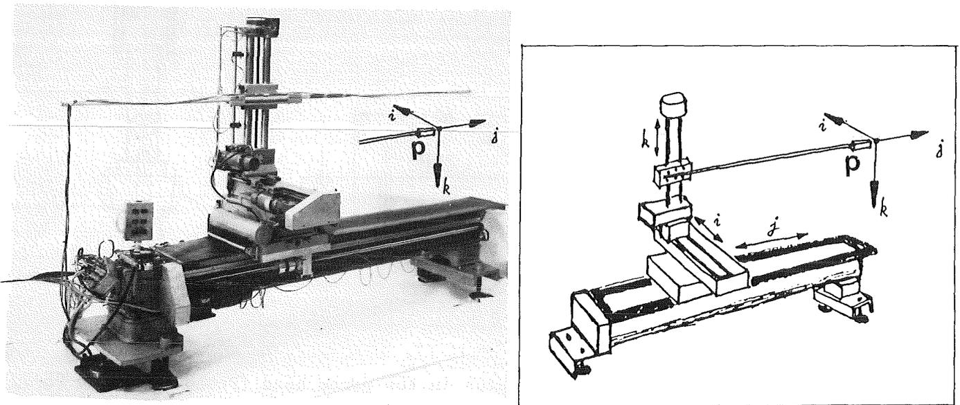
Fig. 3 The scanning apparatus with probe  $P$ . The orientation of the reference frame  $ijk$  is defined by the sliding rails as shown (Photo CERN 243-5-74).
