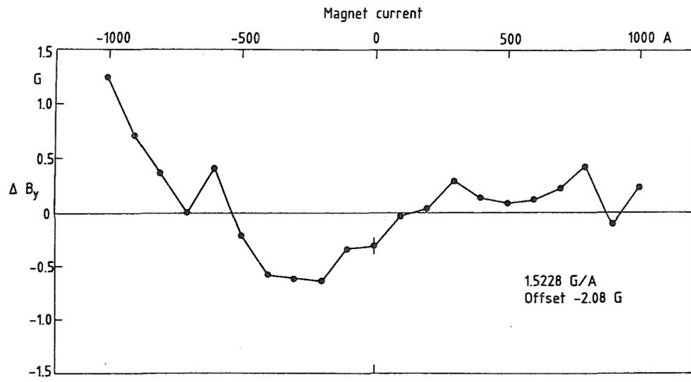
Fig. 12 Longitudinal field strength at the centre of the cooling solenoid measured for varying magnet currents. The deviations of the measured points from a fitted straight line with the parameters given are plotted.
