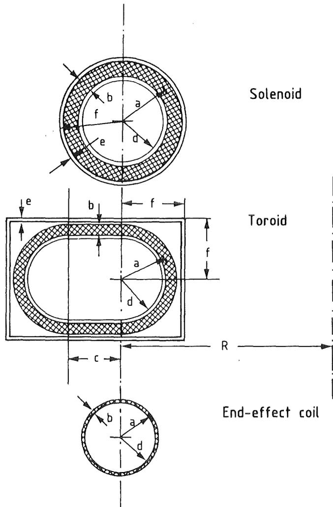
Fig. 2 Cross-sections of magnet coils and screening tubes, the dimensions are given in Table 1.
