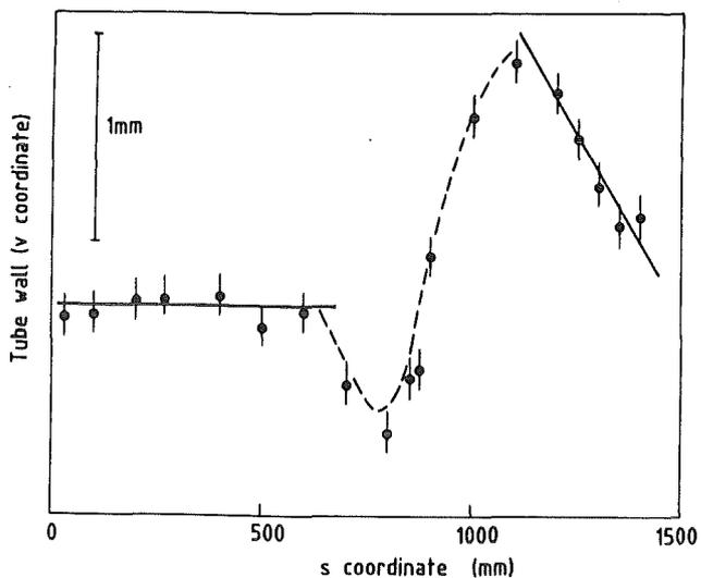
Fig. 18 Profile of the outer wall of the cooling solenoid screening tube measured along a straight line with  $s \approx 0$ ,  $v \approx 200$  mm.
