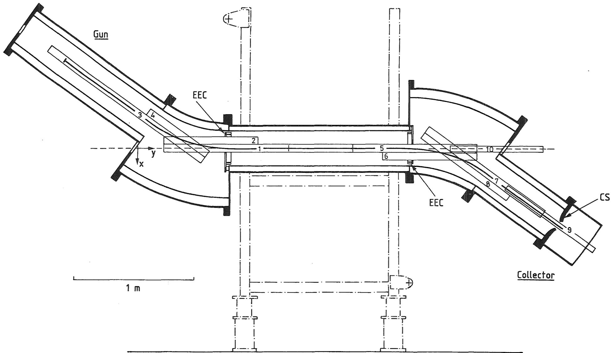
Fig. 1 The magnet assembly, including end-effect coils (EEC), screening plates at gun solenoid and toroids, and the magnetic shunt at the collector (CS). The centre line of the electron beam and the limits of the measuring boxes (1-10) for the field map are also shown.
