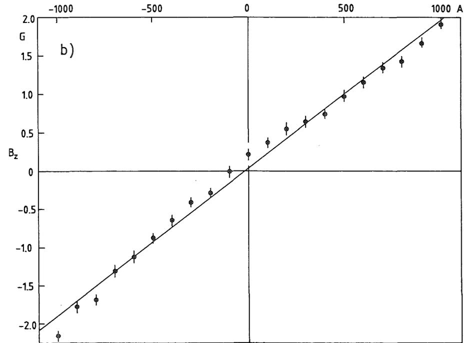
Fig. 13 Transverse field in the cooling solenoid measured for varying magnet currents; a) x component, b) z component.
