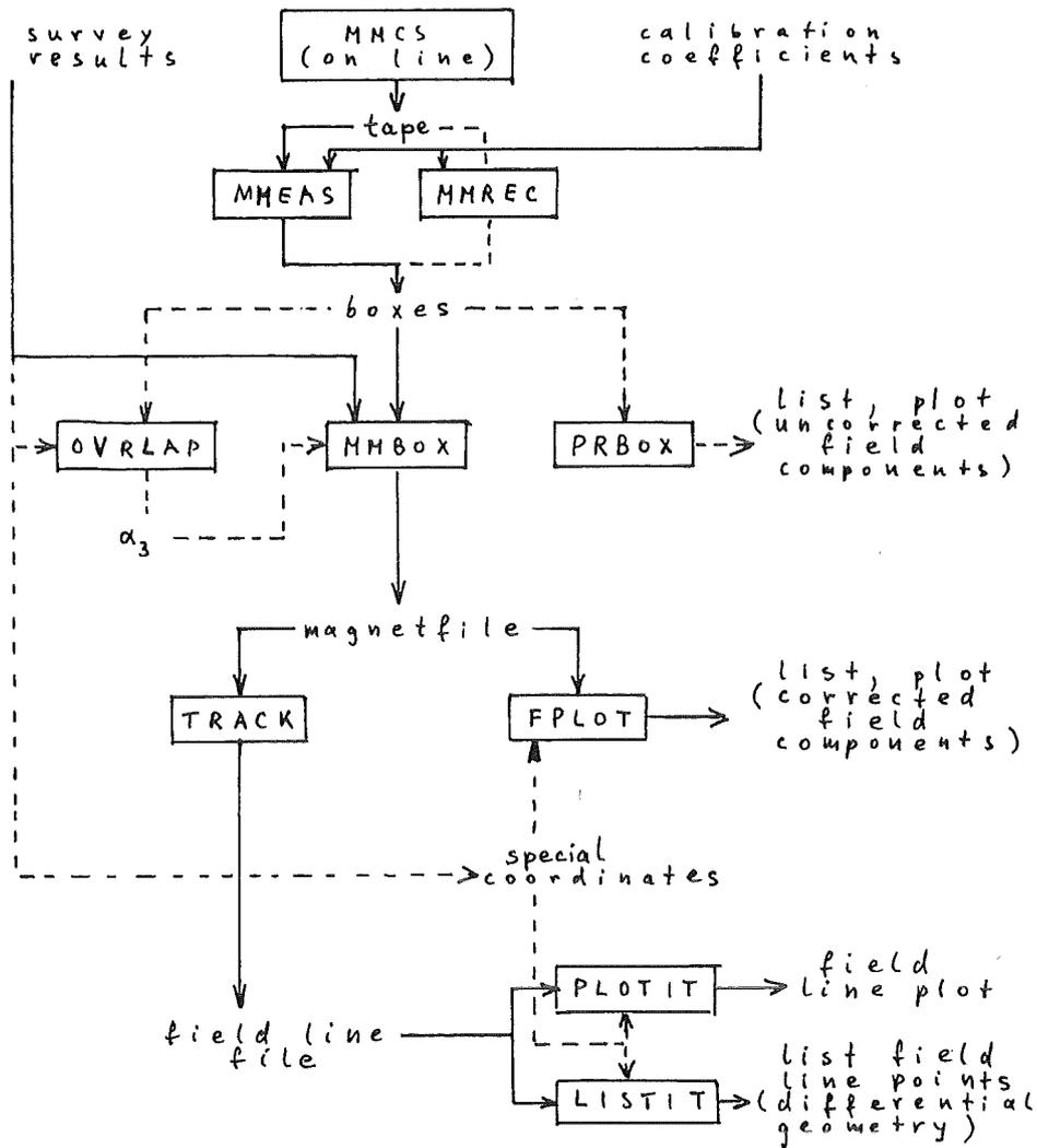
Fig. A.1 Data flow chart showing programs and data sets used for the evaluation.
