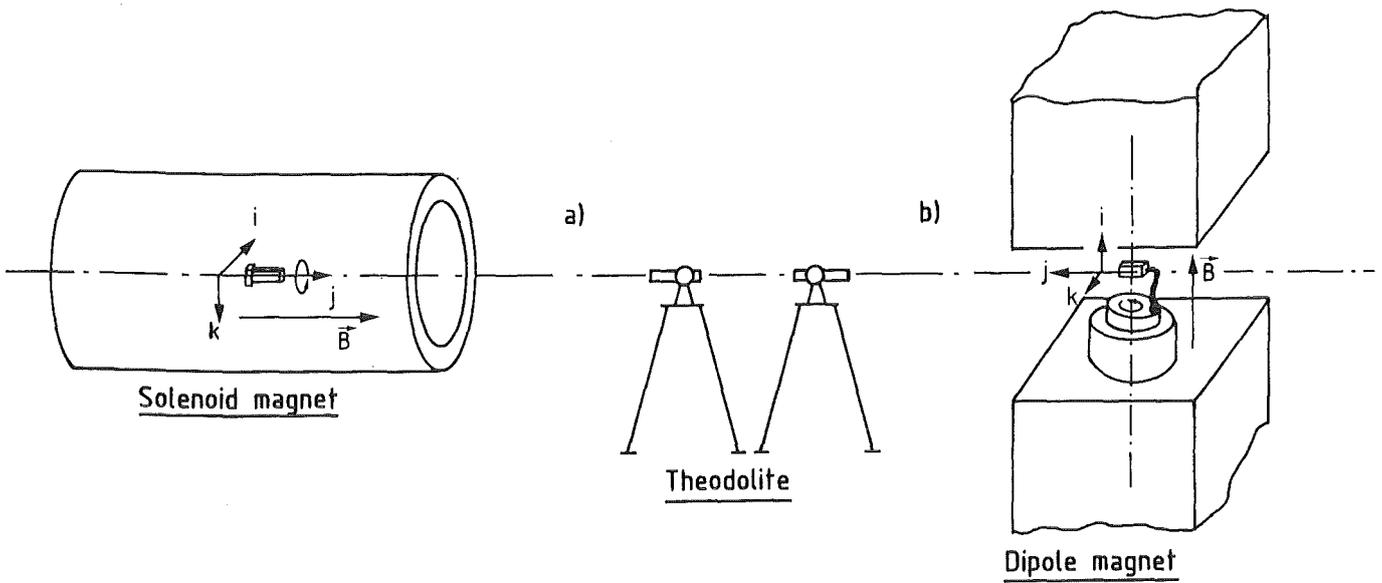
Fig. 5 Set-ups for the determination of Hall-plate misalignments as described in the text, by: a) rotation of the probe about the  $j$  axis, b) rotation about the  $i$  axis.
