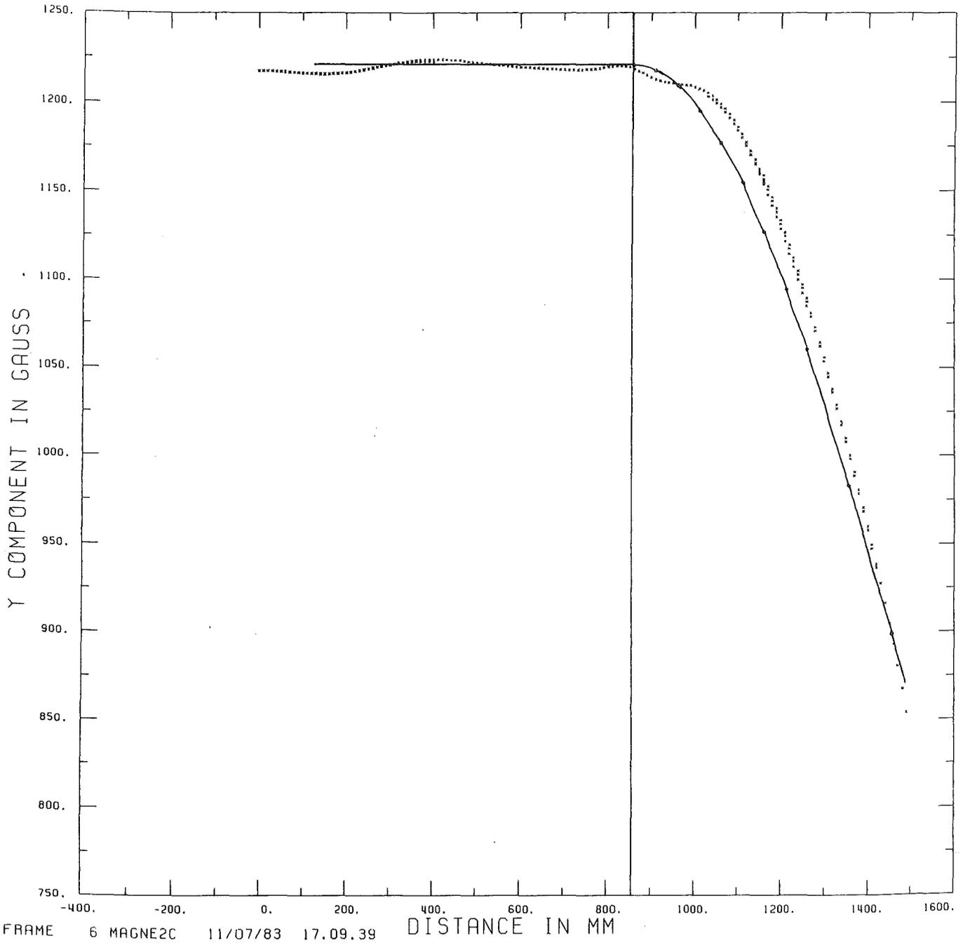
Fig. 11b Field component  $B_y$  in the collector toroid, measured and calculated [line from Eq. (9)].
