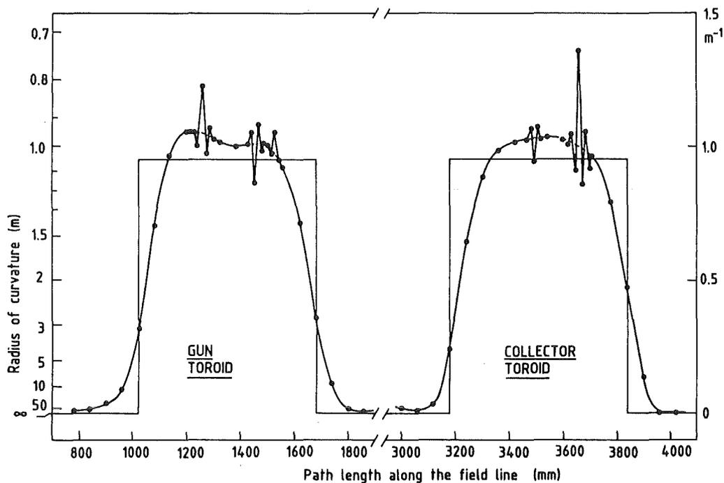
Fig. 20 Radius of curvature of a field line started in the gun solenoid along its path through the toroids.
