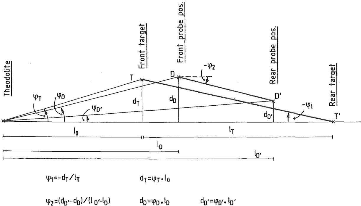
Fig. 8 Determination of the scan axis  $DD'$  relative to the known target axis  $TT'$  from theodolite readings  $\varphi_T$ ,  $\varphi_D$ ,  $\varphi_{D'}$ . The same construction is used for horizontal and vertical angles, which are all assumed to be  $\leq 10$  mrad.
