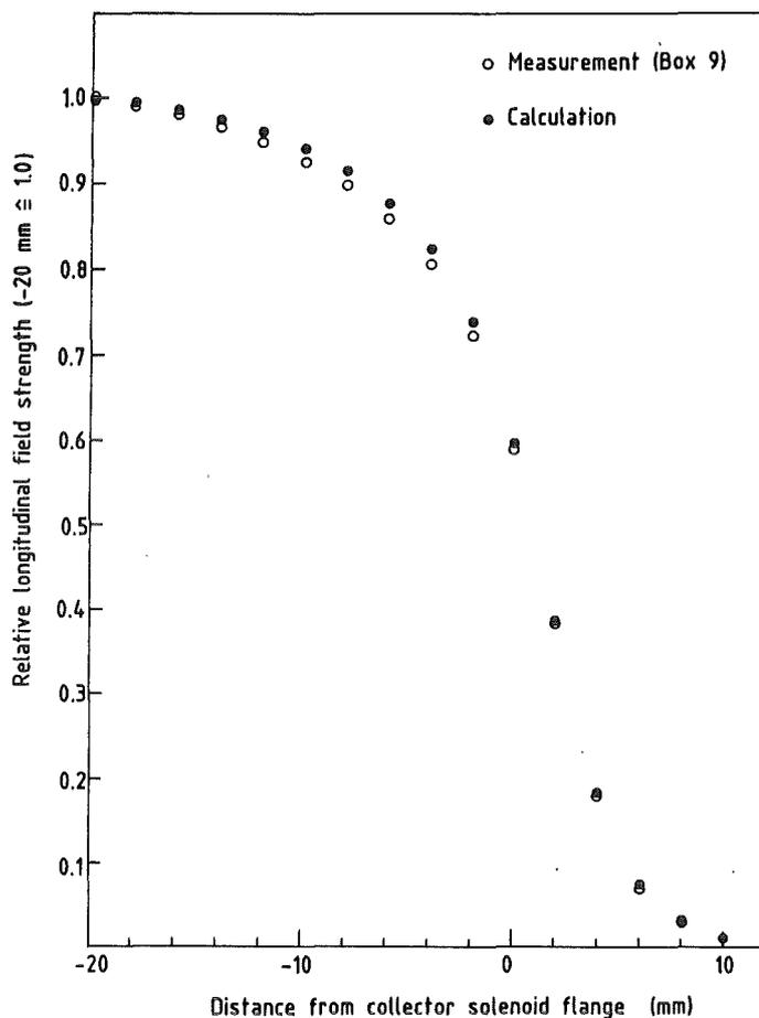
Fig. 19 Measured and calculated longitudinal field strength at the collector entrance (normalized results).
