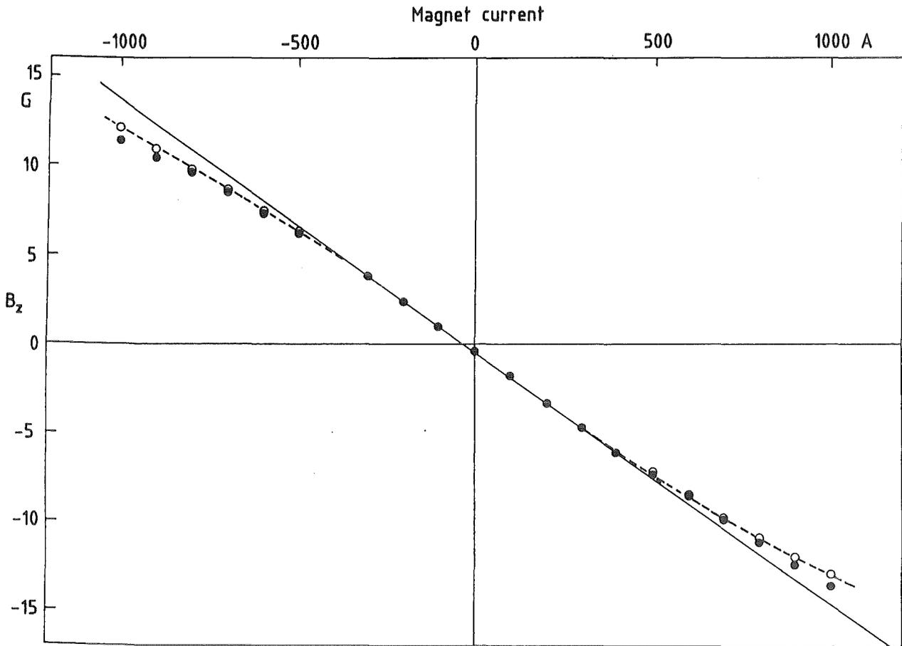
Fig. 14 z component of the magnetic field in the collector toroid measured for varying the magnet current (full circles: measured points, open circles: after subtraction of symmetrical contributions, see text).
