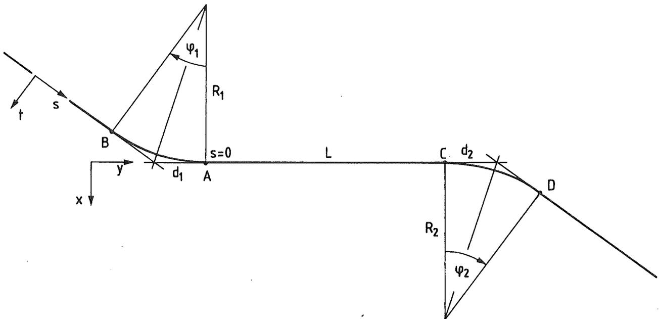
Fig. A.2 Reference points and parameters of the special coordinates for the electron cooling geometry.
