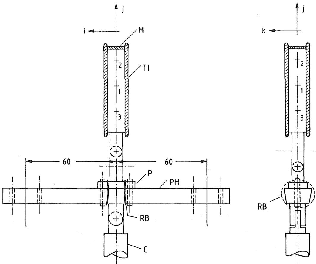
Fig. 4 a) Arrangement of the Hall plates in the probe head (Photo CERN 382-06-77); b) Probe head assembly with Hall plates 1-3 in a thermal insulation TI, and front mirror M. The head is mounted on the probe holder PH by a plug P which is pressed onto the precisely manufactured front plane of PH by a rubber band (RB). The tip of the ceramic tube C is also shown.
