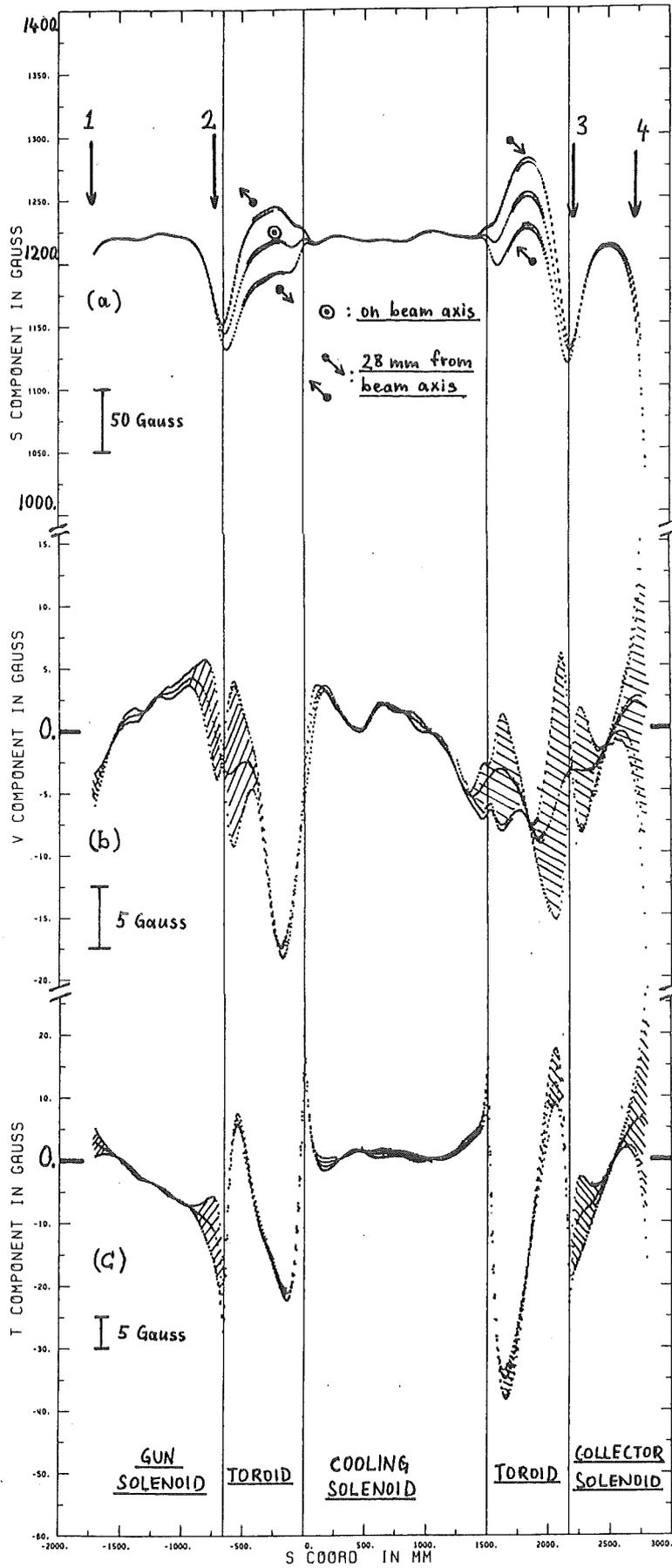
Fig. 17 Magnetic field components along the electron beam:
