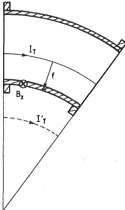
Fig. 15 Estimation of the magnetic field in the z direction produced by the current in the third toroid coil layer (see text).
