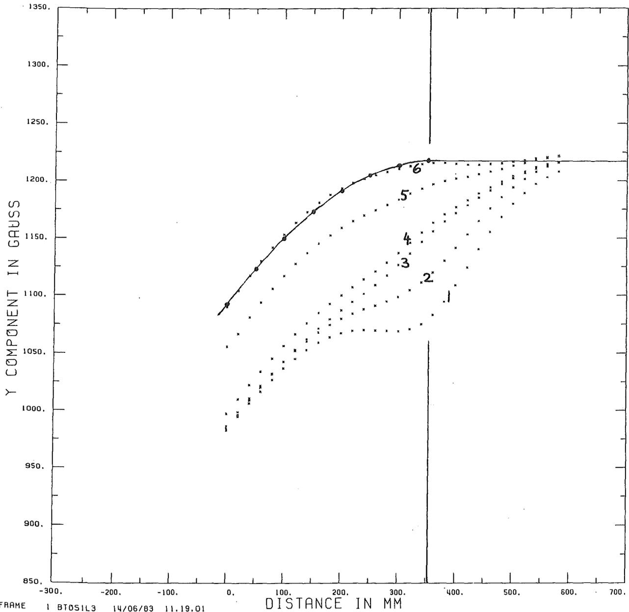
Fig. 10 Field trimming at the gun toroid as described in the text. The vertical line indicates the solenoid/toroid junction.
