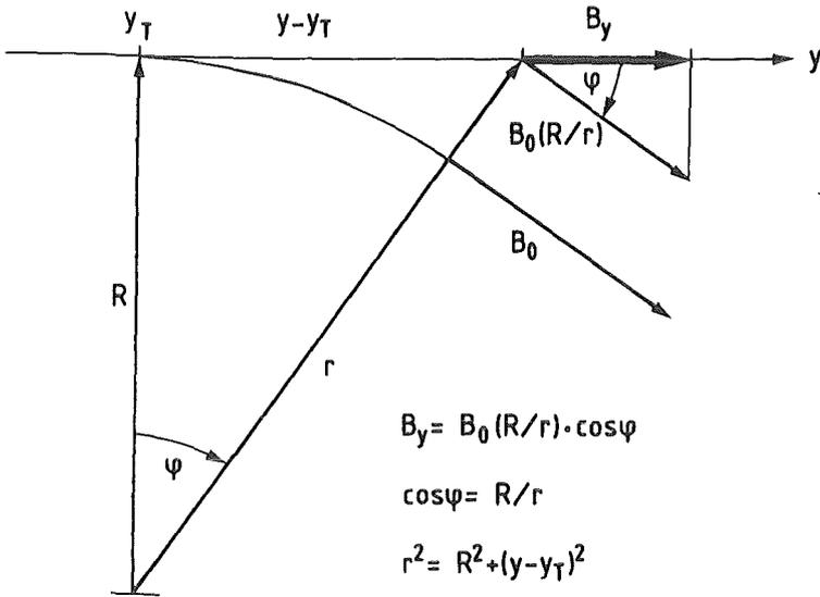
Fig. 9 Calculation of the field strength  $B_y$  in the toroids, assuming a perfect toroid field.
