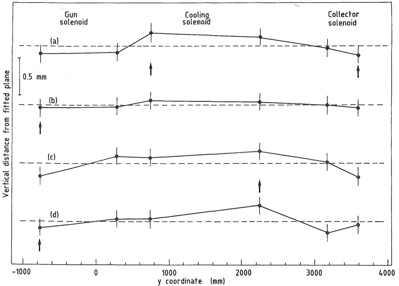
Fig. 7 Vertical deviations of test points on the magnet flanges from a fitted plane (magnet deformation test). The test points and the positions of mechanical supports (arrows) are plotted over their y coordinates for different support arrangements (a-d); d is the final situation.
