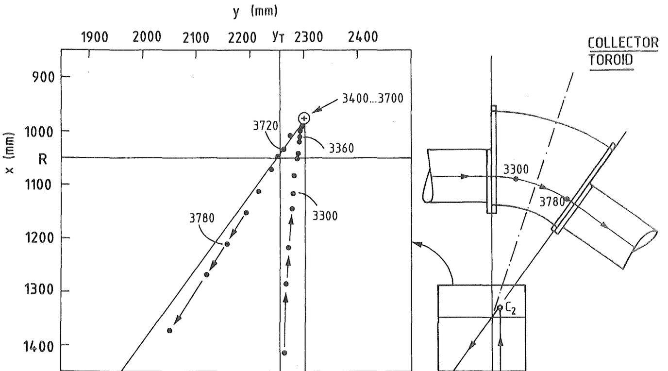
Fig. 21 Map showing instantaneous positions of the centre of curvature in the toroid bending plane along the path of a field line. Arrows show the sense in which the field line is followed, and numbers indicate the path length along the line in mm. a) Gun toroid, b) collector toroid.
