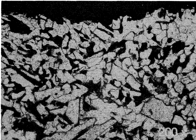
Fig. 6 Optical micrograph of cast steel after 1 year immersion in Q-brine at 90°C and a gamma dose rate of 10 Gy/h
