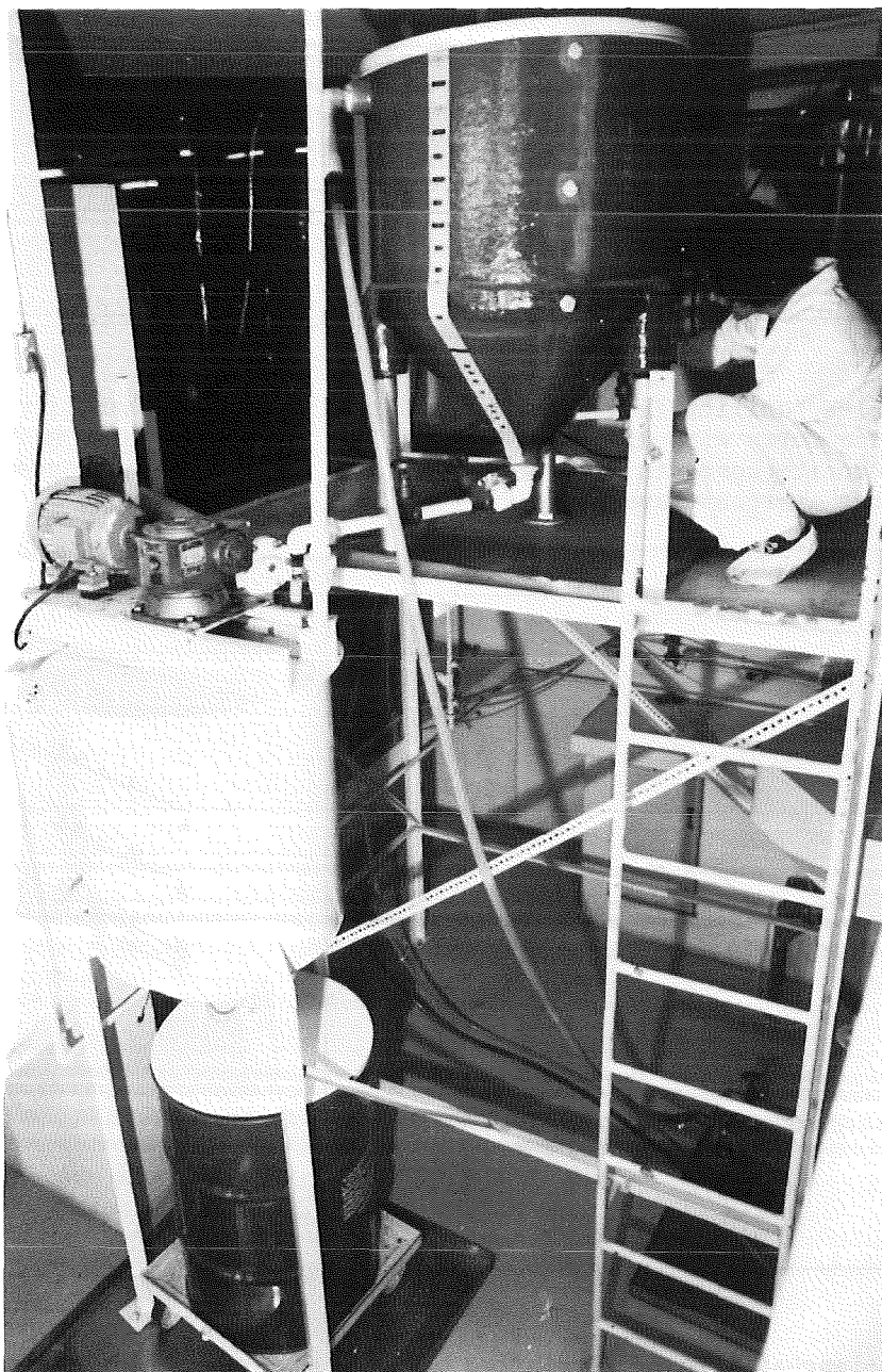
Fig. 11: In-Tank Mixing Cementation Pilot Plant
