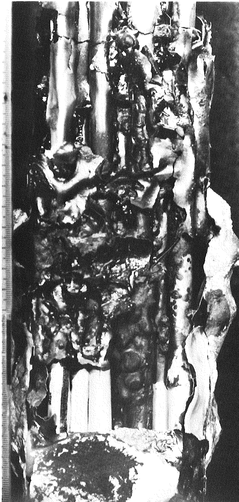
Fig. 33: Some details of the center region of the bundle CORA-5 after the test. Beside relocated melts one can recognize embrittled cladding material and fuel fragments.
