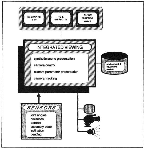
Figure 25. Concept of integrated viewing. The integration of artificial viewing using sensor controlled computer graphics with standard TV unifies and simplifies the work of the camera operator. The goal is to provide one tool for one function.
