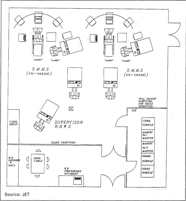
Figure 2. Remote Handling Control Room layout
