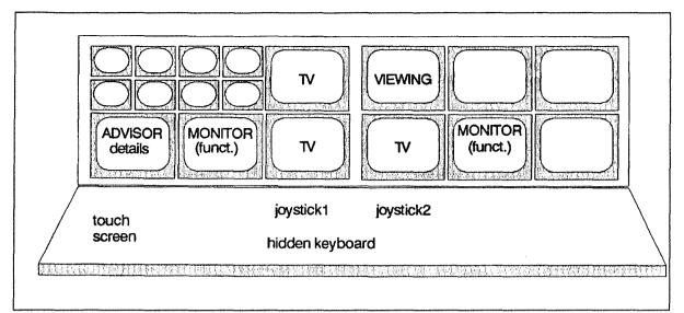
Figure 38. NRWS-panel for tool control. This panel is designed as a one operator place for controlling for example a welding machine.
