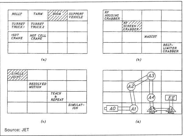
Figure 4. Menu sequence on touch panel. Successive TP pages for the control of the articulated boom.
