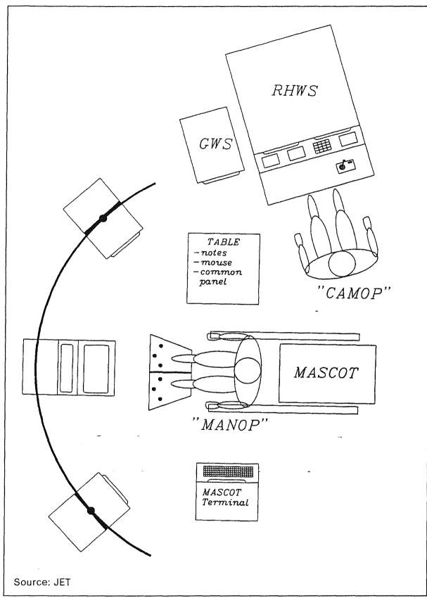
Figure 8. Servo Manipulator Master Station. Layout
