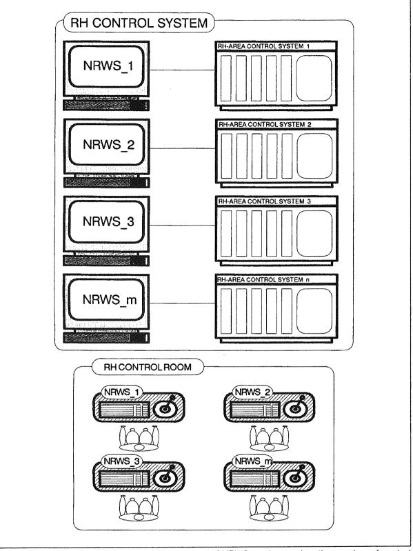
Figure 16. Special purpose NRWS. The number of NRWSs m is equal to the number of control systems n (m = n = 5...7).
