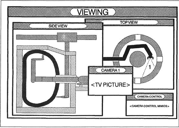
Figure 43. Viewing window. Support the operator in scene surveillance. The example shows the side and top view of a torus. A special window overlays the the picture of the camera 1 onto the animated graphics. In the top view the viewing angle of the camera is marked. A further subwindow provides a camera control interface.
