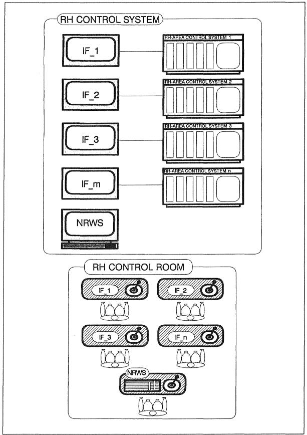
Figure 17. Off-line NRWS. The control system are only directly equiped with a relatively simple operating interface. High level support tools are implemented in the off-line NRWS.
