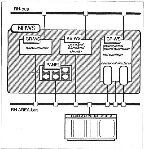
Figure 33. NRWS hardware architecture. Integration of workstations to the NRWS is done by using suitable software providing hardware independence (X-windows). GR-WS: Graphic Workstation, GP-WS: General Purpose Engineering Workstation, KB-WS: Knowledge-based Workstation, PANEL: Input devices and display screens integrated by X-window technique (Client). This integration of a panel is not state of the art.
