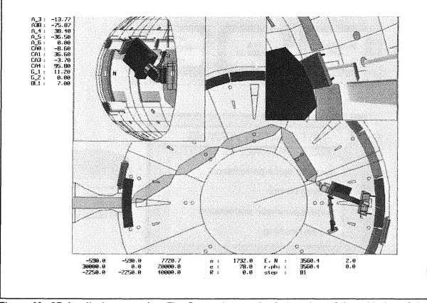
Figure 26. GBsim display example. The figure shows a basic top view of the mid plan of the JET torus, a side view (up left), and a simulated camera view (up right)
