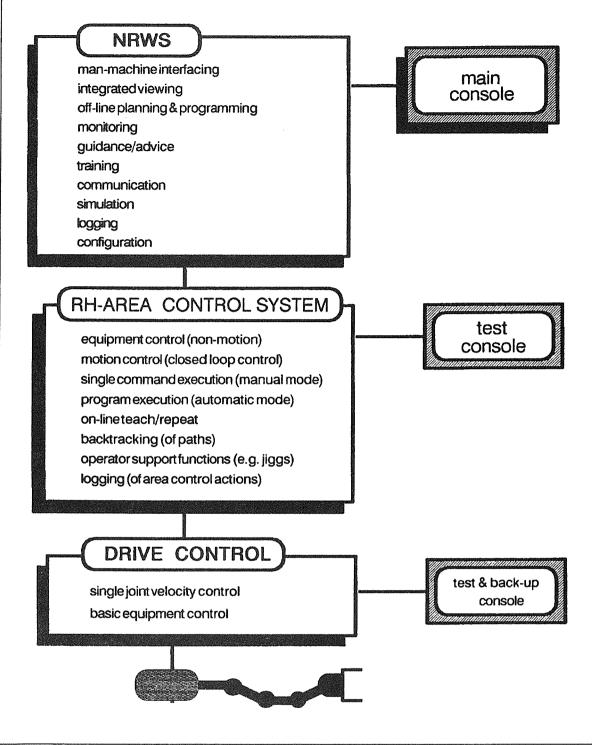
Figure 23. Functionality of control system levels. The NRWS represents the task level support and the man-machine interface, the RH-area control system represents the motion control level
