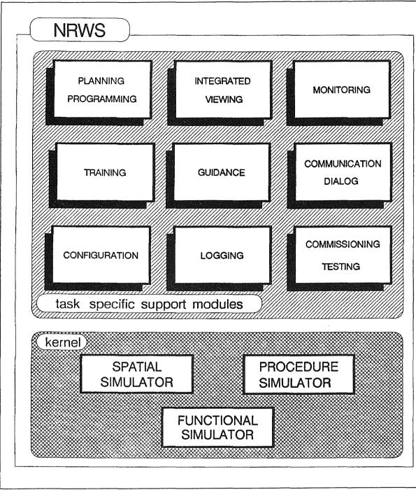
Figure 32. Functional modules of NRWS. The task specific support modules are using the kernel modules which provide the basic functions of simulation, monitoring, editing, and presentation.
