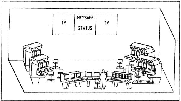
Figure 22. Remote handling control room layout (spatial). Layout example using standard control room equipment and showing one workstation of each type. This spatial layout is not the result of ergonomical investigations, but only a first approach, showing a possible arrangement of components considering communicational aspects.
