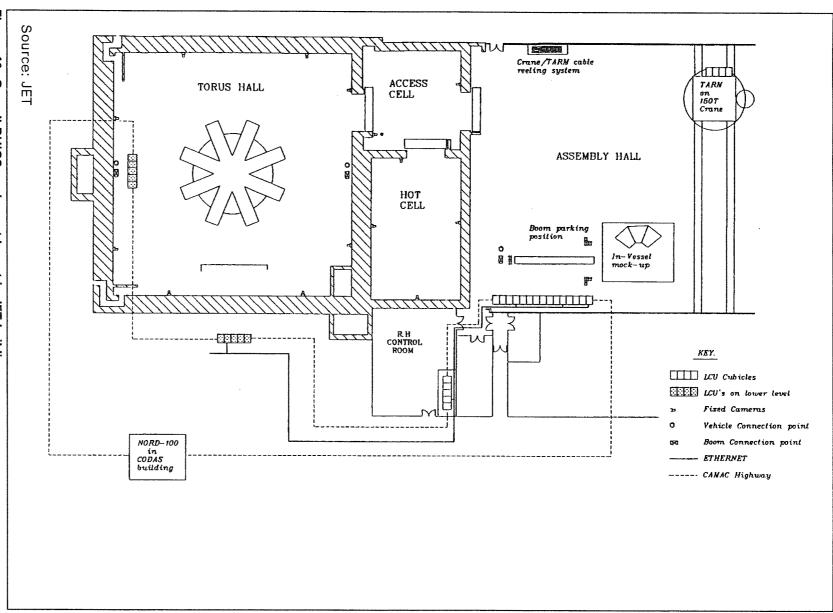
Figure 12. Overall RHICS equipment layout in JET building
