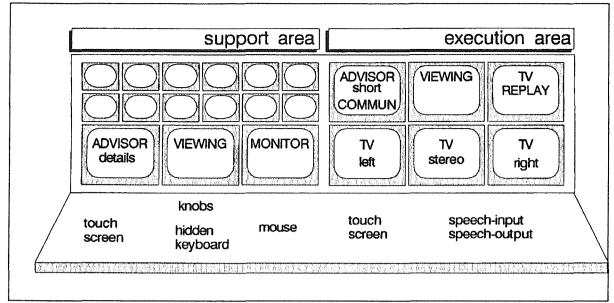
Figure 36. NRWS-panel for master-slave manipulator control. The executing operator (MSM operator) is mainly using speech input, the main displays for him are TV displays and the VIEWING display. The support (camera) operator is mainly using the VIEWING display.
