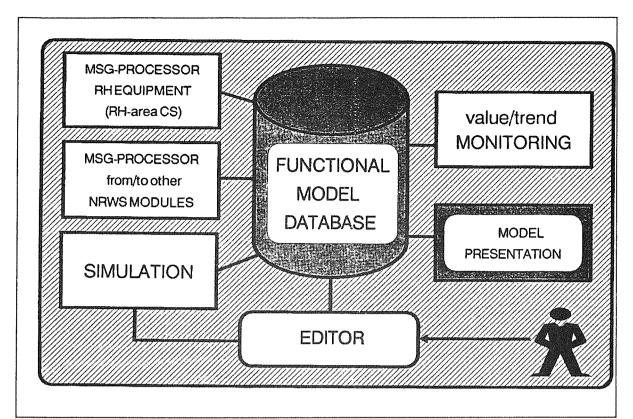
Figure 31. Architecture and usage of functional simulator. For synchronization of the simulator and the control system a special interface is provided, for communication with related NRWS modules (e.g. spatial simulator) a separate interface is available. The system provides modules for value and trend monitoring. The development of functional models is supported by an editor.
