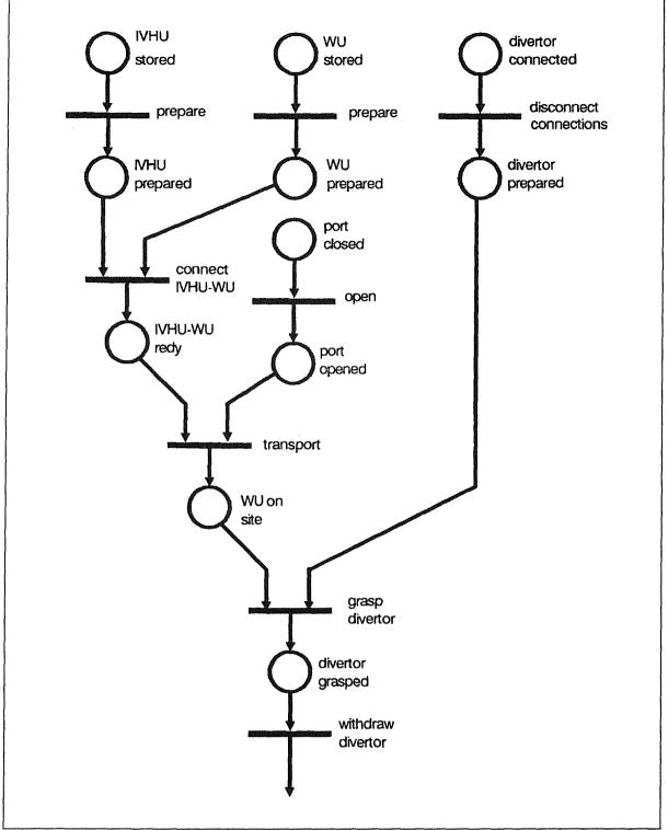
Figure 28. Example of an action net. These nets are used for high level planning and programming including especially the actions of the operator and the whole functionality of the control system. True state descriptions will be marked by a point in a circle (by tokens). The token flow through the structure represents the progress of work.
