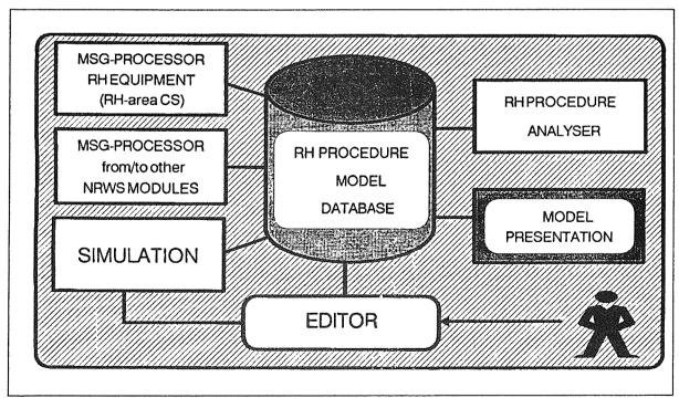
Figure 30. Architecture and usage of procedure simulator. For synchronization of the simulator and the control system a special interface is provided, for communication with related NRWS modules (e.g. spatial simulator) a separate interface is available. Procedures may be analysed by various modules in the planning phase and monitored during execution. Development of the procedure models is supported by a special editor.
