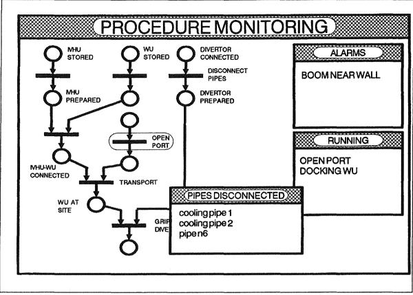
Figure 45. Procedure monitor window. The actual state of e.g. divertor exchange is presented by an action net. Subwindows provide information about a piping subtask, running subtasks, and alarms (warnings).
