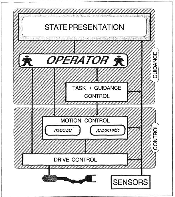
Figure 19. Architecture of control and data flow in the control system. The operator is integrated into the control loop by providing him with all status informations and giving him the possibility of acting on the task control as well as on the motion control and drive control level. The functions of the guidance level are implemented on the NRWS, the functions of the motion control level run on the local controllers and/or the RH-area controller.
