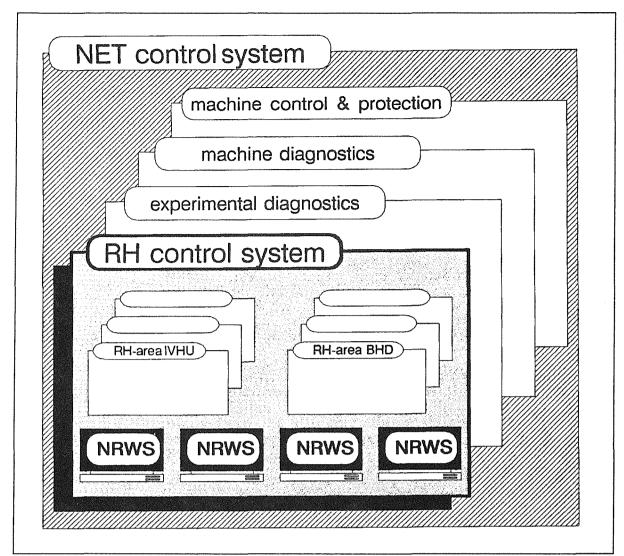
Figure 18. NET control system architecture. The RH control system is a subsystem of the NET control system. The RH control system itself is partitioned into RH-areas. To run a RH area a NET remote workstation (NRWS) has to be attached to the RH-area control system.
