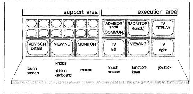
Figure 37. NRWS-panel for transporter & work unit control. The most important information for the executing operator controlling a work unit with a joystick are two TV screens and the VIEWING screen. The support operator controls the transporter by a joystick mainly via a VIEWING screen.
