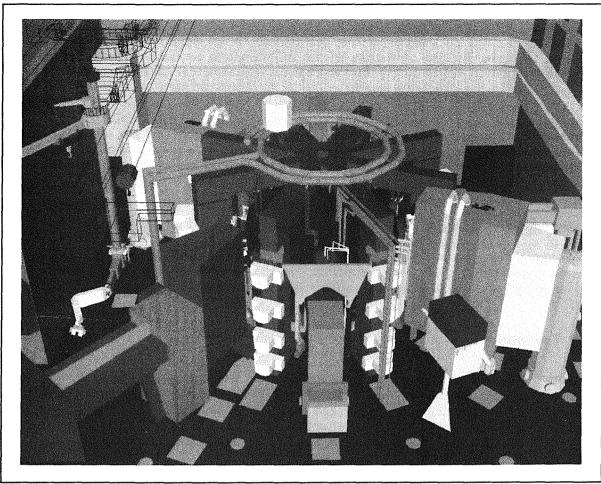
Figure 27. KISMET display example for JET-TARM control. The display shows a birds eye view of the JET torus (ex-vessel view) and the TARM (left hand side)
