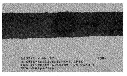
Fig. 4.3-3 Metallurgical cut through an FCI with glass as insulator
