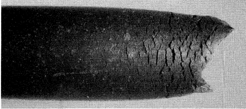
Fig.13: Extensive secondary cracking of the 15 MnNi 6.3 steel tested in Q-brine at 170°C, 13 MPa and 10^{-5} \text{ s}^{-1}
