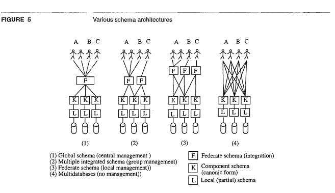
In the first approach, a *single* so-called *global schema* is used for the integration of all partial schemas involved. This global schema is made available to all system users in an identical form and managed centrally by a \_global\_ database administration. Access to the partial schemas always takes place via the global schema.
