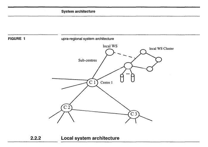
The sub-centres mentioned above consist of local workstations or clusters of workstations. Various Unix derivates are applied as operating systems. Accordingly, the hardware used is rather heterogeneous. Each sub-centre is equipped with a relational database management system (e.g. Oracle, Ingres) at least. It will be the main task of the locally responsible system managers to describe access to \_their\_ data correctly and to harmonize updates with the main centres.
