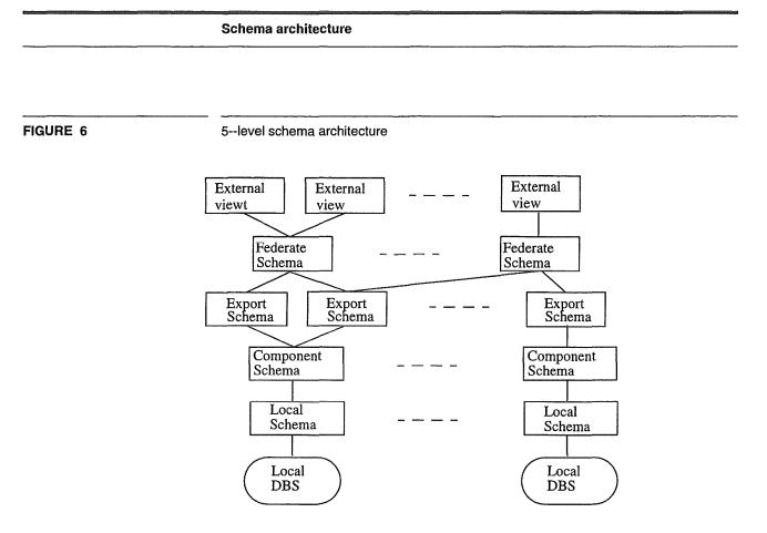
To sum up, all approaches can be represented by the so-called 5-level schema architecture. From the bottom to the top, this architecture consists of the partial database system with a local and a partial schema in canonic form. The partial schemas are made available as export schemas and integrated by means of federate schemas. For the latter, external views can be defined and accessed by the applications.
