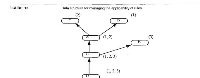
This diagram has the following meaning: each node exactly corresponds to a literal of the rules. At each node, the depending rules are given in brackets. If rule 1 shall be applied and it is found that A does not exist, rule 2 can be excluded at the same time.
