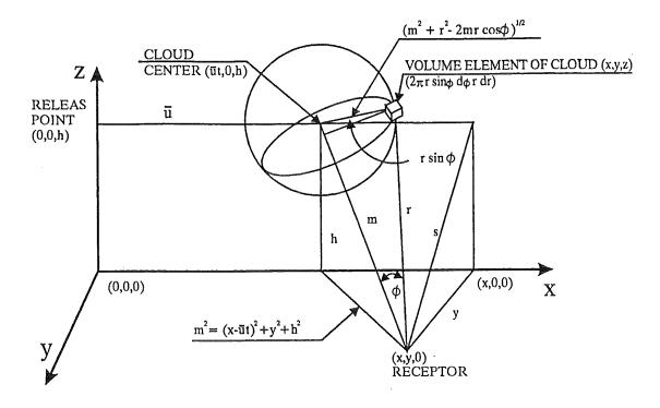
Fig. 7: Coordinate system for cloud gamma-dose calculations
