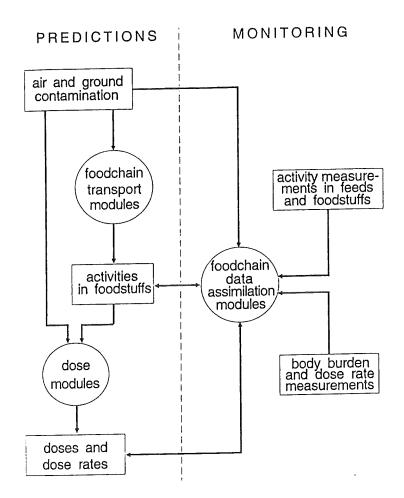
Fig. 4: Basic structure of ASY, food contamination and dose assessment
