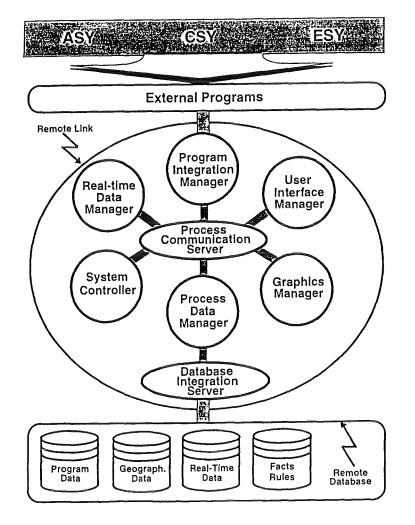
Fig. 21: Modular design of the operating subsystem OSY
