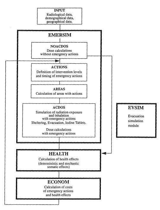
Fig. 16: Sequence of modules for calculating radiological and economic consequences
