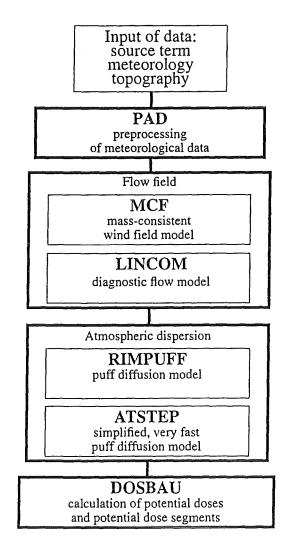
Fig. 10: Sequence of modules in ASY
