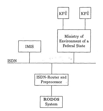
Fig. 24: Example on-line connection of the RODOS System
