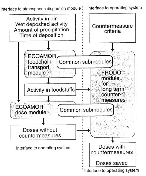
Fig. 11: Data flow in the food chain transfer and dose module ECOAMOR and the long term countermeasure module FRODO within the RODOS system
