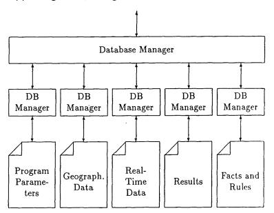
Fig. 23: Structure of the RODOS distributed data base
