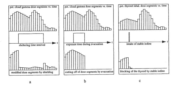
Fig. 14: Modelling of the effect of protective actions on doses a) Sheltering, b) Evacuation, c) Administration of stable iodine tablets
