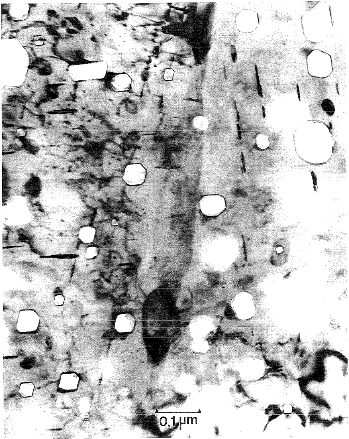
Fig. 8. He- bubbles appearing in the inner part of Sample 2 (Sample 2b).
