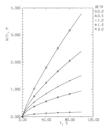
Fig. 3: Evolution of the interface  $x_f^+(t+t^*) - x_f^+(t^*)$ ,  $t^* = 1$ s.
