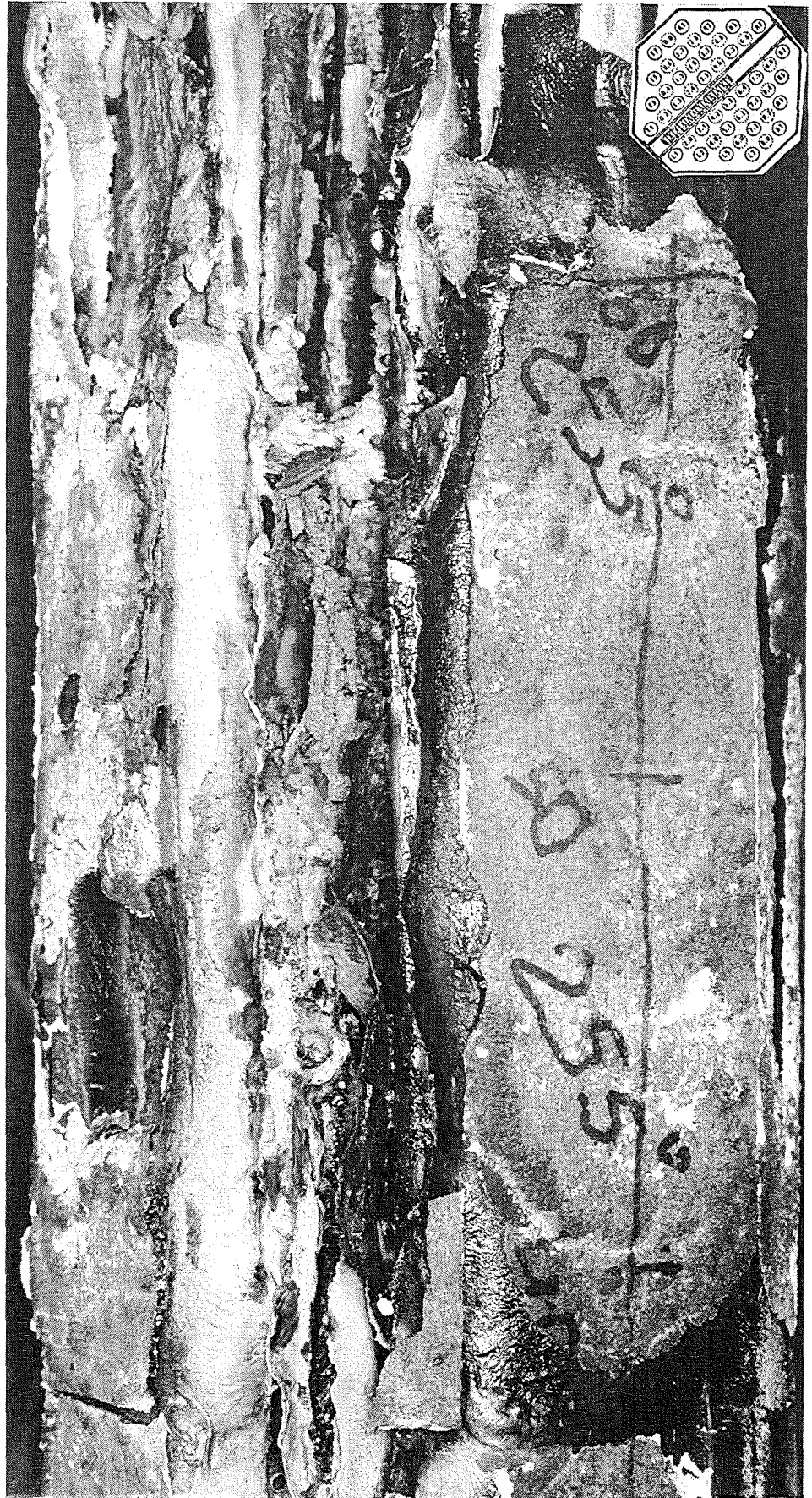
Fig. 94: CORA-18; posttest partial view at 285° orientatation; 350 - 650 mm elevation.
