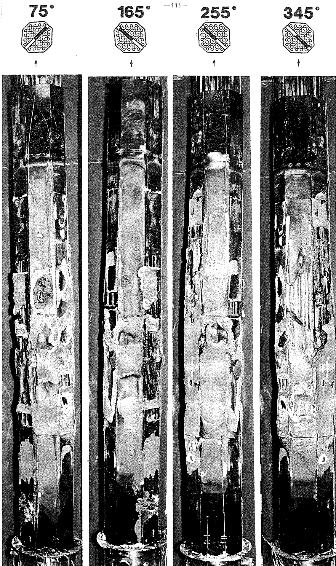
Fig. 83: CORA-18; posttest appearance of the shroud after removal of the insulation
