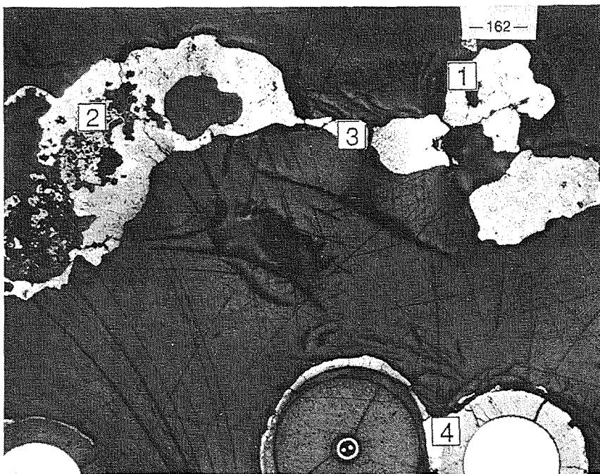
Oxidized surface of absorber melt Pos. 1
