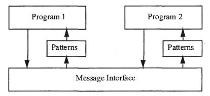
Figure 1: Message Interface of the RODOS System
