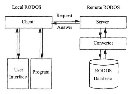
Figure 3: The Connection to Remote Databases
