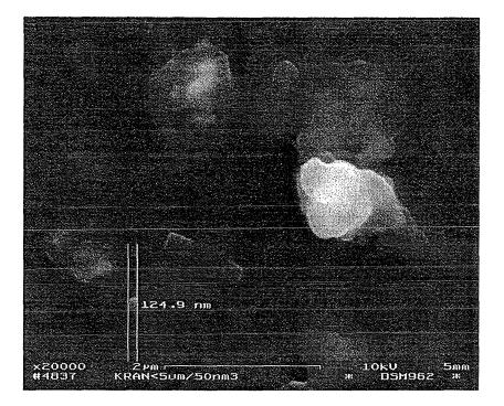
Fig. 6. SEM micrograph of the filter cake on a 50 nm Nuclepore filter. Prefiltration through a 5  $\mu$ m Filter.
