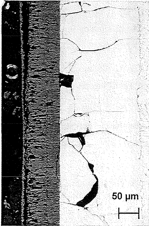
Fig. 1 : Cracks in the \alpha -Zry (taken from [ 1 ]).
