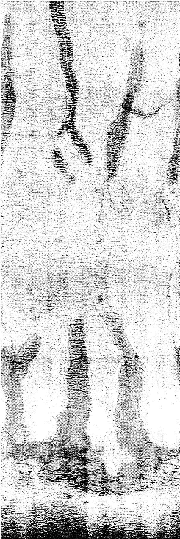
Figure 2.64: Cladding tube circumference of the experiment 02038_1 (1600 °C, 201 \mu\text{m} oxide layer thickness). Left: surface with red penetrant color; right: hand traced cracks.
