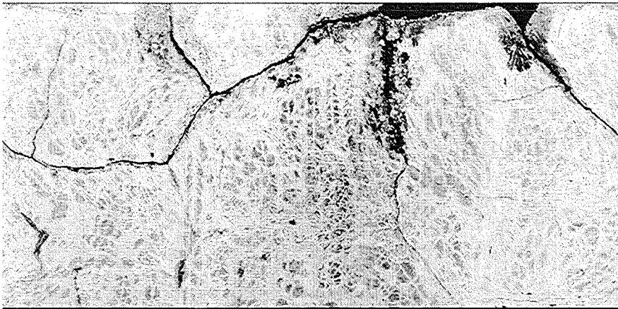
Hot region with cracks
