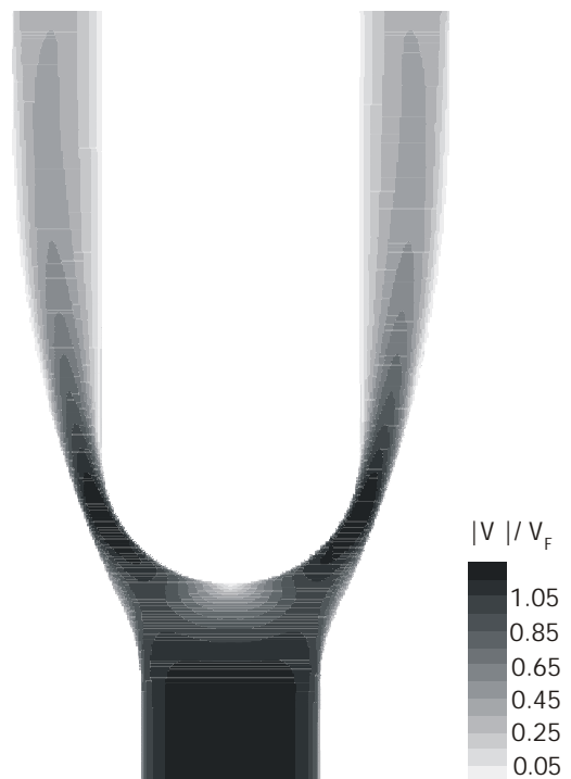
Figure 37: FLUTAN results with k-\epsilon model for low Reynolds numbers. Field of the modulus of the velocity for Re = 2 \times 10^4 .
