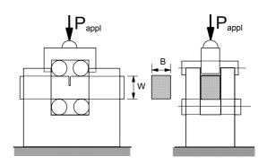
Fig. 1: Device for a 4-roller crack extension test
