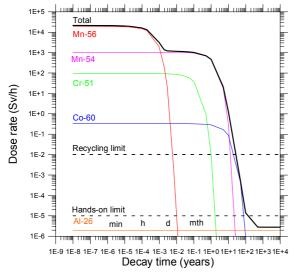
Fig. 1: Contact dose rate of EUROFER-97 after irradiation with 14-MeV neutrons of 1 MWa/m<sup>2</sup> as a function of decay time. Besides the total dose rate the contributions of dominant radionuclides are inserted
