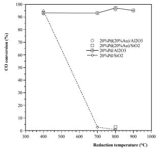
Fig. 3: Methanation activity on Pd/Au catalysts at 400°C
