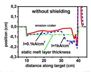
Fig. 9: Calculated crater profiles for a W FW armour for a VDE with 30 MJ/m<sup>2</sup> without shielding
