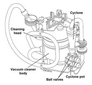
Fig. 1: Remotely operated flake collection vacuum cleaner
