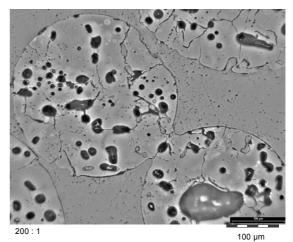
Fig. 4: Cross section of enriched pebbles after 96 day annealing at 970 °C
