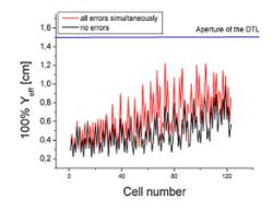
Fig. 7: 100% effective beam size in the Y-Ncell-plane of the DTL with and without combined quadrupole + rf field erors
