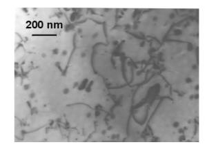
Fig. 2: Dislocations and Mg impurities (black dots) in beryllium after irradiation at 780 K: no gas bubbles are present. Material: pebbles from the BERYLLIUM experiment [3]
