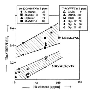
Fig. 3: Effect of He- content generated by  $^{10}$ B on relative decrease of ductile energy USE for various 7-12Cr steels at T<sub>I</sub>=250°C, 2.4 dpa
