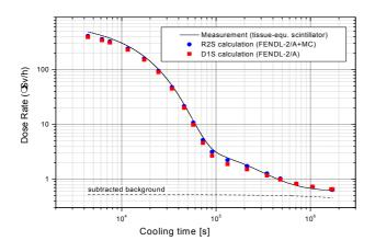
Fig. 3a: Comparison of calculated and measured dose rates
