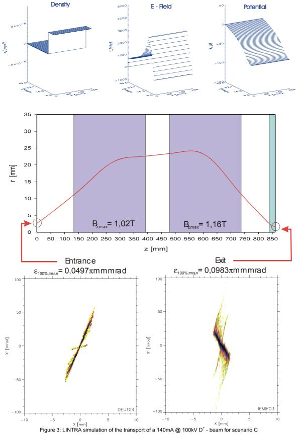
The first three graphs in figure 3 show the assumed electron density, the electrical field and the potential of the electron cloud from beam axis to the wall of the beam transport tube.
