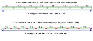
Fig. 8: Scaled scheme of the an Alvarez DTL and IH-type DTL for IFMIF
