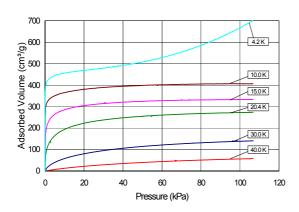
Fig. 5: Measured isotherms for helium
