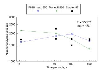
Fig. 1: Comparison of EUROFER 97 with two reference materials with tensile hold times under LCF loading conditions
