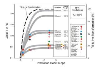
Fig. 4: Irradiation-induced shifts of ductile-to-brittle transition temperature and <sup>10</sup>B-to-He transformation vs. irradiation dose
