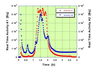
Fig. 2: Comparison between tritium thermal release of a bulk and a plasma exposed disk
