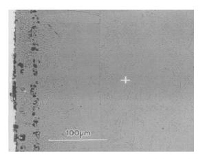
Fig. 1: Cross section of a HDA coated sample after 10000h exposure to flowing Pb-17LI Right side:steel matrix Left side: coating zone with adherent PbLi
