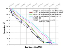
Fig. 4: The temperature traces during the cooldown of the TFMC test configuration
