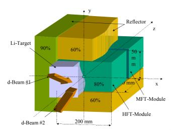
Fig. 1: Geometry and material distribution assumed for the neutronic calculations (x-axis: horizontal; y-axis: vertical; z-axis: beam downstream direction)
