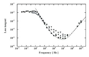
Fig. 1: The loss tangent of unirradiated (circles) and neutronirradiated (to 10<sup>21</sup> n/m<sup>2</sup>) KU1 (up and down triangles). [2]
