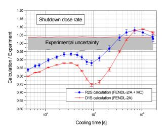
Fig. 3b: C/E (calculation/ experiment) comparison for the dose rate measured with the tissue-equivalent scintillator
