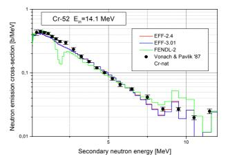
Fig. 2: Cr-52 neutron emission cross-section at 14 MeV incident neutron energy
