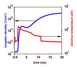
Fig. 12: Tungsten plasma density and temperature evolution at a distance of 1.5 m from the target at the position of maximum density
