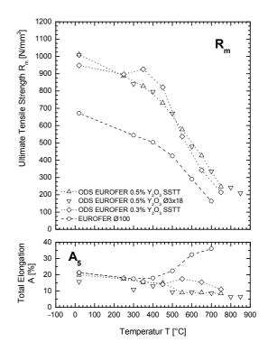
Fig. 1: Ultimate Tensile Strength and Total Elongation of different ODS Alloys compared to EUROFER 97
