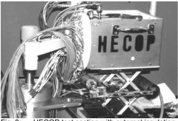
Fig. 3: HECOP test section with external insulation
