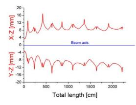
Fig. 9: 99% transverse effective beam envelopes along the IH-DTL
