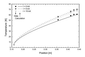
Fig. 2: Measured and calculated temperature profiles along the HTS part (Tube B) of the current lead during steady state operation.
