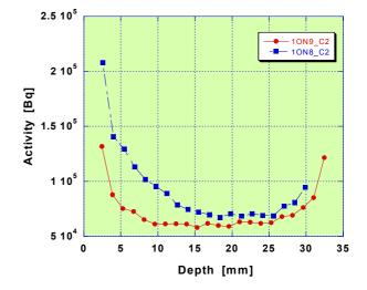
Fig. 1: Comparison between tritium diffusion profiles for tiles 8 and 9 retrieved from the JET outer divertor
