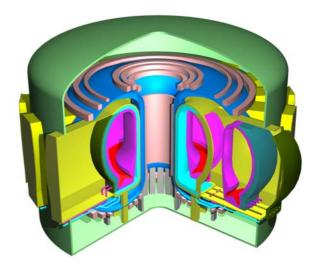
Fig. 1: Full Sector Replacement System (view into open torus, sector partly withdrawn)
