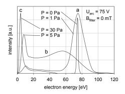
Fig. 3: Electron energy distribution as function of different gas pressures (arc current) at low input powers
