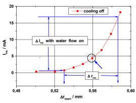
Fig. 1: Mechanical vibration of the coaxial insert under operating conditions. The marked point indicates the position before turning on the water flow
