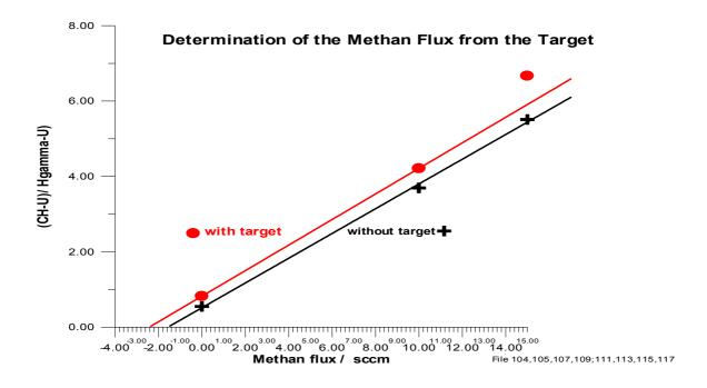
Fig. 2: Intensity of the CH-band at  $\lambda$  = 430 nm normalized to H<sub>a</sub> with and without the graphite target exposed to the plasma. An additional injection of methane causes a linear increase of the CH photon flux
