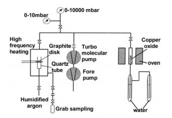
Fig. 1: Experimental set-up for the RF detritiation
