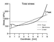
Fig. 1: Example for the application of SDC design rules to BTM first wall (decomposition of stress)
