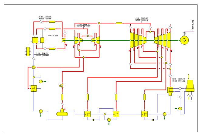
Fig. 1: Steam circle for the HCPB-Power Plant Conceptual Study
