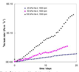
Fig. 2: <sup>4</sup>He leak rate of ferrofluidic seal for various pressure differences
