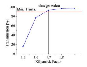
Fig. 1: Transmission as a function of the electrode voltage of the RFO
