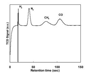
Fig. 3: µTCD chromatogram of the µGC with HayeSep capillary
