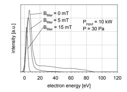
Fig. 5: Electron energy distribution for different magnetic filter field strengths
