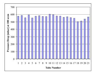
Fig. 1: Pressure drop of the different PERMCAT tubes
