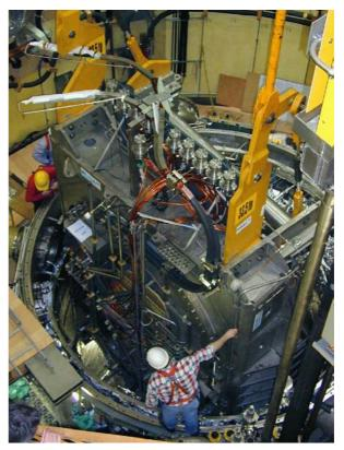
Fig. 3: The ITER TFMC configuration during lifting into the TOSKA vacuum vessel
