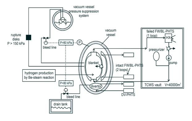
Fig 1: Ex-vessel LOCA scenario without plasma shutdown, leading to in-vessel break and injection of steam and air into the vacuum vessel. Burst membranes open flow paths to the safety systems when the differential pressure exceeds 0.8 bar
