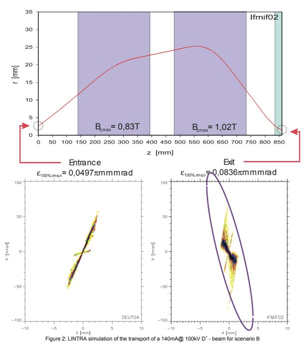
Figure 2 shows results of simulations gained from the LINTRA code under assumption of a global compensation degree of 90% and a decompensation drift section of 30mm at the end of the LEBT system to simulate the entrance of the RFQ structure (scenario B).
