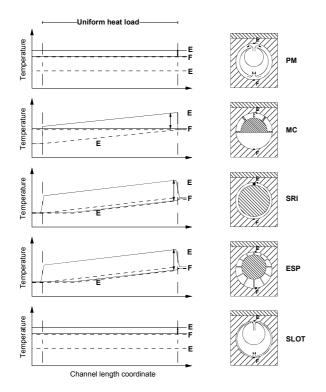
Fig. 2: Characteristic temperature profiles along the coolant flow path ( — wall temperature, - - coolant temp.)
