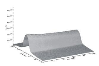
Fig. 3: Intensity of incident light detected by a CCD camera as a function of transversal and longitudinal position (see text)
