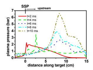
Fig. 5: Time dependent profiles of the external pressure from the plasma shield as calculated with FOREV-2 for a disruption case with 30 MJ/cm<sup>2</sup> and a time duration of 10 ms
