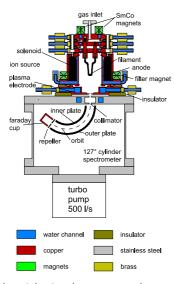
Fig. 1: Experimental setup: ion source and energy analyzer, not in scale
