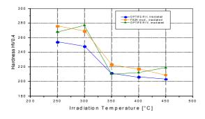
Fig. 2: Vicker Hardness HV0.4 of HFR la specimens
