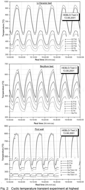
Fig. 2: Cyclic temperature transient experiment at highest heating plate performances, measured temperatures within the pebble beds and the first wall
