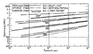
Fig. 2: Stress dependency of minimum creep rate for 3 RAFM-steels
