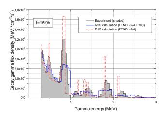
Fig. 4: Comparison of measured and calculated decay gamma ray spectra at 15.9h after irradiation
