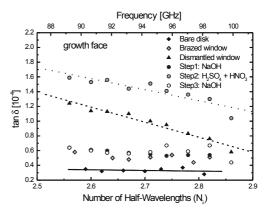
Fig. 6: Apparent dielectric loss values measured at 90-100 GHz at different testing stages of the Maquette window
