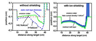
Fig. 8a Fig. 8b. Calculated crater profiles in a Be FW armour for a VDE with  $30 \text{ MJ/cm}^2$  for the two values of the Halo current of 0.1 and 1 kA/cm<sup>2</sup> without shielding (a) and with shielding (b)
