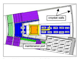
Fig. 1: Mid-plane port section of MCNP model (horizontal cut)
