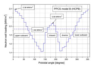
Fig. 1: Poloidal wall load distribution calculated with MCNP for PPCS plant model B (HCPB blanket). The total fusion power is 3300 MW
