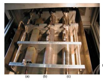
Fig. 5: Test sections being installed in the MEKKA-facility of the Forschungszentrum Karlsruhe. (a) Test section with electrical separation of liquid metal containing duct from rectangular shaped structure material. (b) ferromagnetic thick walled test section. (c) nonferromangetic stainless steel test section
