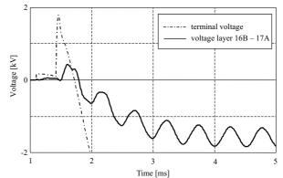
Fig. 2: Voltage at location of maximum transient insulation stress. At t = 1.42 ms the arc in the circuit breaker extinguishes and the current starts to commutate to the dump resistor path
