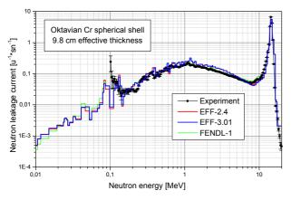
Fig. 1: Neutron leakage spectra of the Oktavian Cr transmission experiment.
