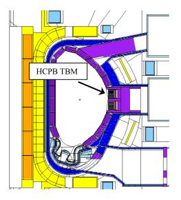
Fig. 2: Radial-poloidal cut of the MCNP model of ITER (with integrated HCPB TBM in the horizontal port) used for the nuclear analysis
