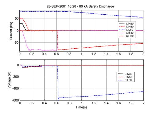
Fig. 6: Current and voltage traces during the current commutation from the power supply across the short circuit path in the dump resistor
