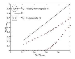
Fig. 7: Measured magnetic field inside the test section as a function of the externally applied magnetic field  $B_0$  for the MANET test section (a) and the ferromagnetic test section (b)
