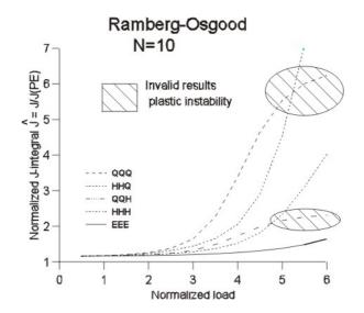
Fig. 2: Normalised J-Integral values for different size of CT specimen for Ramberg-Osgood material law with N=10 indicating regions where results are not ransferable
