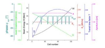
Fig. 5: Main structure parameter of the DTL versus the cell number
