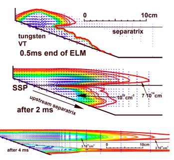
Fig. 11: Tungsten plasma density contours (thick lines) and plasma particle flux (plasma density times velocity, arrows) at 3 time moments. Peak target heat load at the SSP is 1 GW/m<sup>2</sup>. (10 GW/m<sup>2</sup> at the hot spot), wetted area 5%
