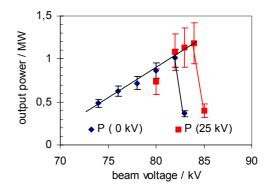
Fig. 3: Output power vs. accelerating voltage: without and with a depression of 25 kV
