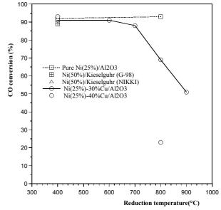
Fig. 1: Methanation activity on Ni/Cu catalysts at 400°C
