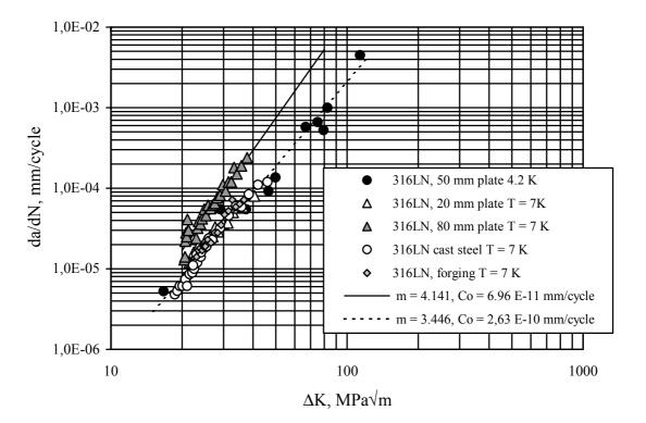
Fig. 3: FCGR of Type 316LN base materials at 7 and 4 K (R = 0.1). The lines along with m and C<sub>o</sub> show the mean of the determined Paris constants (m is dimensionless)
