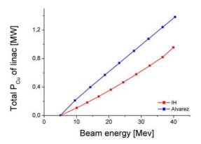
Fig. 12: Sum of the rf copper power losses per tank of both structures as a function of the beam energy
