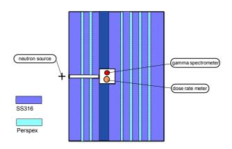
Fig. 1: Vertical cut of the experimental assembly
