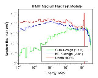
Fig. 2: Neutron spectra of IFMIF MFTM without moderator (CDA design 1996), and with W and C moderator/reflector (KEP design 2001) in comparison with the HCPB blanket of a DEMO-reactor
