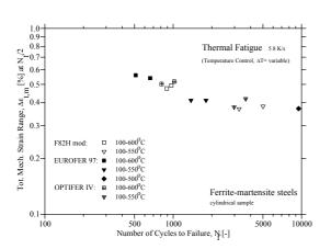
Fig. 2: Comparison of total mechanical strain range  $\Delta\epsilon_{t,m}$  of thermal fatigue behaviour between F82H mod., EUROFER 97 and OPTIFER IV
