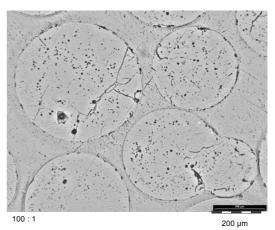
Fig. 3: Cross section of not enriched pebbles after 96 day annealing at 970 °C
