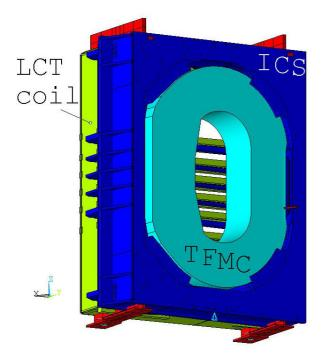
Fig. 1: Mechanical model with TFMC fixed in the Intercoil Structure and the LCT coil behind
