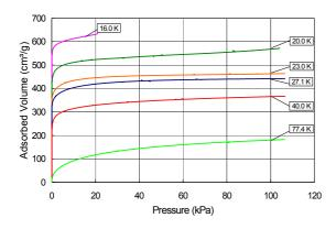
Fig. 6: Measured isotherms for hydrogen
