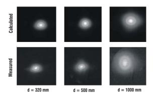
Fig. 1: Calculated and measured RF-beam pattern at different positions from the window
