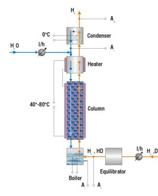
Fig. 1: Catalyst test installation
