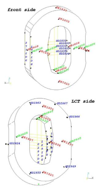
Fig. 2: Mechanical sensors on the TFMC: GDIxxx displacement devices, GRIxxx rosette strain gauges, GEIxxx uniaxial strain gauges
