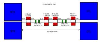
Fig. 3: Schematic layout of the MEBT for matching the beam from RFQ to DTL
