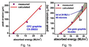
Comparison of measured total and calculated erosion by evaporation only for a CFC (a) and a IG-430U (b) sample at the e-beam facility JEBIS. Sample heating was with 100 keV electrons of peak power density of .41 GW/m<sup>2</sup>
