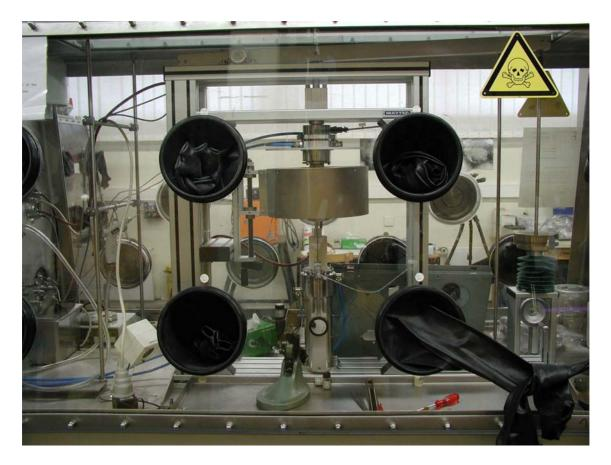
Fig. 2: High Temperature Creep Measurement on Be-Pebbles
