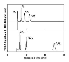
Fig. 1: TCD-A and TCD-B chromatograms of GC-2
