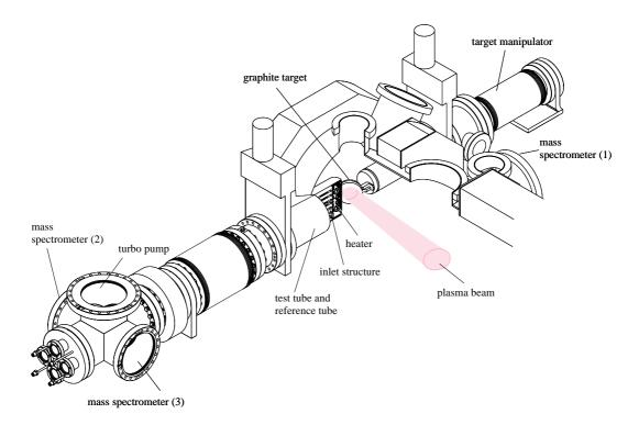
Fig. 1: Arrangement of the "hot liner" experiment. A graphite target acting as a source of hydrocarbons is fixed in the centre plasma region of PSI-2. The molecules escaping from the plasma enter the hot liner duct. The latter consists of two identical channels one with aheated head structure, the other (reference channel) is kept at room temperature
