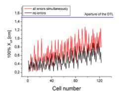
Fig. 6: 100% effective beam size in the X-Ncell-plane of the DTL with and without combined quadrupole + rf field errors
