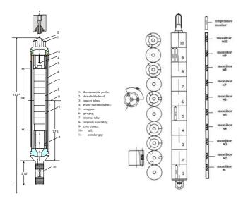
Fig. 1: Dismountable irradiation rig with a thermocouple Fig. 2: Scheme of the neutron and temperature monitors location in the suspensor
