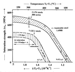
Fig. 2: Irradiation temperature dependence of saturation hardening of martensitic 7-12Cr and austenitic Cr/Ni steels by the plot  $\Delta\sigma_{i,s}$  vs.  $1/T_T=T_i$
