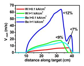
Fig. 10: Typical melt velocities for Be and W for a VDE with 30 MJ/m<sup>2</sup> and .1 sate indicated numbers describe the fraction of the melted mass which is splashed by droplets
