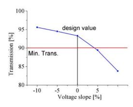
Fig. 2: Transmission as a function of the voltage-slope of the RFQ
