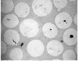
Fig. 2: Cross section of Li<sub>4</sub>SiO<sub>4</sub> pebbles (natural enrichment)
