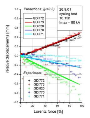
Fig. 3: Predicted and measured coil deformation of a cycling test
