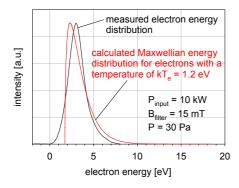
Fig. 4: Comparison of a measured and calculated electron energy distribution in order to estimate the electron temperature
