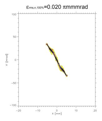
Fig. 4: Emittance determined by calculation using an CCD camera measurement
