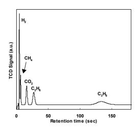
Fig. 2: µTCD chromatogram with molecular sieve capillary
