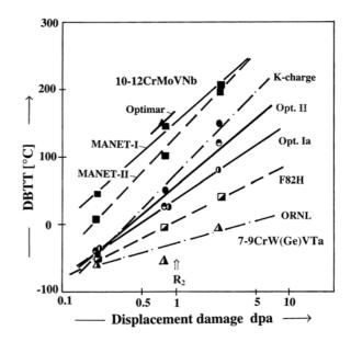
Fig. 1: Displacement damage dependence of DBTT<sub>i</sub> vs. In (dpa) for various RAFM and MANET-I,II steels at  $T_I=T_T=250^{\circ}$ C and  $\leq 15$ dpa
