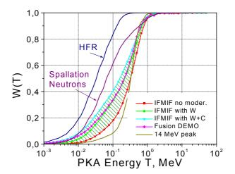
Fig. 3: W(T) function for the HCPB DEMO blanket in comparison with IFMIF (hatched area), the mixed spectrum reactor HFR and a typical spallation source
