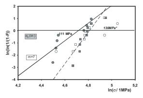
Fig. 2: Weibull analysis of the critical strength measured for disks of KU1 with machined surfaces. The data are given for neutron-irradiated specimens (full circles), unirradiated control specimens (open circles) and for comparison for irradiated / unirradiated Infrasil 301 with abraded surface (full / open squares) [4]
