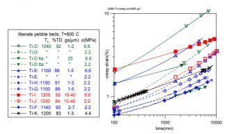
Fig. 1: Thermal creep strains of different metatitanate pebble beds
