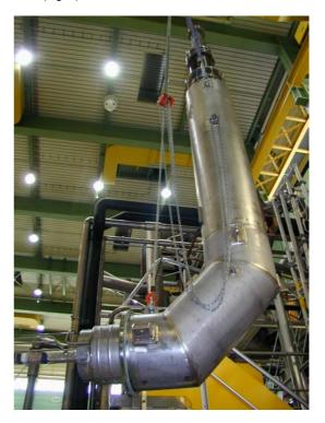
Fig. 1: One of the assembled power feedthroughs ready for installation at the flange of the TOSKA vacuum vessel
