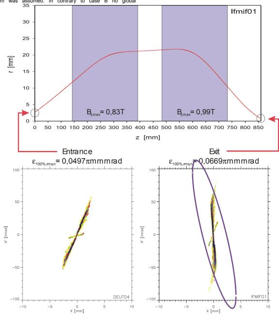
Figure 1: LINTRA simulation of the transport of a 140mA@ 100kV D<sup>+</sup> - beam for scenario A
