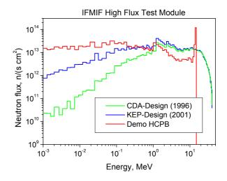
Fig. 1: Neutron spectra of IFMIF HFTM without moderator (CDA design 1996), and with W and C moderator/reflector (KEP design 2001) in comparison with the HCPB blanket of a DEMO-reactor
