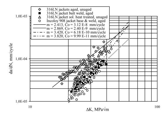
Fig. 2: FCGR of Type 316LN (Mat.: Valinox, aged and unaged) and aged Incoloy 908 (base/weld) jacket materials at 7 K (R = 0.1). The lines for m and  $C_o$  show the mean of the determined Paris constants (m is dimensionless)
