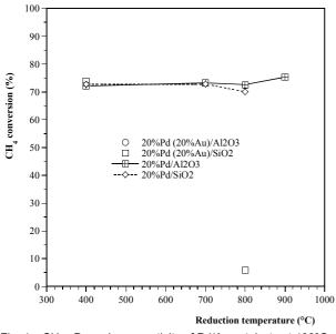
Fig. 4: CH<sub>4</sub> - D<sub>2</sub> exchange activity of Pd/Au catalysts at 400°C
