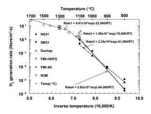
Fig. 1: Hydrogen generation from reaction of graphite with steam
