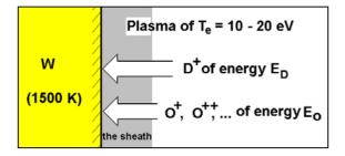
Fig. 1: The scheme of the plasma-target interaction
