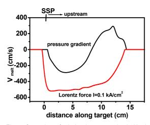
Fig. 7: Comparison of calculated average melt velocities in the tungsten melt layer for the two different forces Lorentz force with current density of 0.1 kA/cm<sup>2</sup> and gradient of plasma pressure. Close to the SSP both velocities are directed downstream
