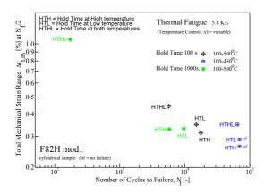
Fig. 3: Comparison of total mechanical strain range  $\Delta\epsilon_{tm}$  of thermal fatigue behaviour of F82H mod. with 100 s and 1000 s hold times
