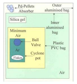
Fig. 2: Transport concept of the JET flakes
