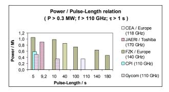
Fig. 4: Output power vs. pulse length
