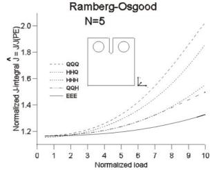
Fig. 1: Normalised J-Integral values for different size of CT specimen for Ramberg-Osgood material law with N=5
