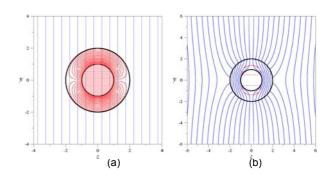
Fig. 3: Magnetic field lines and electric current distribution in a 2D MHD flow in a circular duct above the magnetic saturation field. (a) Non-ferritic wall (μ=1); (b) ferritic wall (μ=100)
