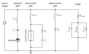
Fig. 1: Schematic discharge circuit of the ITER CSMC.  $L_{Dr}$  represents and inductor adjustable to 10 to 20  $\mu$ H in series to a parasitic inductances of 9  $\mu$ H,  $L_{paras1}$  and  $L_{paras2}$  are parasitic inductances of 1 $\mu$ H and 30  $\mu$ H, respectively
