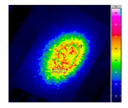
Fig. 7: Surface temperature distribution after a focused 6 ms 140 GHz gyrotron beam pulse on a 20x20 cm coated panel mock-up as target
