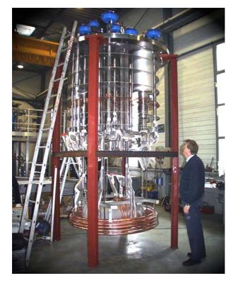
Fig. 2: Internal structures of 3000 I control cryostat
