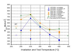
Fig. 1: Yield strength, Rp0.2, of HFR Ia specimens
