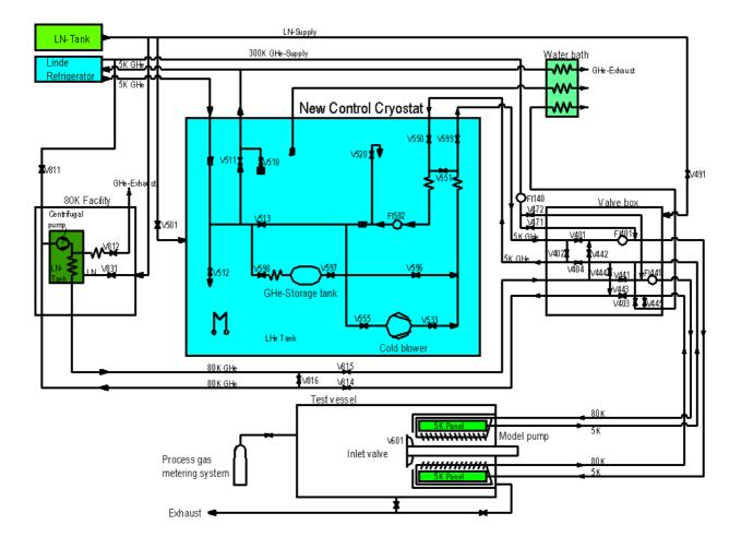
Fig.1: Simplified flow scheme of TIMO with upgraded new control cryostat
