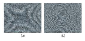
Fig. 2: Two results of measurements of a saddle like contour on an aluminium plate;  $\lambda_{synth} = 14,25 \ \mu m$ ; (a): measurement area: 4 mm x 3 mm (b): measurement area: 16 mm x 12 mm
