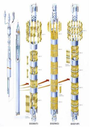
Fig. 5: Irradiation capsule with sample holders. D330: 91 tensile specimens; D329: 130 charpy specimens; D331: 160 fatigue specimens
