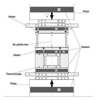
Fig. 2: Schema of the HECOP test facility. Black points indicate thermocouples. In the pebble bed each black point corresponds to two thermocouples at the same bed height
