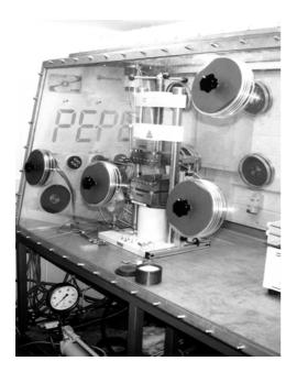
Fig 1: Glove-box with the press used in the HECOP experiments (laboratory of the firm Goraieb Versuchstechnik)
