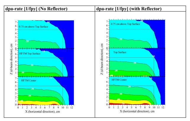
Fig. 2: Contour map with dpa/fpy iso-surface lines at three horizontal levels (*left side: without reflector; right side with reflector (10 cm Eurofer); the beam enters from the bottom*)
