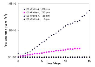
Fig. 1: <sup>4</sup>He leak rate of ferrofluidic seal for various rpm's
