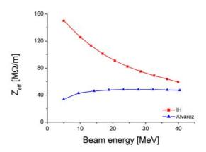
Fig. 11: Effective shunt impedances of both structures as a function of the beam energy
