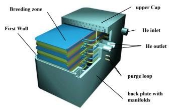
Fig. 1: Isometric view of the TBM without external manifolds and mechanical attachments to ITER
