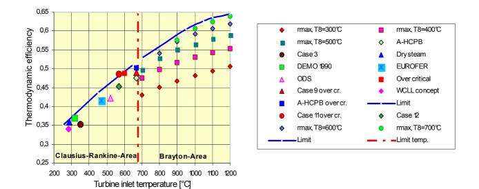
Fig. 2: Maximal attainable thermodynamic efficiency as function of the thermodynamic process
