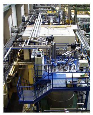
Fig. 3: TIMO facility showing new 3000 I control cryostat and cryotransfer line to cold valves box
