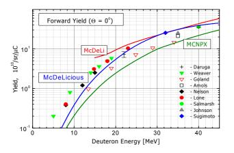
Fig. 1: Thick target d-Li forward neutron yield data.
