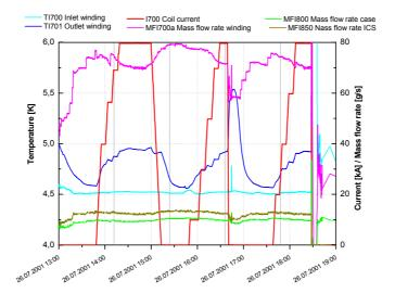
Fig. 5: Typical cryogenic operation parameters during operation with current (slow ramp down, inverter mode discharge, safety discharge)
