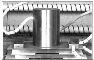
Fig. 1: Test arrangement to measure electrical resistivity. The test sample is located between the cylindrical slab and the uppermost plate
