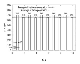
Fig. 1: Fast frequency step tuning (1s) between 136.3 GHz (TE $_{21,6}$ ) and 147.4 GHz (TE $_{24,6}$ )
