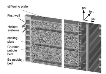
Fig. 1: Improved HCPB blanket concept, poloidal arrangement of the components: first wall, cooling plate, stiffening plate and layers of Li4SiO4 and beryllium pebble beds
