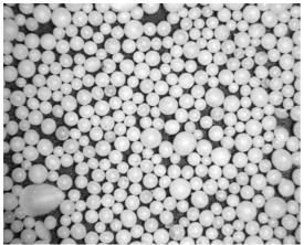
Fig. 1: Li<sub>4</sub>SiO<sub>4</sub> pebbles (natural enrichment)
