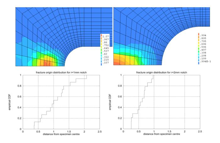
Fig. 2: Predicted (top) and observed (bottom) fracture origin location distribution
