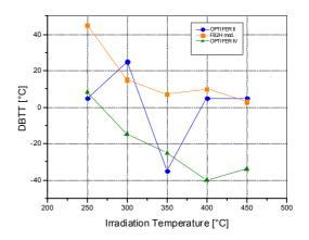
Fig. 3: DBTT of HFR la specimens vs. irradiation temperature
