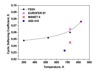
Fig. 1: The cyclic softening coefficient S for both steels under examination and similar steels cycled at the referred temperatures
