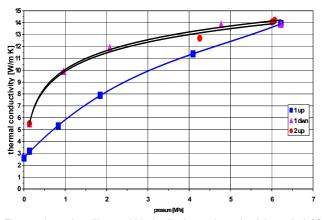
Fig. 4: 1 mm beryllium pebble bed's thermal conductivity at 250 °C bed average temperature as a function of pressure (temperature gradient in the bed about 50 °C)
