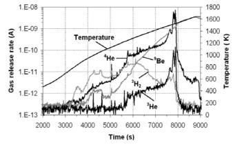
Fig. 1: He and 3H release from irradiated beryllium during a fast heating up to the melting point. Material: pebbles from the BERYLLIUM experiment. [2]
