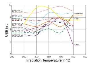
Fig. 1: Upper shelf energy vs. irradiation temperature
