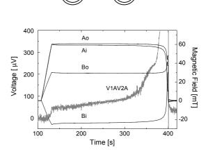
Fig. 3: Azimuthal magnetic fields measured by Hall probes close to the surfaces of Tubes A and B at a current of 10 kA indicating that the current flows mainly in Tube A. The voltage V1AV2A across Tube A suggests that the current in this Bi-2212 superconductor is close to the critical current. The nomenclature used is indicated in the scheme shown above
