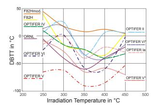
Fig. 2: DBTT vs. irradiation temperature
