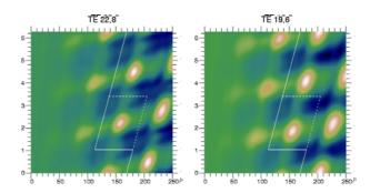
Fig. 2: RF power distribution at the unrolled waveguide wall of a Denisov-type launcher for the  $TE_{22,8}$  mode (left) and  $TE_{19,6}$  mode (right)
