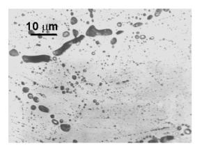
Fig. 3: Large bubbles inside the grains and at grain boundaries in irradiated beryllium after out-of-pile heating up to 1300 K: the formation of gas release pathways at grain boundaries is in progress. Material: pebbles from the BERYLLIUM experiment [3]
