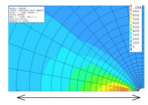
Fig. 3: Fracture origin location prediction for pre-cracked specimen (length of arrow is 40 µm)
