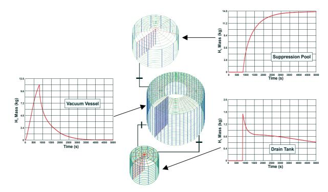
Fig.2: Results of the ITER First-wall coolant leak simulation with GASFLOW: Calculated hydrogen masses in the ITER-FEAT vessels for initial phase of accident (< 5000 s)
