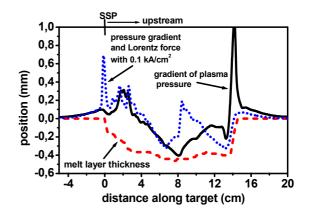
Fig. 6: Numerical results on crater depth for tungsten armour during a disruption with peak heat load of 3 GW/m<sup>2</sup> and time duration of 10 ms for the two different forces gradient of plasma pressure only and sum of plasma pressure and Lorentz force due to a current density of .1 kA/cm<sup>2</sup>.For comparison the melt layer thickness without melt motion is also shown
