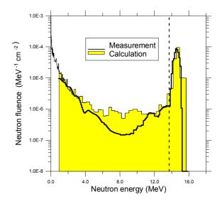
Fig. 2: Comparison of measured and calculated fast neutron fluence, normalised to one source neutron
