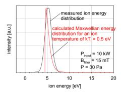
Fig. 2: Comparison of the measured and calculated ion energy distribution in order to estimate the ion temperature
