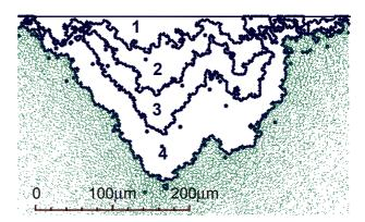
Fig. 4: Results from numerical simulation of evolution of size and depth of a single pit under pulsed cyclic surface heat loads simulating disruptions with 30 MJ/m<sup>2</sup> and duration of 10 ms
