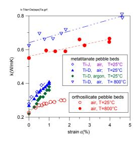
Fig. 2: Thermal conductivity of deformed orthosilicate and metatitanate pebble beds
