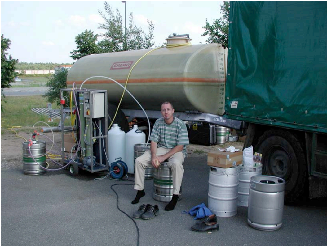
Fig. 3: Concentration of humic and fulvic acids from the groundwater by reverse osmosis (S. Geyer (photo: G. Buckau)).
