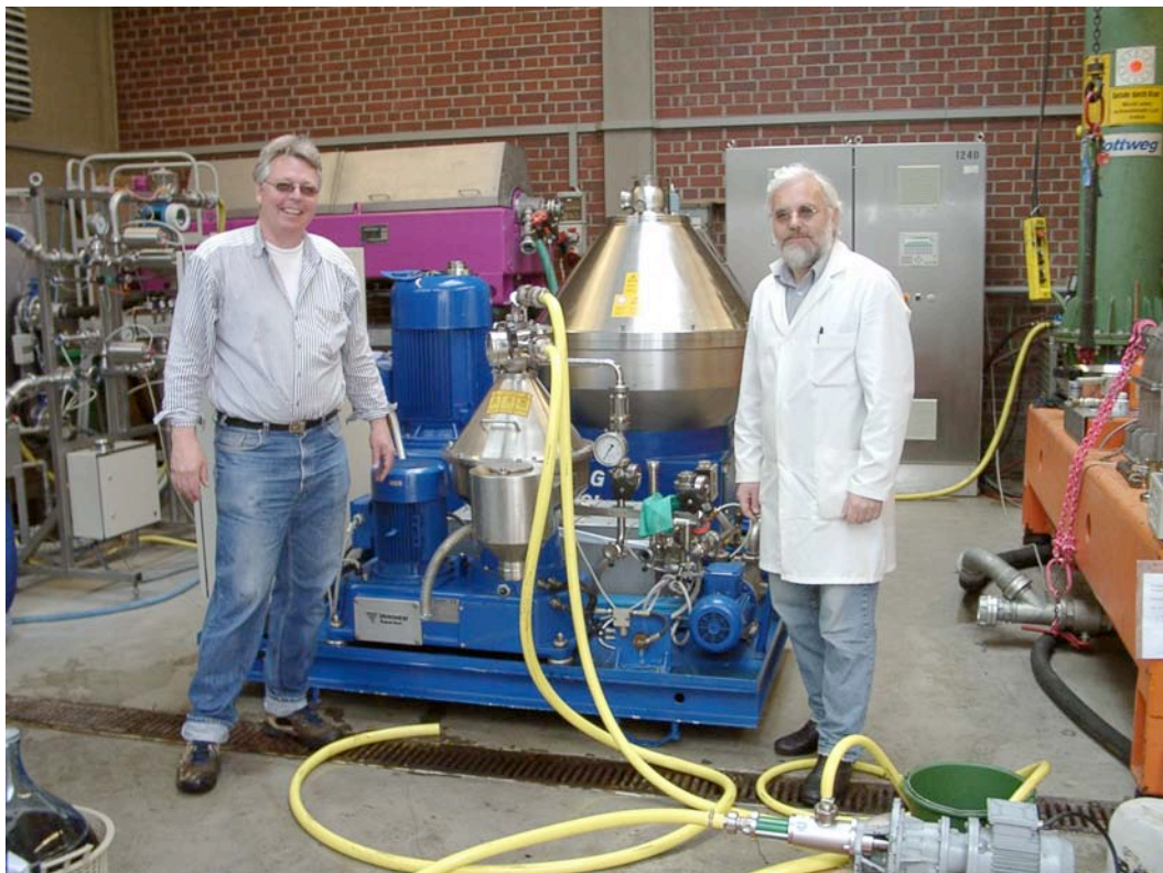
Fig. 4: View of the flow-through centrifuge (Flottweg GmbH, Vilsbiburg) together with G. Buckau and M. Wolf (photo: Flottweg GmbH).
