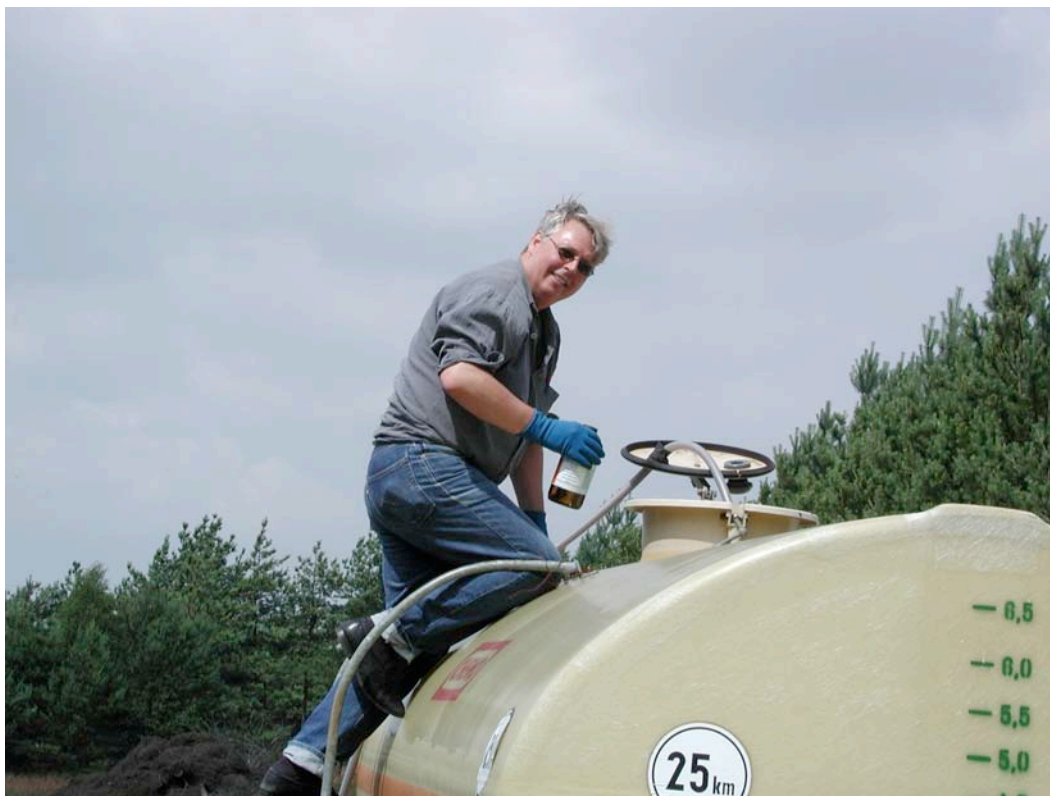
Fig. 2: Acidification of the original groundwater from borehole Gohy-573 in the tank trailer by G. Buckau (photo: S. Geyer).
