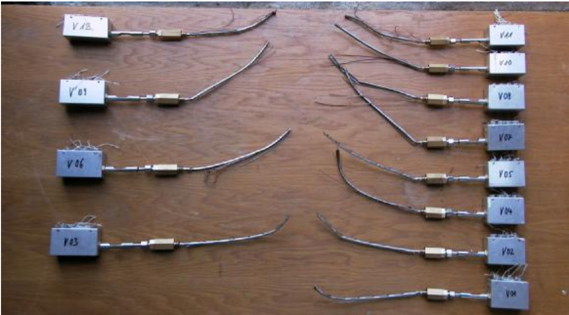
Fig. 4.2 Set of the measuring lances used in test 01, after disassembly.
