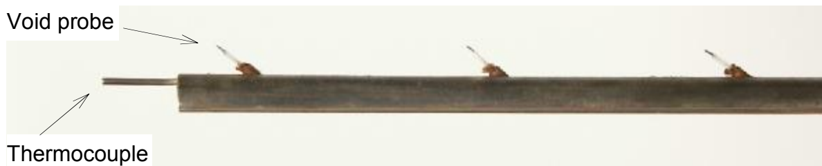
(c) Detail showing the three innermost void probes and the thermocouple. The distance between two void probes is 35 mm.
