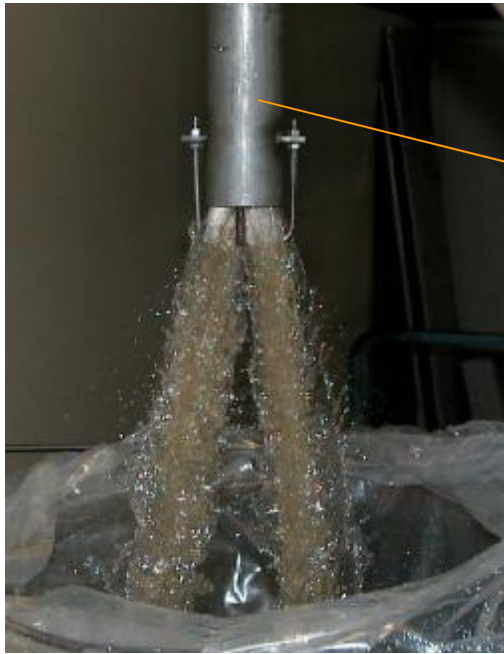
(a) Test with water showing the division of the flow.
