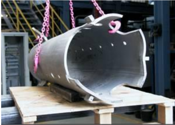
Fig. 5.5.10 ECO-05. Plastic deformations of the restriction tube caused by the steam explosion.
