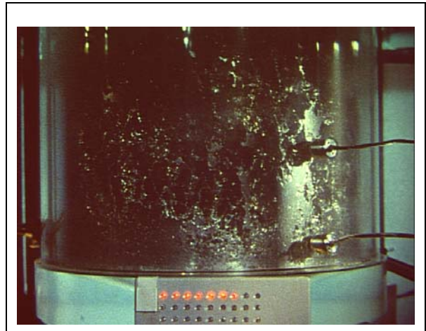
t =1000 ms: End of two-phase flow at the breach
