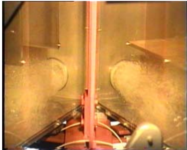
Fig. 5.172 D06 View of flow into subcompartments
