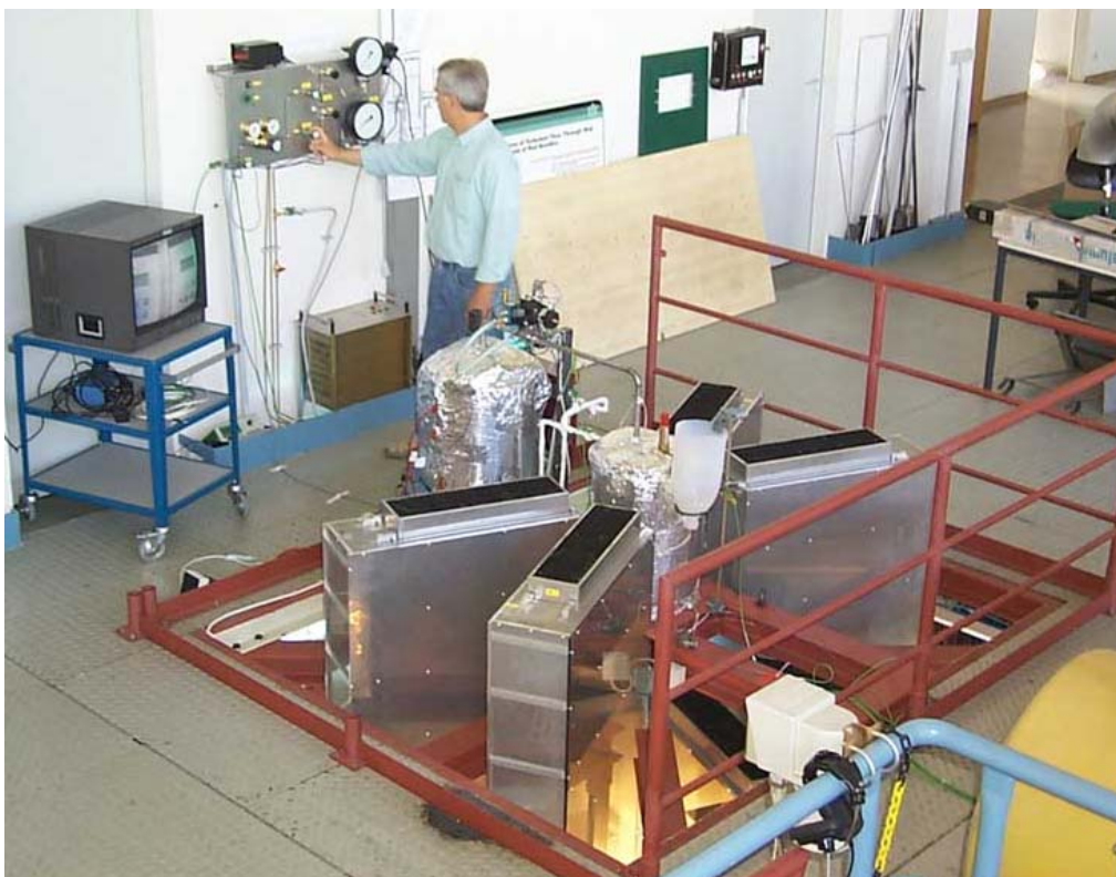
Fig. 2.5 Top view of the test facility; four large subcompartments can be seen, and the RCS-RPV pressure vessel at the center.
