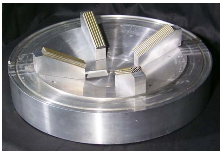
Fig. 2.12 Pedestals to stop the lower head
