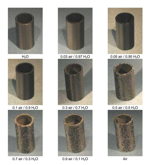
Post-test appearance of specimens oxidised 10 min at 1200 °C
