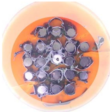
Figure 6.6: Color macro photos of cross sections at 900-1050 mm for quantification of material distribution by image analysis.
