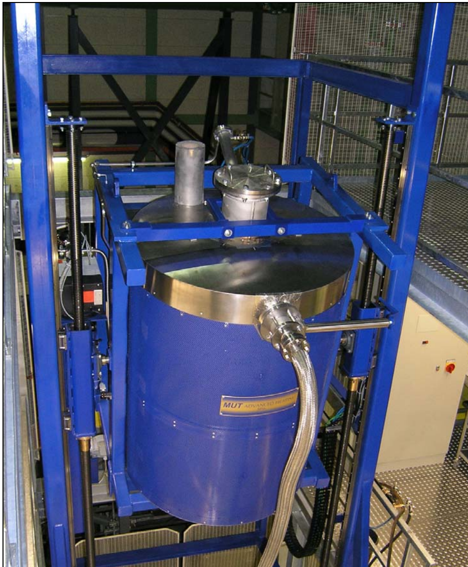
Fig. 5-7: LIVE heating furnace
