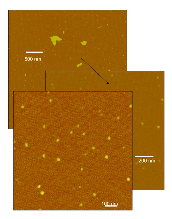
Figure 6-8: Tapping mode AFM of a dry MX80-bentonite colloidal solution sample
