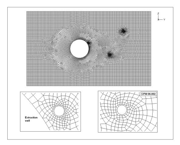
Figure 3-2: Finite element model used for calculation of tracer tests and detail of the mesh near the boreholes; dimensions of the model plane:  $20 \text{ m} \times 12 \text{ m}$ .
