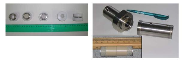
Figure 2-19: (left) Reactor of the CIEMAT setup in different assembly stages. The bentonite pellet is squeezed into a stainless-steel cylinder by two filter plates. (right) Stainless steel reactor version of the KIT-INE experimental setup. Two bentonite pellets with the PEEK spacer and the filter plates are inserted.
