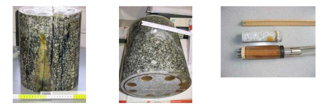
**Figure 2-30:** Preparation of the core from the Grimsel test site, Switzerland, for the transport experiments. At the surface of the core epoxy resin is used as sealing material (a). Afterwards both ends where cut plane and a borehole was drilled in the middle of the core with a 90° angle to the fracture zone (b). The packer system and drilled core from the location where the packer system is placed into the Grimsel core (c).
