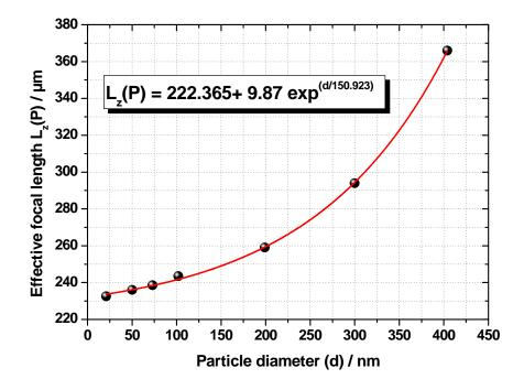
**Figure 6-9:** Effective focal length ( $L_z(P)$ ) determined by analyzing the position of 5000 single plasma events in the laser beam axis using a microscope CCD camera. Commercial polystyrene reference colloid dispersions (DUKE Scientific) with different colloid diameters (21, 50, 73, 102, 199, 300, 404 nm) are diluted with ultrapure water to the required colloid concentration.
