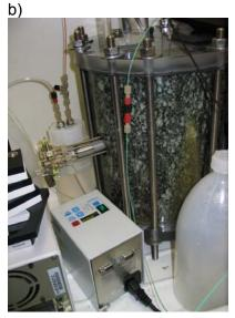
**Figure 2-31:** Core with installed packer system (a). At the end all PEEK pipes are closed with a check valve. Final experimental setup in the laboratory (b). A peristaltic pump is used to pump the water from the bottom of the core through the fracture. Another pump is injecting the tracer cocktail and GGW through the packer system. For details see text.
