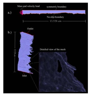
**Figure 3-8:** View of the semi-2D finite element mesh with the applied boundary and load conditions. Note that the aperture is shown as 30 times exaggera-ted for displaying reasons b.) 3D model with the inlet and outlet velocity boundary condition. The detailed view of a part of the 3D mesh shows an area inside the model where the fracture is closed.
