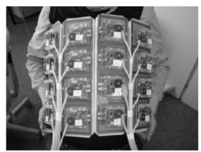
Fig. 3.12 Experimental 32 element coil array
