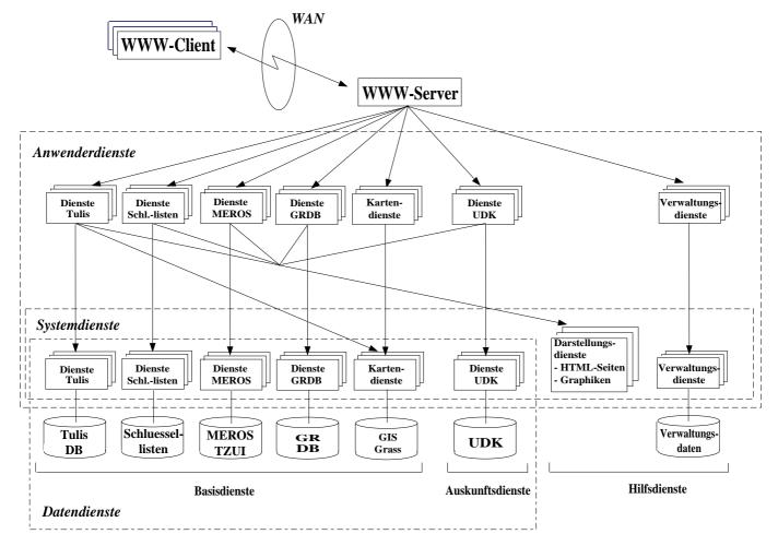
Figure 1: EIS service oriented architecture
