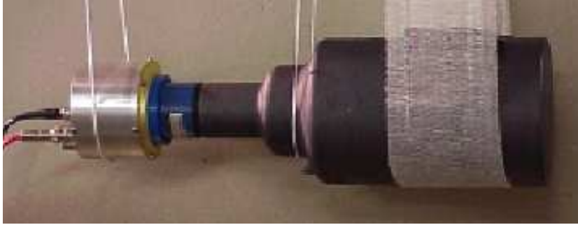
Figure 4.3: Scintillation counters with minimized neutron sensitivity employed at n_TOF.
