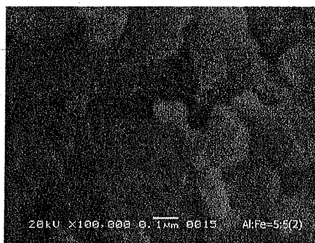
Fig. 7. SEM picture of Al : Fe=5 : 5(2) pillared clay, magnification 100,000 x
