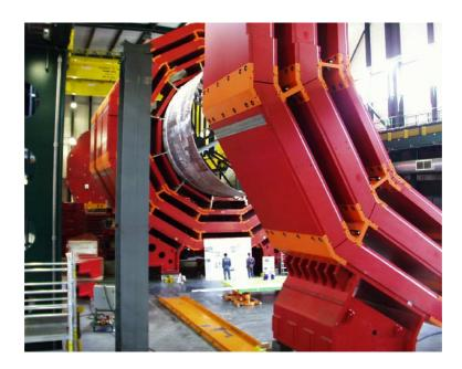
Figure 3.7: The yoke of the CMS detector at an early stage of magnet assembly. [CMS]
