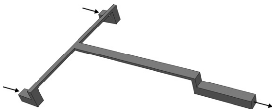
Figure 9. 3D image of the mesh geometry generated for CFD simulations with arrows indicating flow inlet and outlet boundaries.
