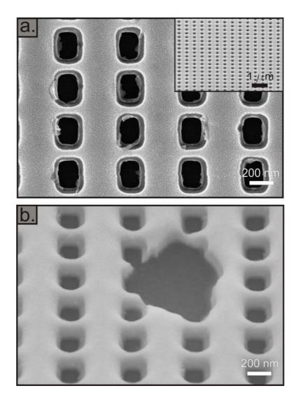
**Figure 5.19** SEM images of a meta-material with cross-double wire geometry. **a.** A top view of the meta-material structure. (Top inset) A low-magnification overview of the surface this structure. **b.** A close-up view of a break in the meta-material film showing the brighter, top and bottom gold layers, and the semi-transparent middle layer which is the photoluminescent Er doped arsenic trisulfide dielectric spacer.
