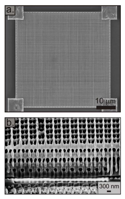
**Figure 5.9** SEM images of the woodpile structures fabricated with an Er doped  $As_2S_3$  photoresist film **a.** a low-magnification overview of the top of the woodpile structure. The in-plane rod distance, *a*, of this structure was 700 nm. **b.** Cross-section imaging of the woodpile structure showed that this structure exhibited periodicity in three-dimensions.
