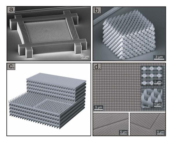
**Figure 1.4** 3D structures that were fabricated using 3D DLW in the organic photoresist SU-8. **a.** SEM image of a woodpile photonic crystal **b.** SEM image of an SP<sub>2</sub> photonic crystal **c.** Schematic depiction of a 3D-2D-3D photonic crystal hetero-structure. The line-defect present in the 2D layer was envisioned to provide lossless wave-guiding around sharp bends. **d.** SEM images of the hetero-structure depicted in **c.**
