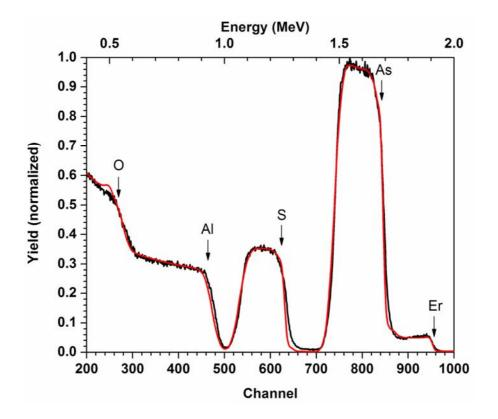
**Figure 5.3** RBS experimental spectrum (black curve) and the simulation (red curve) of an Er doped  $As_2S_3$  thin film on a sapphire substrate. The simulation agrees well with the experimental data. The stochiometry of this film is  $Er_{0.4}As_{39.4}S_{60.2}$  and represents an erbium concentration of 1.35 wt %.
