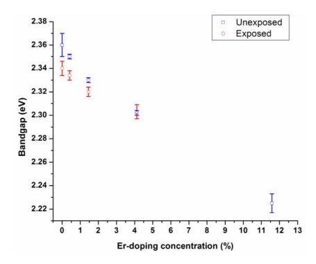
Figure 5.14 Optical band-gap of Er doped As<sub>2</sub>S<sub>3</sub> films with increasing concentration of Er.
