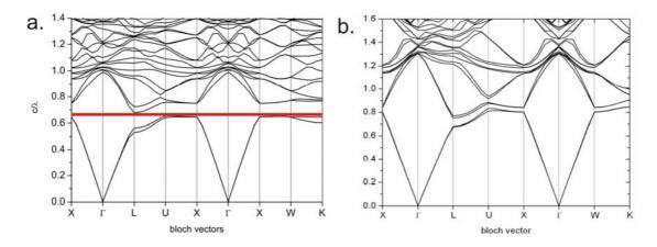
**Figure 1.2** The band structure diagram for a 3D woodpile photonic crystal made with a material with a) a dielectric constant ( $\varepsilon$ ) equal to 6.002 (or a refractive index (*n*) equal to 2.45) a full-photonic band gap is present. b) When the material that is used has a lower dielectric constant  $\varepsilon = 2.464$  (*n* = 1.57), only certain directions posses a photonic stop gap, and a full-photonic band-gap is absent.
