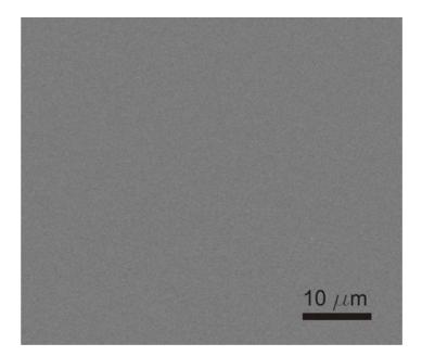
Figure 5.4 The surface of an  $As_2S_3$  photoresist film that has been doped with Er. The SEM image shows that the surface is perfectly smooth and defect free.
