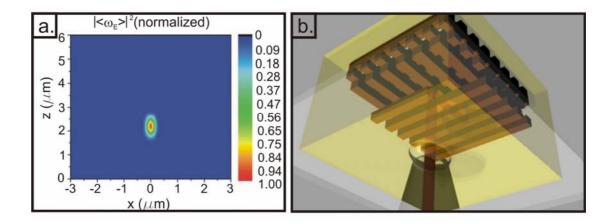
**Figure 3.1 a.** A simulation of the voxel that is generated in the conventional organic photoresist SU-8. The normalized square of the time averaged electric energy density  $|\omega_{\rm E}|^2$  exhibits iso-intensity surfaces of different intensities inside the volume of the focal spot. **b.** A graphical depiction of the 3D DLW process. Here the focus of the laser is scanned inside the photoresist material to trace out the design of the 3D structure.
