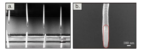
**Figure 3.12 a.** FIB cross-section of the step-ladder test structures that are routinely produced using the 3D DLW with the shaded-ring filter in-place. **b.** the individual bars have a lateral resolution of 180 nm and has an aspect ratio as expected from the simulation of the normalized square of the time averaged electric energy density  $|\omega_{\rm E}|^2$  inside As<sub>2</sub>S<sub>3</sub>.(see Figure 3.11)
