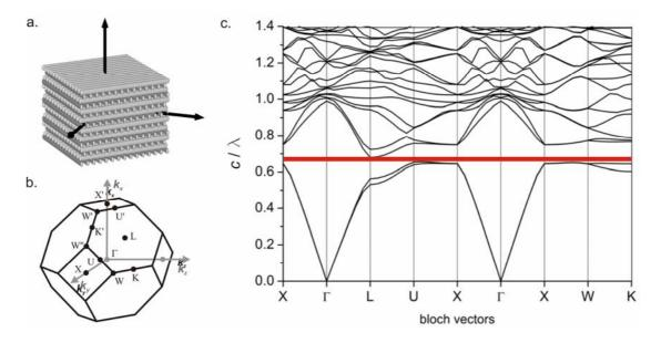
Figure 1.1 a. A woodpile photonic crystal with FCC symmetry. b. The first Brillouin zone of such an FCC structure. c. The band-structure calculation of such a woodpile photonic crystal structure ( $\varepsilon = 6.0025$ ) exhibiting a full-photonic band gap.
