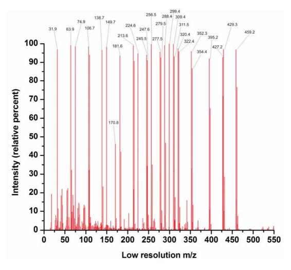
**Figure 2.3** A mass spectrum of the  $As_2S_3$  precursor as obtained from the MS2 mass spectrometer. The masses of the important fragments are assigned. A discussion of the fragments is provided in the text and in Figure 2.4.
