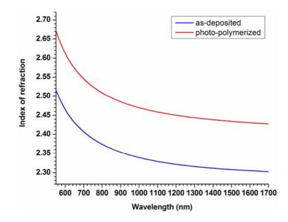
**Figure 2.12** The refractive index dispersion curve of the  $As_2S_3$  photoresist in the as-deposited form (blue curve) and the photo-polymerized form (red-curve). The refractive index exhibits an increase upon photo-polymerization from 2.31 to a value of 2.45 at the wavelength of 1550 nm. This represents a 5.5% increase in the refractive index.
