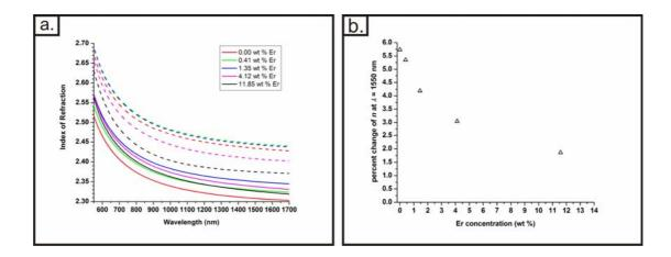
**Figure 5.15 a.** The refractive index dispersion curves for films doped with increasing concentrations of Er. **b.** The percentage change in the refractive index between an as-deposited films and a photo-exposed film, at 1550 nm wavelength, as a function of Er concentration.
