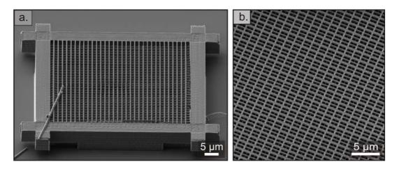
**Figure 3.5** SEM images of  $As_2S_3$  woodpile structures that have been etched out using a wet-etchant containing the diisopentylamine molecule. **a.** The structures are perfectly straight and there are no shrinkage effects that are commonly experienced with structures that are produced using organic photoresist such as SU-8. **b.** A close-up image of the surface of the structure reveals that the rods are smooth and exhibit excellent in-plane periodicity.
