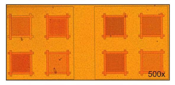
**Figure 3.4** An optical microscope image of the structures that have been photo-patterned into the photoresist material using the 3D DLW process. The structures are directly visible after the 3D DLW process due to the increase in the refractive index that is experienced upon photo-polymerization.
