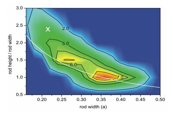
**Figure 3.9** Gap-width map in percent of the mid-gap frequency for the independently adjustable parameters. The white cross marks the position corresponding to the sample measured in (a). Refining the parameters can yield a gap width of up to 8.8%, for a rod aspect ratio of almost 1.0. Structures below the solid white line are not mechanically stable.
