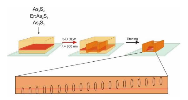
**Figure 5.11** A schematic of the steps leading to the fabrication of a step-ladder structure which is used to demonstrate spatially selective photoluminescence.
