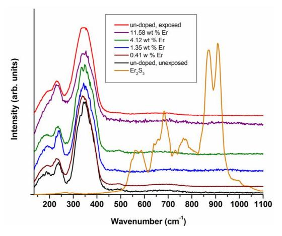
**Figure 5.16** Raman spectrum of Er doped  $As_2S_3$  films that contain different Er concentrations. The individual spectra are vertically staggered for clear representation of the data. A Raman spectrum of polycrystalline  $\delta$ -Er<sub>2</sub>S<sub>3</sub> is also overlaid here to show that the Er has not agglomerated into small clusters.
