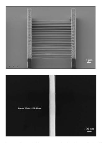
**Figure 4.6** (Top) SEM image of a test-ladder structure that has been etched with an etchant solution containing the highly-selective amine *N*-(4-methoxybenzyl)-(pyren-1-yl)amine. Such a test-ladder demonstrates the ability to simulate 3D structures because it contains freely suspended nano-rods which can serve to represent a true 3D feature. (Bottom) An SEM image of the highest lateral line-resolution that can be achieved using the step-ladder test structure.
