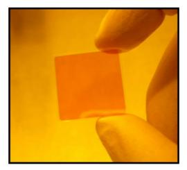
Figure 2.6 A typical as-deposited  $As_2S_3$  photoresist thin film on a silica glass substrate. The film is orange in color and optically, clear and transparent.
