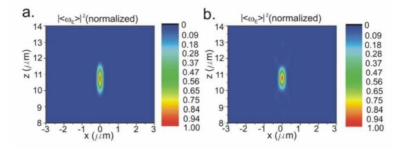
**Figure 3.11** A comparison of the normalized square of the time averaged electric energy density  $|\omega_E|^2$  that is 10.8 µm into the depth (z) of an As<sub>2</sub>S<sub>3</sub> photoresist. **a.** the  $|\omega_E|^2$  without shaded- ring filter and **b.** the  $|\omega_E|^2$  with the shaded ring filter. Once can see that elongation of the voxel can be improved from 6:1 to 4:1 via the introduction of the shaded ring filter.
