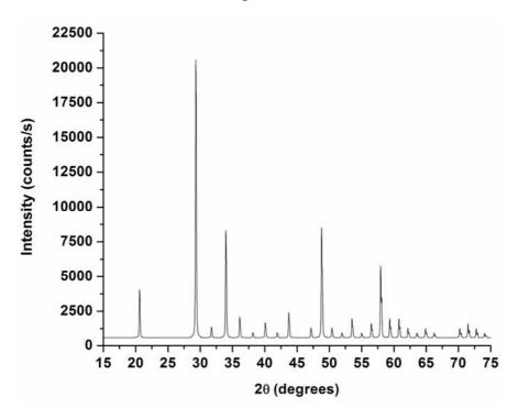
b. Er<sub>2</sub>O<sub>3</sub> Spectrum From the JCPDS-ICDD Database (PDF # 08-0050).
