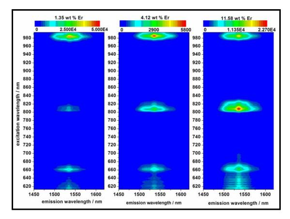
Figure 5.18 PLE spectra of 3 Er:As<sub>2</sub>S<sub>3</sub> films doped with progressively higher Er concentrations.
