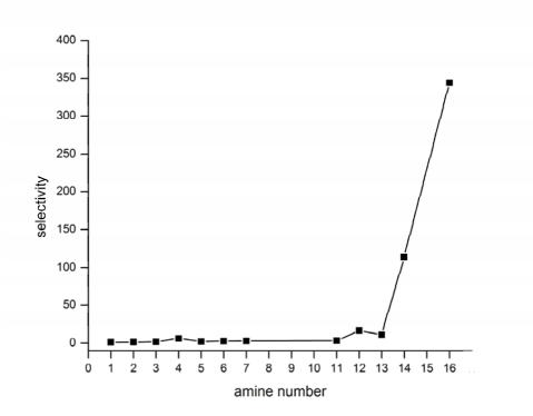
**Figure 4.5** A plot showing the selectivity  $\gamma$  of the different amine molecules synthesized in this study. It can be clearly seen in this graph, that there is a dramatic increase in the selectivity as the steric size of the amine increases. Amines 8 to 10 and 15 are not plotted on this graph as these amines did not show any showed no reaction when used as the active species in the etchant.
