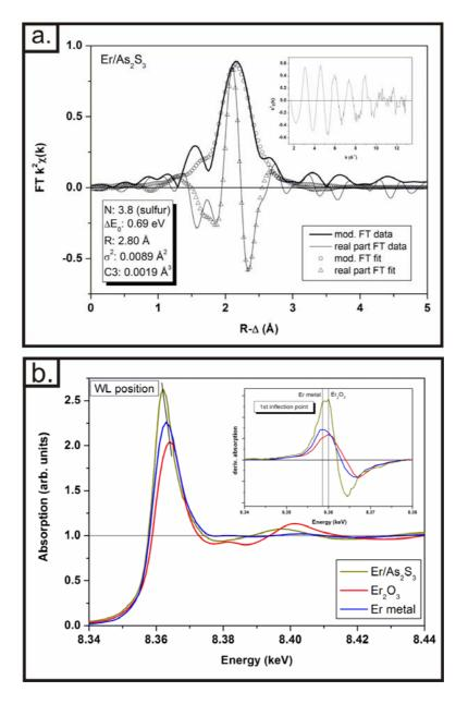
**Figure 5.17** Synchrotron data collected from a 1.35 wt % Er doped  $As_2S_3$  thin film and 2 reference samples of pure Er metal and  $Er_2O_3$  powder. **a.** The spectrum of the EXAFS measurement on the 1.35 wt % Er doped  $As_2S_3$  thin film. **b.** The spectrum of the XANES measurement of all 3 samples.
