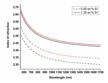
**Figure 5.6** The refractive index dispersion curve that is obtained from the thin film ellipsometery of an un-doped sample (black curve) and a 1.35 wt % Er doped sample (red curve), in both the as-deposited and photo-polymerized states.
