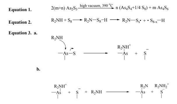
**Figure 4.2.** The chemical reactions that have been proposed to occur during the different stages of the etching process. Equation 1 shows the species that are generated during the thermal evaporation of the precursor material. Equation 2 shows the initial steps of a multi-step reaction where an amine catalyzes the ring-opening scission of S-S bonds in the  $S_8$  molecules. Equations 3a and b show the two reaction steps that take place on the surface of the exposed areas.
