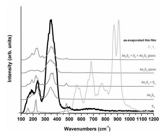
**Figure 2.8** A comparison of the Raman spectrum of the as-deposited film and the pure compounds and their mixtures. Once can easily distinguish the contributions of each compound in the as-deposited thin film. The numerical assignments of the bands are provided in the text and in Figure 2.8.
