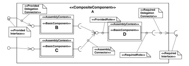
Figure 3.13: Example Instances: Composite Component
