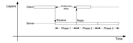
Figure 6.11: Phases in LQNs Illustration [FMW<sup>+</sup>07]
