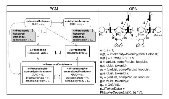
Figure 4.20: Mapping PCM2QPN: InternalAction
