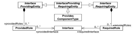
Figure 3.8: Component, Role, Interface (meta-model)
