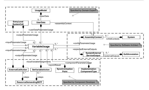
Figure 4.4: Classes containing Variable Usage (meta-model)
