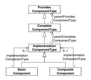
Figure 3.9: Component Types (meta-model)
