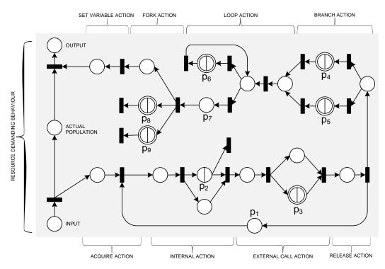
Figure 4.26: QPNs resulting from mapping a PCM RDSEFF (Example)
