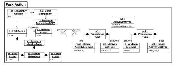
Figure 6.23: Mapping PCM2LQN: ForkAction
