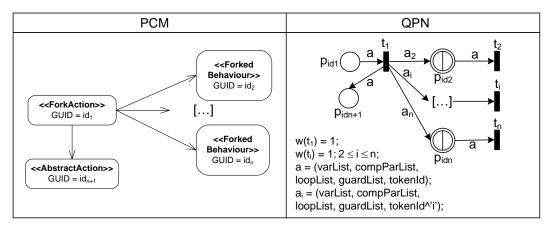
Figure 4.23: Mapping PCM2QPN: Fork Action
