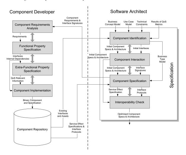
Figure 3.2: Component-Based Development Process: Specification Workflow (Detailed View)
