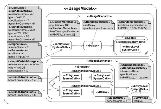
Figure 4.7: Usage Model (Example)
