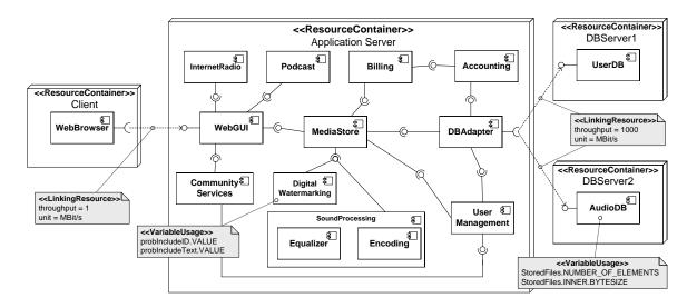
Figure 7.2: Media Store, Static View and Deployment
