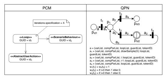
Figure 4.16: Mapping PCM2QPN: Loop
