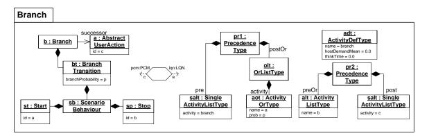
Figure 6.19: Mapping PCM2LQN: Branch
