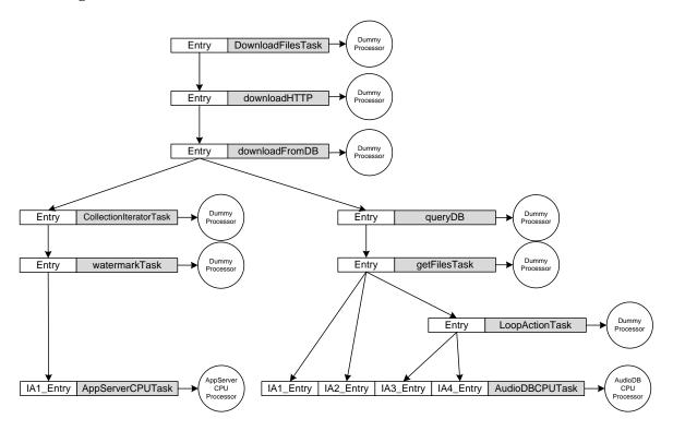
Figure 7.10: Layered Queueing Network for the MediaStore
