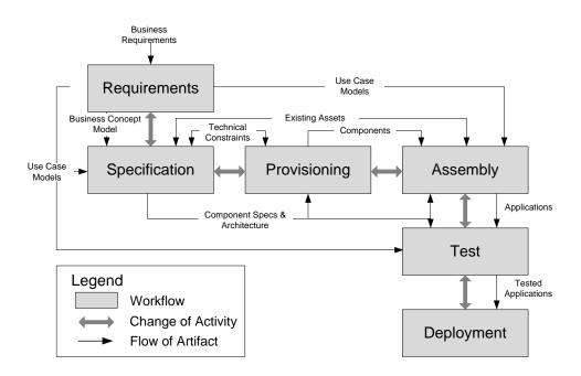
Figure 2.2: Component-Based Development Process [CD01]
