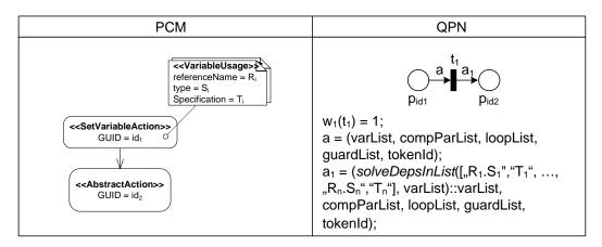
Figure 4.22: Mapping PCM2QPN: SetVariableAction
