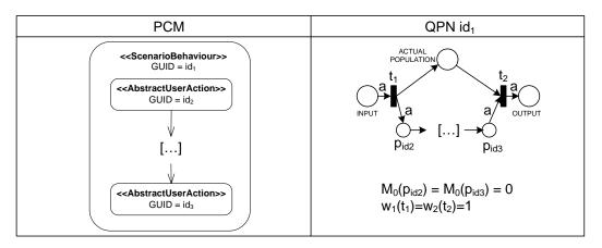
Figure 4.14: Mapping PCM2QPN: ScenarioBehaviour
