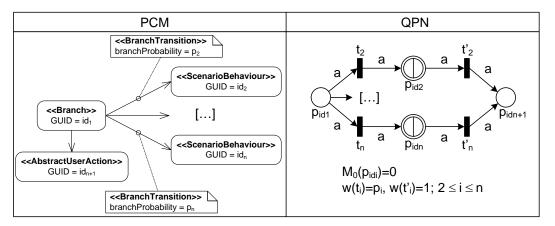
Figure 4.15: Mapping PCM2QPN: Branch
