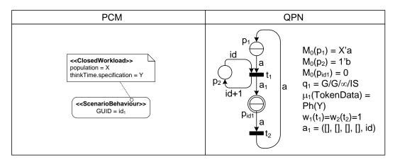
Figure 4.12: Mapping PCM2QPN: Closed Workload
