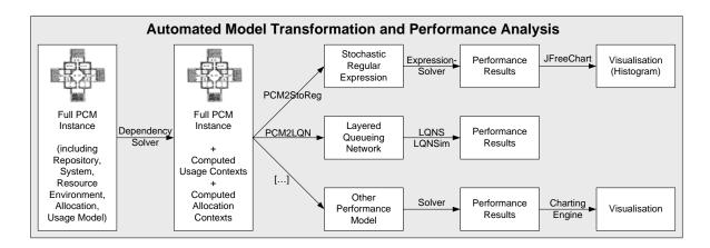
Figure 6.1: Model Transformation Process Model
