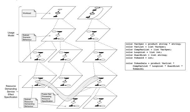
Figure 4.11: HQPN Instance as a Result of a Mapping from a PCM Instance
