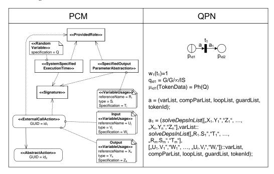
Figure 4.21: Mapping PCM2QPN: ExternalCallAction for system external service
