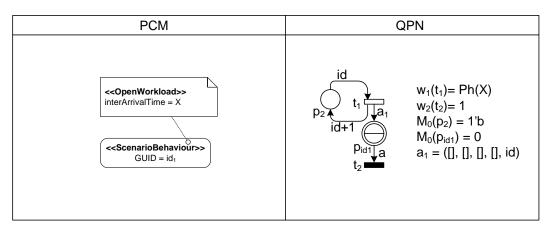
Figure 4.13: Mapping PCM2QPN: Open Workload
