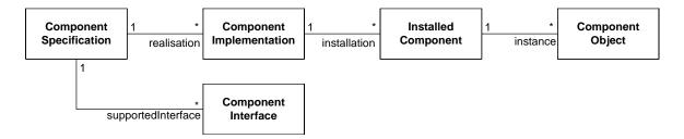
Figure 2.1: Forms of Software Components [CD01]
