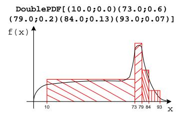
Figure 3.20: Example: pdf-discretisation with variable intervals
