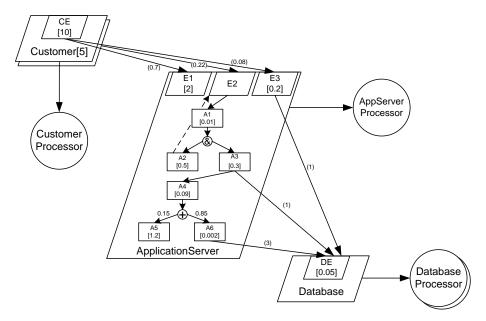
Figure 6.12: Simple LQN Example with 3 Layers
