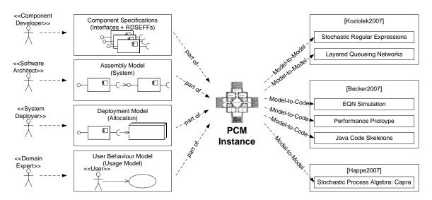
Figure 3.4: Palladio Component Model: Parts and Analysis Models
