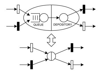
Figure B.1: Queueing Place and its Shorthand Notation [Kou06]
