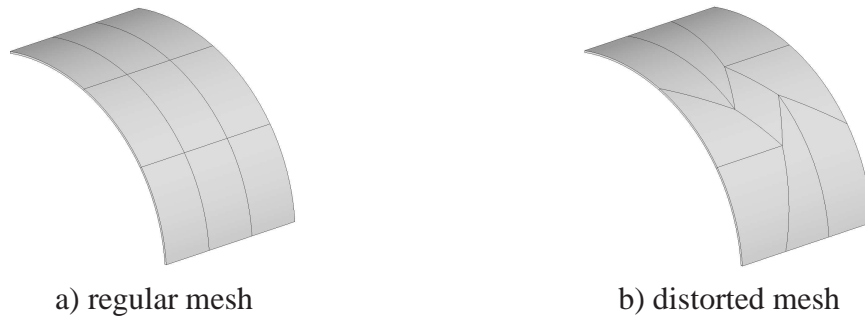
Fig. 15 Cylindrical cantilever shell: finite element meshes with 9 high order solid elements
