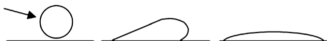
Fig. 2 Schematic drawing in lateral perspective of drop spreading on the target liquid surface
