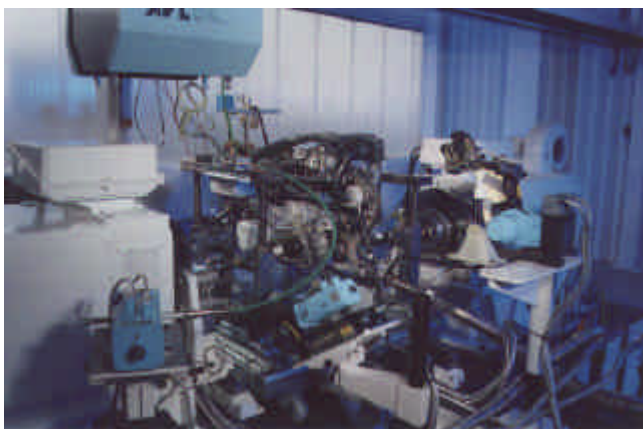
Fig. 2 AVL powertrain test bed with combustion engine and manual gearbox in Front-Wheel-Drive configuration
