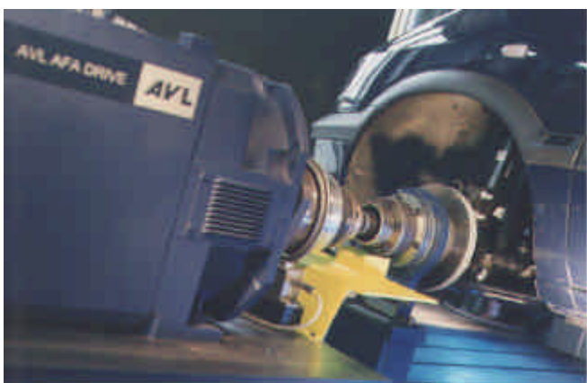
Fig. 4 Multiconfiguration Test Bed for Fuel Cell Drives – Complete Vehicle Setup
