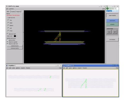
Figure 7.6: An event in the TRD event display. The incoming particle creates a secondary  $\delta$ -electron on top of the detector. Due to its low energy the trajectory is not a straight line and is rejected by the track finder algorithm.
