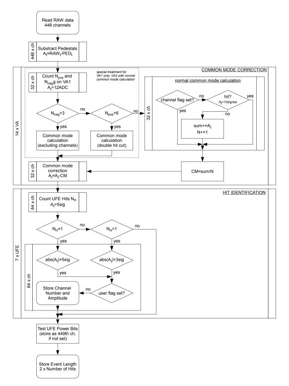
Figure 6.20: Simplified flowchart of the data reduction routine of the UDR2. Before the hit identification routine the raw data values retrieved from the front end electronics are pedestal subtracted and a common noise correction for each VA chip is applied.
