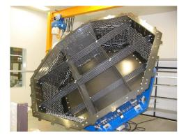
Figure 3.21: The TRD carbon fiber support structure. The twelve layers of straw tube modules in the middle (1) are rotated by  $90^{\circ}$ with respect to the four layers on top (2) and four layers on bottom.
