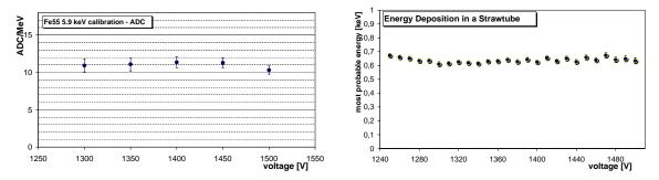
Figure 4.44: Voltage dependence of the calibration factor. The calibration factor KF should be independent of the gas gain, which is perfectly confirmed within the errors.
