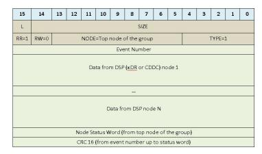
Figure 6.28: AMS sub-block format. During normal operation the only sub-block is the JINJ sub-block containing the JINF and SDR board data.
