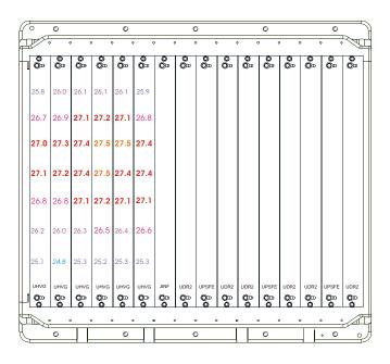
Figure 5.23: U-Crate temperature profile read out by the MHV100 sensors of the UHVG boards.
