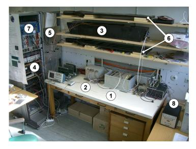
Figure 4.38: Setup of the Karlsruhe cosmics test stand. The qualification model of the U-Crate (1) and the UPD box (2) read out a TRD chamber (3), which is supplied by a ground support gas system (5). The entire DAQ system is powered by a 28V commercial power supply (4). The trigger is generated by NIM-logics modules (7) by coincidence of scintillator modules (6) placed on top and on bottom of the chamber. A DAQ computer (8) reads out and controls the U-Crate via the AMSWire protocol.
