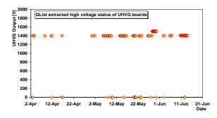
Figure 7.28: Housekeeping data steadily collected by JMDC from the U-Crate QList during the second half of the pre-integration phase. The high voltage for the TRD was kept stable at 1400 volts except for a short running period in order to compensate a lower gas gain with high gas pressure during a TRD gas system test.
