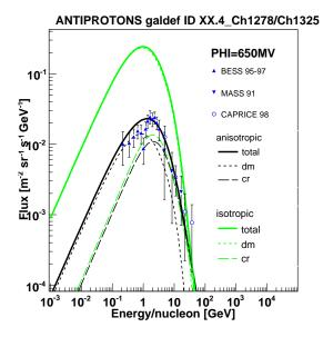
Figure 2.10: Antiproton flux in isotropic and anisotropic propagation models. In isotropic models the signal from dark matter annihilation extracted from gamma ray observation clearly dominates the cosmic ray flux and is inconsistent with the data. In anisotropic models the flux is much reduced by blowing away dark matter signal originating in the halo of the galaxy.
