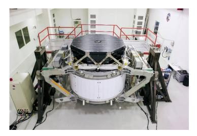
Figure 6.1: AMS-02 at CERN in December 2007. The entire detector is read out by a flexible network of independently operating slave computers and one out of four main DAQ computers of AMS-02 as the master.
