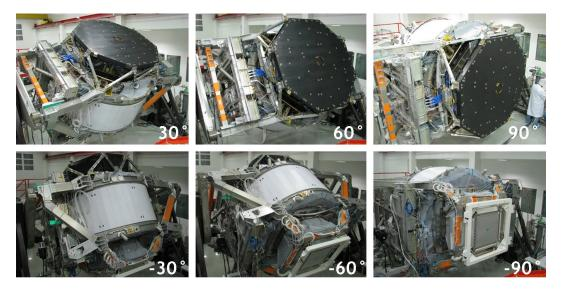
Figure 7.26: AMS-02 rotation test at the end of the pre-integration phase. The main aspect was the test of the mechanical stability mainly of the tracker. The position of the ladders was monitored throughout the test by the tracker alignment system (TAS).
