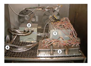
Figure 4.24: QM2 ESS climatic chamber test setup. The U-Crate (1) and the UPD box (2) are interconnected by qualification model cables. Front end simulator (UFS) boxes (3) are connected to the UDR2 boards of the U-Crate. The chamber wall allows to connect 28V power to the UPD box and AMSWire cables (4) to the JINF board of the U-Crate.
