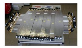
Figure 3.12: One out of two ToF planes. Each plane consist of two layers of crossed scintillator panels. Photomultiplier tubes are attached to the ends of the panels.
