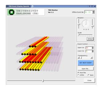
Figure 4.40: A snapshot of the event monitor with  ${}^{55}Fe$  radioactive source. The opening angle of the source is visible in the adapted version of the monitor averaging the amplitudes over time.
