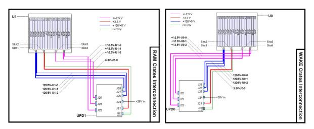
Figure 5.12: Interconnecting cables between the UPD box and the U-Crate. The 14 cables of different length were produced at CSIST.
