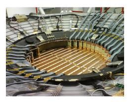
Figure 3.5: The AMS-02 tracker mounted in the center of the vacuum case. The picture was taken during the pre-assembly of AMS-02.
