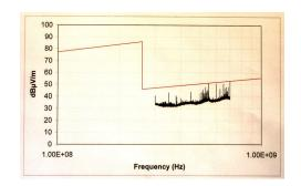
Figure 4.33: The emitted spectrum during the operation of the U-Crate. Clearly visible are the peaks, which touch the limit of allowed radiation at a few hundred MHz.
