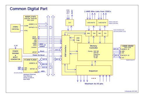
Figure 4.11: Scheme of the common digital part (CDP) of xDR nodes in AMS-02. The central part is the digital signal processor (DSP) with an internal memory of 2x64 kByte. The operating programs are stored in a flash memory. The DSP clocks an Actel FPGA, which controls the transmissions on the AMSWire links. A sequencer part of the FPGA retrieves the digitized data from the front end electronics and stores it to a SRAM memory for the DSP's disposal.
