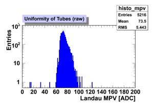
Figure 7.45: Mapping of the MPV obtained by a fit of the Landau function to the amplitude distribution of the on-track energy deposition in a tube.
