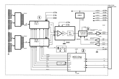
Figure 4.7: UFE board schematics. The two VA32 chips (1) take over the pre-amplifying, shaping and multiplexing of 32 channels. The hybrid control circuit HCC (2) controls the readout sequence and the switching of the VA32 chips. The analog signals are digitized by an AD7476 ADC (3).
