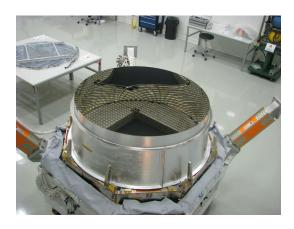
Figure 3.10: The RICH assembled and mounted on top of the ECAL to the lower unique support structure (USS).
