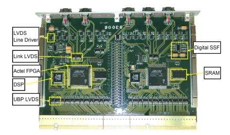
Figure 4.9: Picture of the JINF board. Four AMSWire links are present to the higher DAQ system on the front panel and one link for the trigger. The JINF connects to all nodes in the U-Crate by AMSWire links on the backplane as well as by LeCroy buses to slow control electronics.
