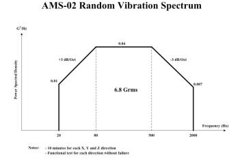
Figure 4.26: The vibration spectrum of the ESS. Unlike the thermal stress, which will be performed again with the assembled AMS-02 instrument in a space simulator, the vibration test of the parts is the last test of mechanical stresses before the launch in the Space Shuttle.
