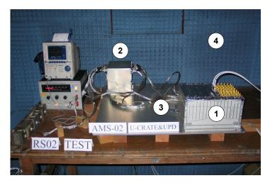
Figure 4.29: The EMC test setup at CSIST facilities. The U-Crate (1) and the UPD box (2) are interconnected by cables shielded with a metal mash (3). An aluminum plate simulates the radiator, on which the crates will be mounted in AMS-02. The EMC test chamber is equipped with walls absorbing the electromagnetic radiation (4).
