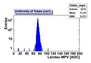
Figure 7.47: Mapping of the MPV obtained by a fit of the Landau function to the amplitude distribution of the on track energy deposition of a tube after inter-calibration of the modules.
