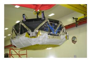
Figure 3.22: The assembled TRD lifted by a crane. The carbon fiber structure is stabilized by the M-structure machined from solid Aluminum.
