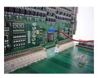
Figure 5.2: UDR2 test backplane solid state fuse test. Test points on the UDR2 and UPSFE boards allow to insert a load into the digital circuit in order to test the correct switching of the solid state fuses on the boards.
