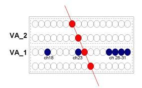
Figure 7.19: Affected channels of the M-type UFE board. Only channels of one out of four modules of a chamber show the pedestal shift at fast consecutive readings, which allows a track reconstruction even in the case a particle hits such a tube losing the amplitude information.
