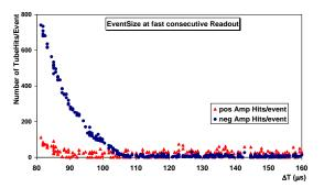
Figure 7.20: TRD event size at fast consecutive triggers. Below time differences of about  $110 \,\mu s$  the number of channels with a negative amplitude due to the reset signal crosstalk increases strongly.
