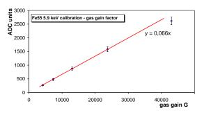
Figure 4.42: Extracted signal amplitude for the  ${}^{55}Fe$  source in ADC units. The amplitude is a function of the high voltage according to the Diethorn formula.
