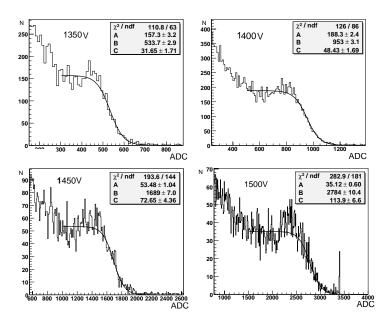
Figure 4.41: Histogram of tube hits with a  ${}^{55}Fe$  gamma source. Due to the uncorrelated readout the tube is read out in the maximum of the collected charge by incident only. The Gaussian becomes a Fermi-like distribution. Nevertheless the maximum value is fixed by the energy of the  ${}^{55}Fe$  photons at a given high voltage and can be extracted for an energy calibration.
