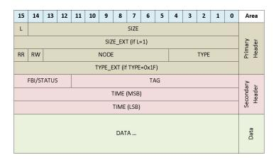
Figure 6.27: Format of an AMS data block. [11]
