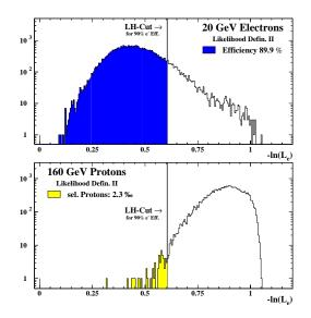
Figure 3.32: The likelihood-cut definition. The cut is defined such that 90% of electrons are identified correctly. The proton rejection factor is the inverted number of wrongly identified protons and is for all energies well above 100.
