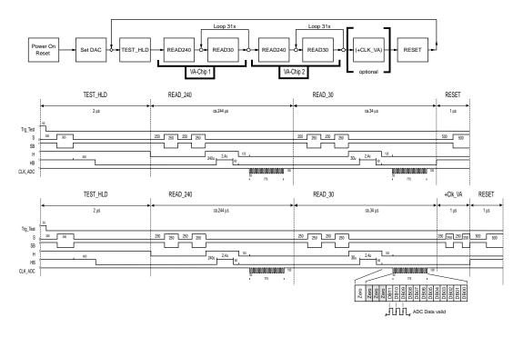
Figure 6.23: UFE DAC calibration sequence
