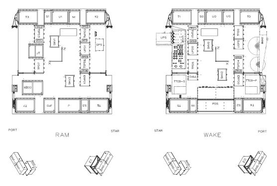
Figure 3.34: Mapping of the electronics crates mounted to the two main heat radiators.
