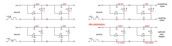
Figure 4.17: Simplified Cockcroft-Walton high voltage chain. The working principle is explained in the text.
