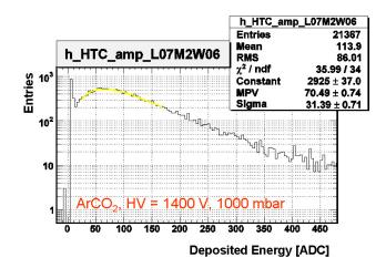
Figure 7.44: *Histogram of on track amplitudes of a singe tube.* As expected negative amplitudes cannot be found on track of a particle.
