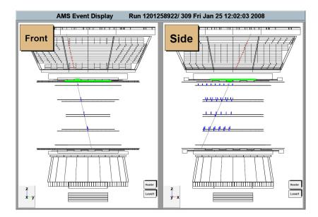
Figure 8.1: Cosmic ray track recorded with AMS-02 during the pre-integration phase in January 2008.
