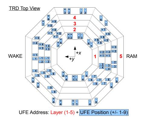
Figure 6.29: Map of the mounting position of the UFE boards on the TRD. The UFE address is used to identify the chamber, which is connected to a UDR2 front end link in table 6.30. [49]
