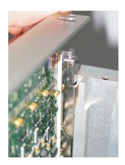
Figure 5.11: Wedge-locks present on all boards of the U-Crate.
