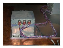
Figure 4.31: EMC test cable preparation. The cables interconnecting the U-Crate and the UPD box are not shielded in contrast to first test in Taiwan.
