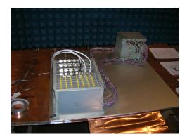
Figure 4.30: The EMC test setup at Terni facilities. The UPD box and the U-Crate were mounted to an Aluminum plate to ensure a realistic grounding. With the applied modifications of the hardware the test was passed successfully.
