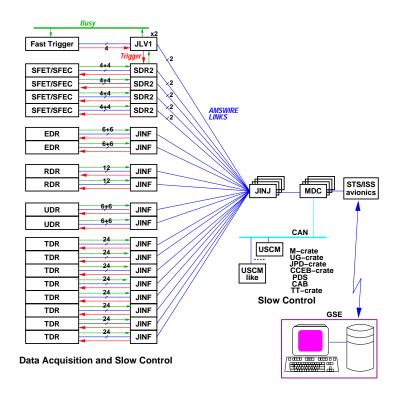
Figure 6.2: AMS-02 data acquisition architecture.
