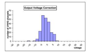
Figure 5.21: Distribution of UHVG channel calibration correction at 1000V. The value is calculated from the difference of the output voltage to the mean DAC setting, which corresponds to 1000V.
