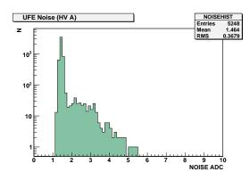
Figure 7.10: The distribution of the TRD channel noise with UHVG half A active. About one sixteenth of the channels shows a higher noise, which cannot be observed with UHVG half B active.
