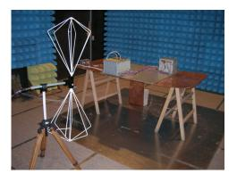
Figure 4.32: Emitted electromagnetic radiation test. The antenna records the emitted radiation during the operation of the U-Crate.
