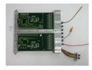
The board with soldered cables and the connectors mounted to the Iframe. PCB with assembled parts and conformal coating.
