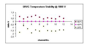
Figure 5.22: UHVG channel temperature dependence of the output voltage. For this random sample of channels the output voltage shows a variation of about 2V at  $70^{\circ}C$  temperature variation, which is well within the requirement.
