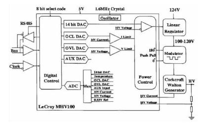
Figure 4.16: Schematic of the UHVG high voltage control circuit. The custom made MHV100 chip takes over the control and monitoring and is addressed via the LeCroy bus. The modulated peak voltage at the input of the high voltage cascade is regulated such that the feed back voltage from a divider circuit and the 14-bit DAC generated voltage match.
