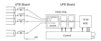
Figure 4.5: TRD front end electronics scheme. The VA32 chips, which switch the signals from the UTE capacitors to the ADC, and the ADC chips are controlled by a hardware control chip (HCC) on the board. The clock is given by the UDR2 board sequencer.
