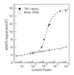
Figure 3.28: The energy deposition from ionization and transition radiation for high Lorentz factors. At high energies the contribution from the transition radiation saturates. [50]
