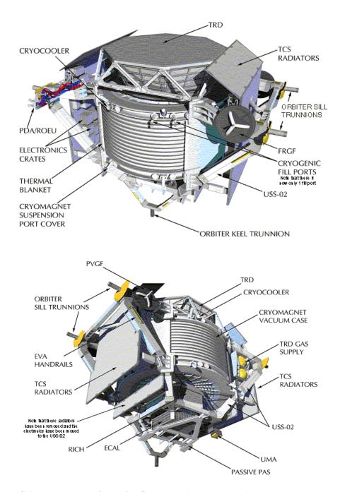
Figure 3.3: Schematic view of the AMS-02 periphery. The subdetectors are mounted inside a unique support structure (USS), which allows the mounting to the Space Shuttle bay by standardized trunnions and to the ISS by an attachment system (PAS) on the bottom. The vacuum case for the cryogenics system is the central part of the structure. The heat dissipated by the electronics systems are radiated into space by four radiator plates.
