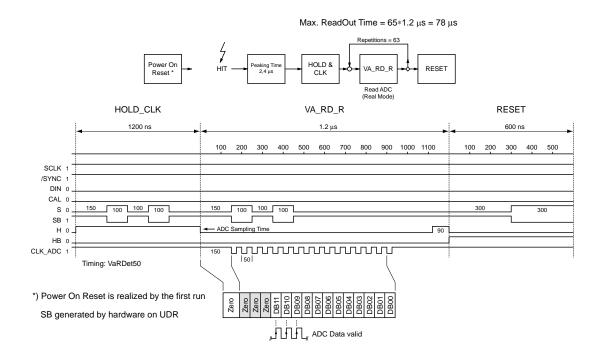
Figure 6.12: Readout Sequence Definition for UFE Boards.
