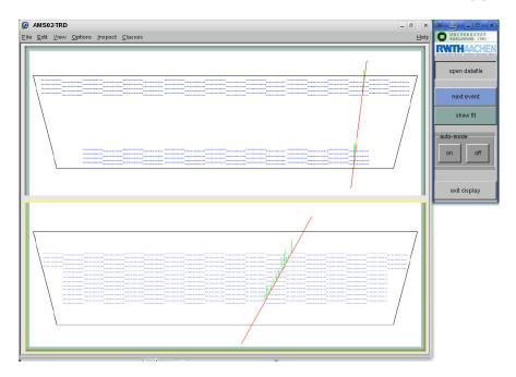
Figure 7.4: The TRD event display in the two dimensional projection. The reconstructed particle track is indicated by a drawn-through line. The Amplitude is visualized by a bar on top of the hit tube.
