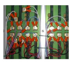
Figure 5.13: An assembled power cable. The wires are mechanically protected by expandable sleeve. On UPD side a connector is attached, which allows easy disconnecting of the cable. On the opposite side gold plated ring lugs are crimped to the cable to be fixed to the U-Crate backplane.
