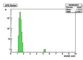
Figure 7.9: The distribution of the TRD channel noise with UHVG half B active. The output has 3-bit precision as in the calculation by the DSP resulting in a decimal precision of 0.125 ADC units. Only two out of 5248 channels show a high noise.
