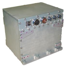
Figure 4.18: Picture of the UPD box. The DC/DC converter boards are completely covered by the aluminum housing. Receptacles attached to the walls allow to connect cables to the U-Crate to the different DC/DC converters inside the box.
