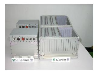
Figure 5.10: U-crates during the assembly. The crates are partially equipped with electronics boards, which are slided into the corresponding slots into VME connectors on the backplane. Before the backplane has been mounted to the backside of the crate's aluminum walls.
