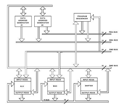
Figure 6.10: Core architecture of the ADSP-2187L. The function of each unit is briefly summarized in this section. [6]
