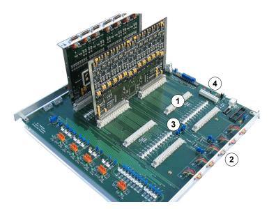
Figure 5.1: UPSFE/UDR2 QM test backplane. The boards are powered via the backplane by VME connectors (1). AMSWire links (2) are present for the communication with the UDR2 board. Shunt resistors (3) are present in all power lines for monitoring of the current. A load resistor allows to apply a variable load by test points on the boards shown in figure 5.2.
