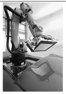
Fig. 1 Compact, robot-based sensor head for recording of light map and optical flow data
